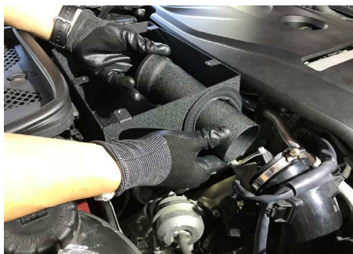
Figure 17: Install the intake tube. 安裝進氣管
