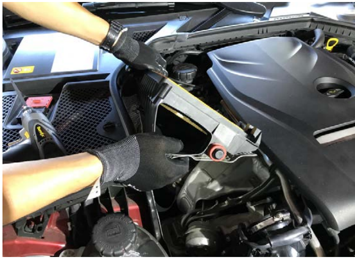
Figure 7: Remove the factory airbox. 拆下原廠氣箱
