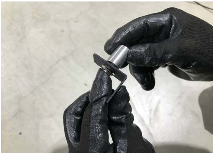
Figure 9: Install the mount on the breaket. 將安裝座安裝到斷路器上
