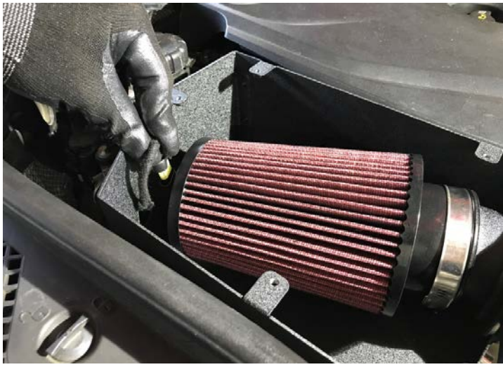
Figure 20: Connect the mass air sensor. Make sure the wire is smooth and has "No twist" 連接空氣品質感測器
