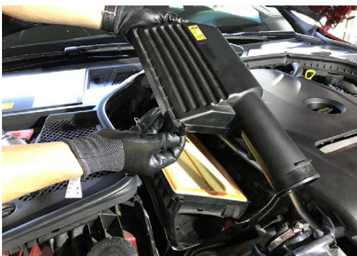
Figure 6: Remove the factory airbox cover. 拆下原廠氣箱蓋
