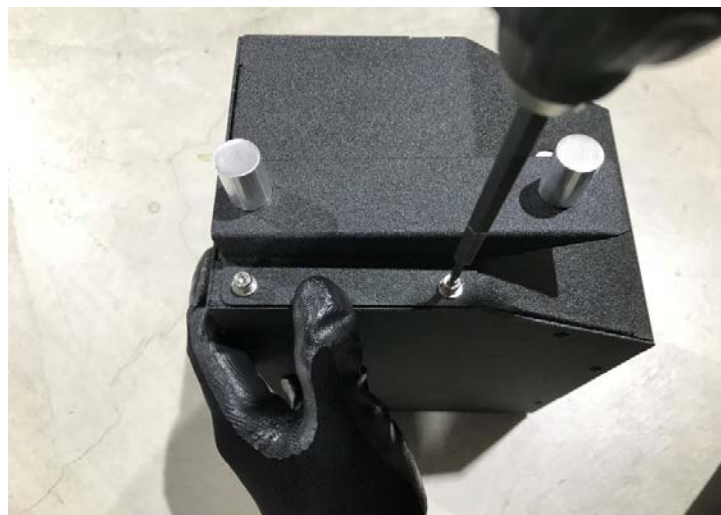
Figure 13: Install the breaket on the heat shield. 將斷路器安裝在隔熱罩上
