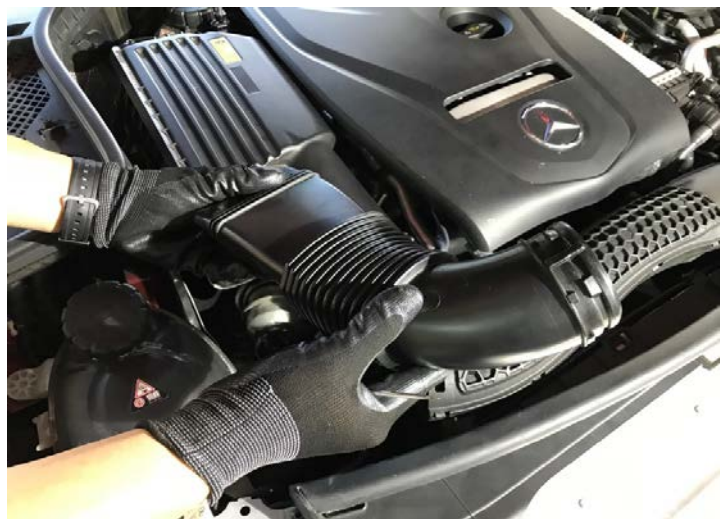
Figure 2: Remove the air ducts. 拆下空氣管道
