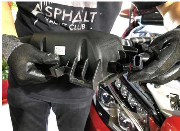
Figure 8: Remove the sensors at the factory airbox carefully. 小心地拆下原廠氣箱中的感應器
