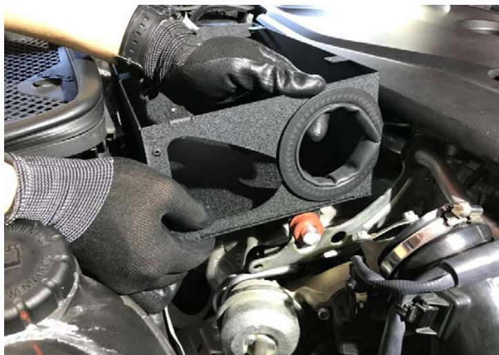
Figure 16: Install the heat shield. 安裝隔熱罩
