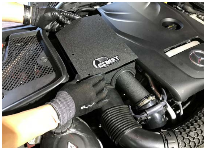
Figure 22: Install the heat shield cover and secure with bolt. 安裝隔熱罩並用螺栓固定 M4 Bolt 8mm x6
