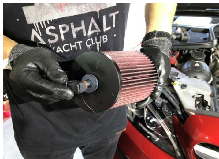
Figure 9: Put into the filter rubber and feel it tight. 放入過濾膠中，感覺是緊的
