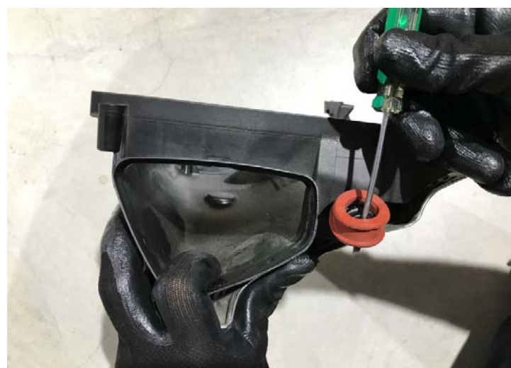
Figure 14: Remove the rubber at the factory airbox. 去除原廠氣箱中的橡膠
