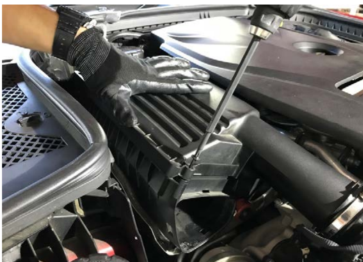
Figure 5: Loosen the bolt at the factory airbox. 鬆開原廠氣箱處的螺栓
