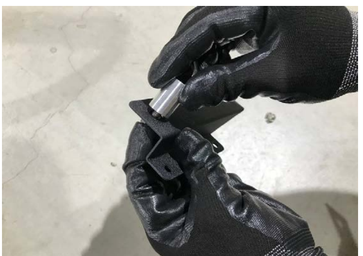
Figure 12: Install the mount on the breaket. 將安裝座安裝到斷路器上
