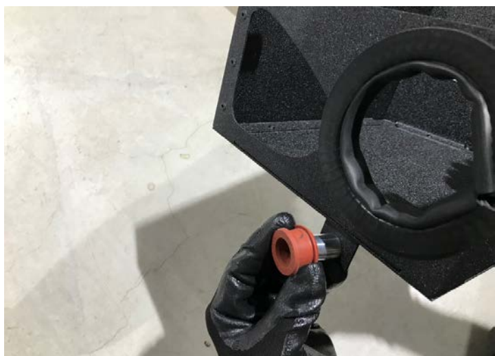
Figure 15: Install the rubber on the heat shield breaket. 將橡膠安裝到隔熱罩支架上
