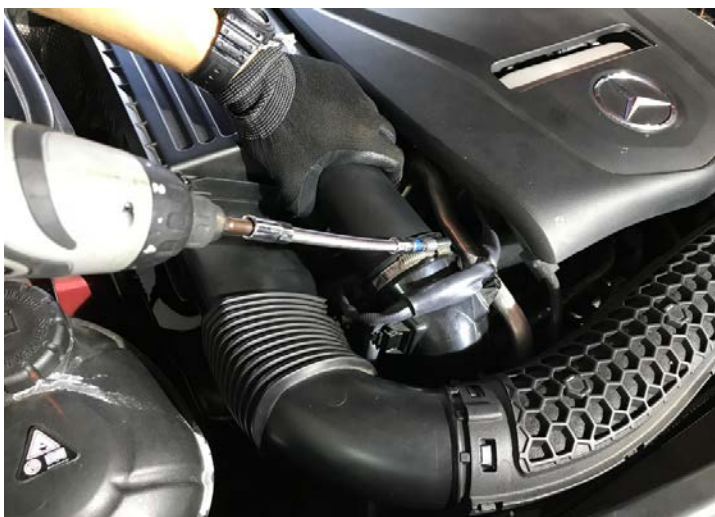
Figure 3: Loosen hose clamp at the factory tube. 鬆開原廠管上的軟管夾
