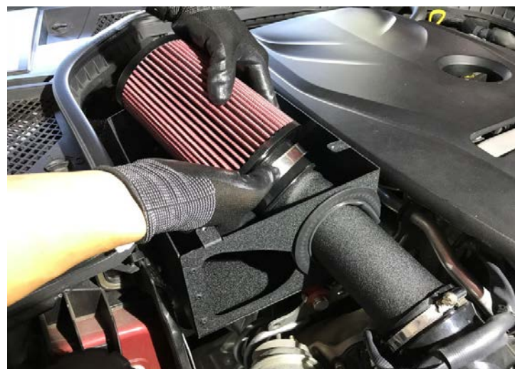
Figure 19: Install the air filter. 安裝空氣濾芯
