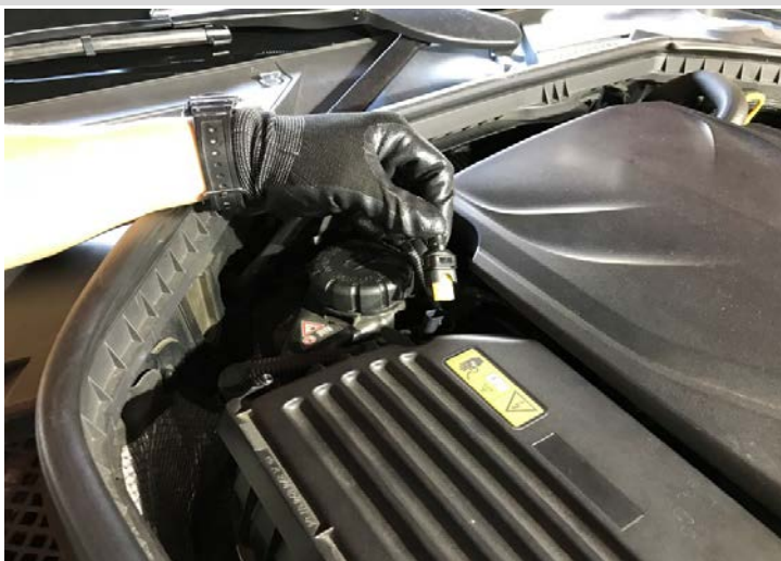
Figure 4: Unclip the sensor. 鬆開感應器
