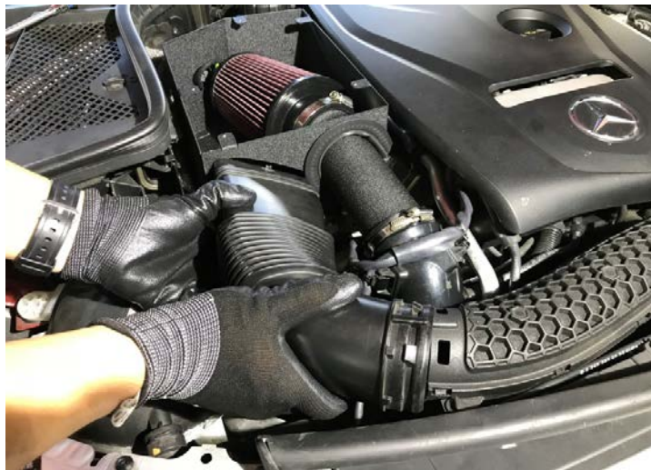
Figure 20: Connect the mass air sensor. Make sure the wire is smooth and has "No twist" 連接空氣品質感測器
