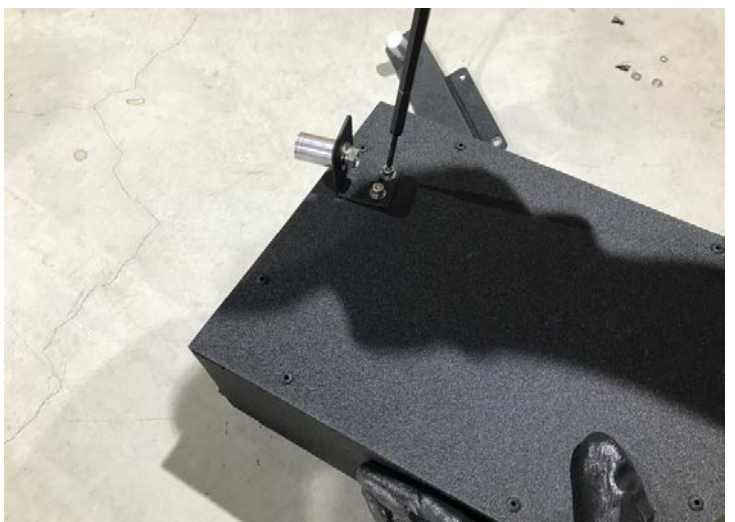
Figure 11: Install the breaket on the heat shield. 將斷路器安裝在隔熱罩上
