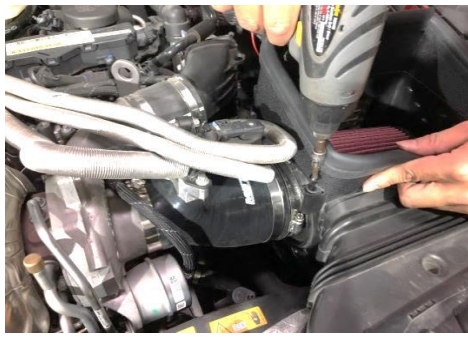
Figure 31: Install and tighten the screws for the heat shield
