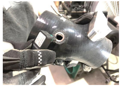
Figure 18: Install the temperature sensor on the MST silicone inlet hose
