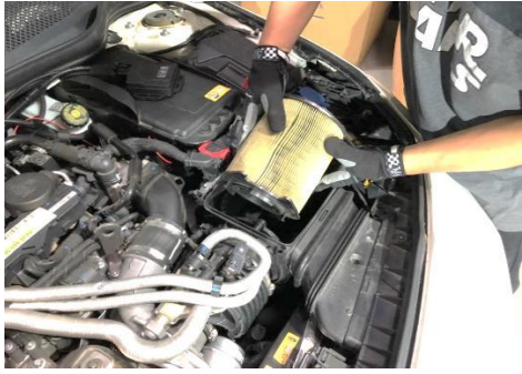
Figure 4: Remove the stock air filter by turning it counterclockwise.
