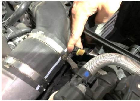
Figure 8: Separate the temperature sensor
