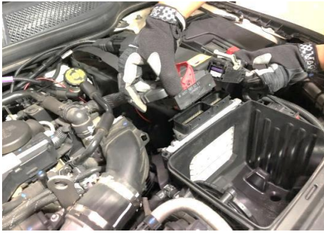
Figure 5: Disconnect the ECU connector
