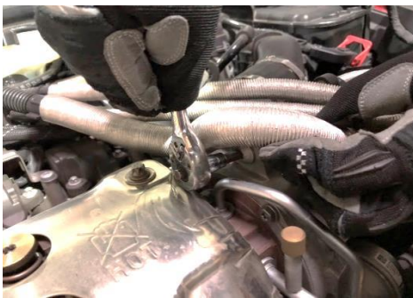
Figure 11: Unscrew the sensor bracket bolts
