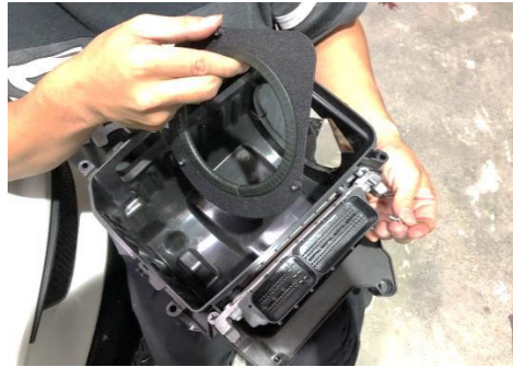
Figure 19: Place the MST "B" heatshield inside of air box
