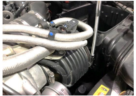
Figure 9: Loosen the clamps on the stock hose
