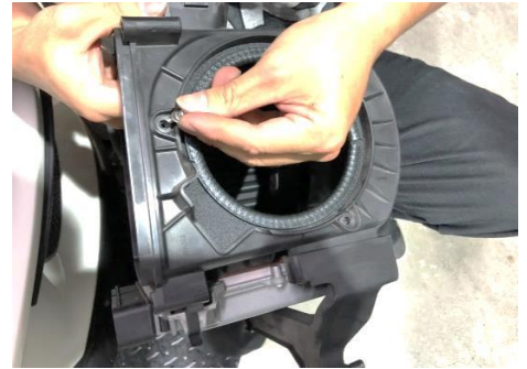
Figure 21: Lock the screws for the MST heat shield on the stock air box.
