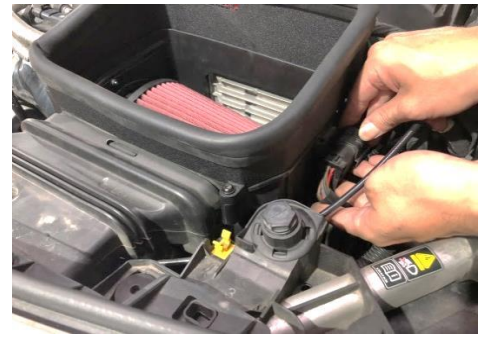
Figure 33: Reconnect the connector on the side of air box
