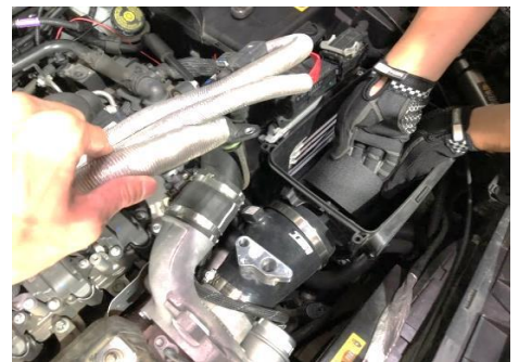
Figure 24: Install the 100mm MST intake pipe
