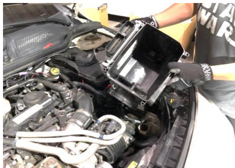
Figure 10: Remove the stock air box
