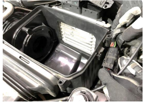
Figure 6: Disconnect the wire harness connector on the side of air box.
