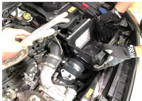
Figure 23: Install the stock air box.
