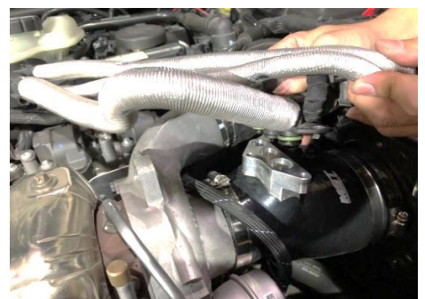
Figure 27: Reconnect the sensor into the hose. [Metal Bracket is not re-used]
