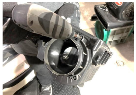
Figure 15: Unscrew the screws on the stock air box
