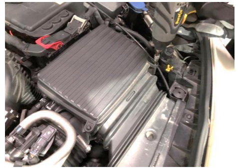
Figure 3: Loosen the screws on the air box
