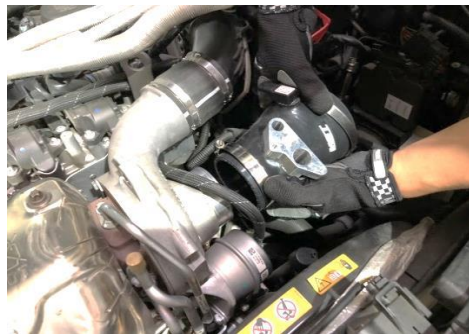
Figure 22: Install the MST silicone inlet
