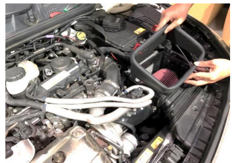
Figure 30: Install the MST heat shield "A" on the air box
