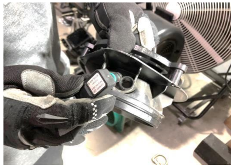
Figure 17: Remove the temperature sensor on the adapter
