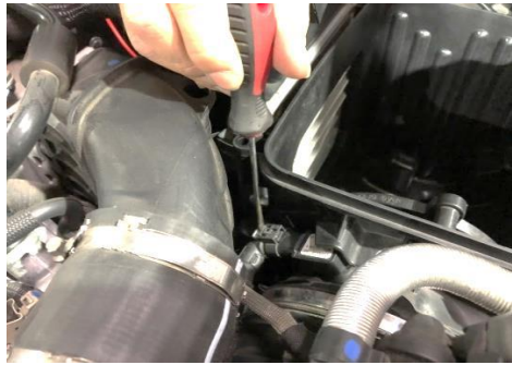
Figure 7: Disconnect the temperature sensor.
