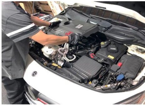
Figure 2: Remove the engine cover.
