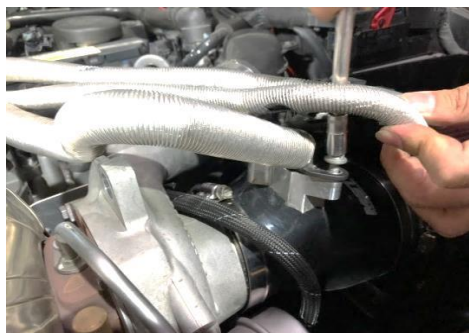
Figure 28: Lock the screws on the hose
