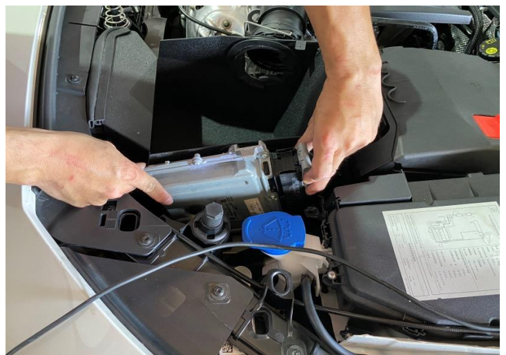
Figure 18: Install the ECU on the heat shield.
