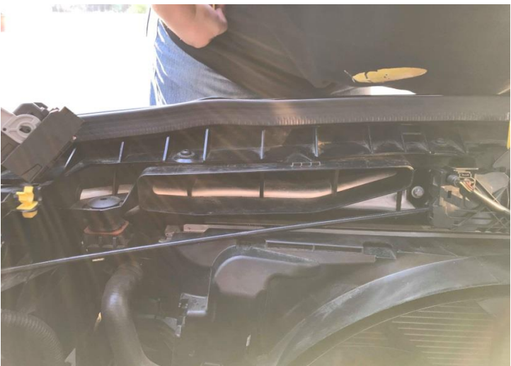
Figure 11: Release the inlet cover by squeezing and pushing the cover retainer tabs located on either side of the secondary inlet.
