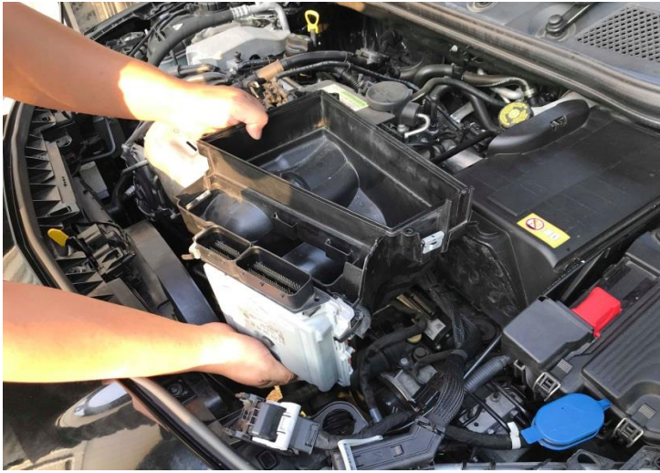
Figure 7: Remove the stock air box.
