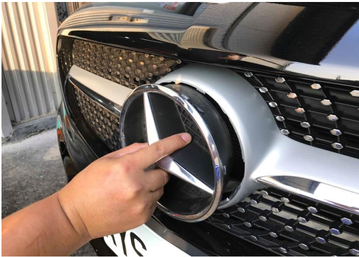
Figure 9: To open up maximum airflow to intake, the secondary air inlet must be uncovered. Twist the Mercedes emblem on the grill counterclockwise and pull to remove it. If your car is equipped with Distronic radar-assisted parking and cruise control features, this emblem will not be removable by twisting in this fashion. The grill will need to be removed to allow removal of the cover as detailed in step 3h below.
