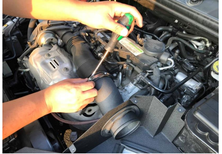
Figure 22: Tighten the hose clamp.
