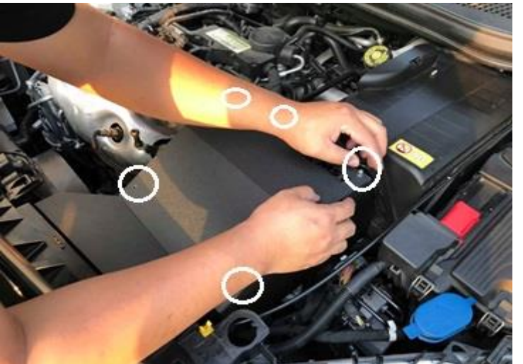
Figure 24: Install the heat shield cover and secure with bolt. M4 Blot 8mm x5
