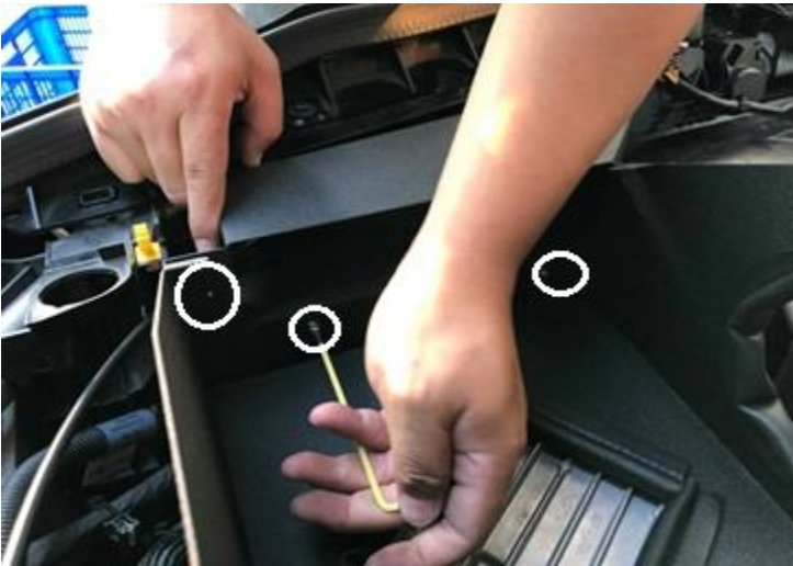
Figure 20: Secure with bolt. M4 Blot 8mm x3
