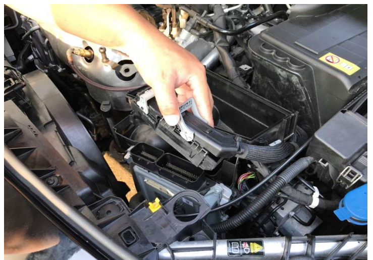
Figure 6: Disconnect the ECU. (the ECU will install below the Heat Shielded)
