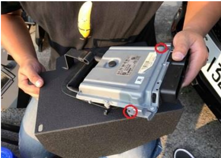
Figure 8: Fasten the ECU to the bottom of the heat shield. M4 Bolt 12mm x 2
