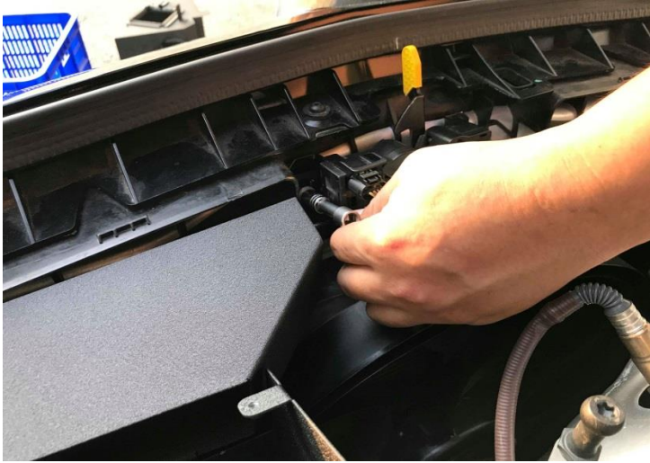
Figure 19: Secure with bolt.
