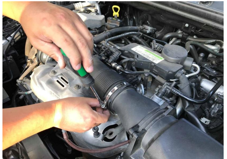
Figure 4: Loosen hose clamp at the factory airbox connection and remove as shown.
