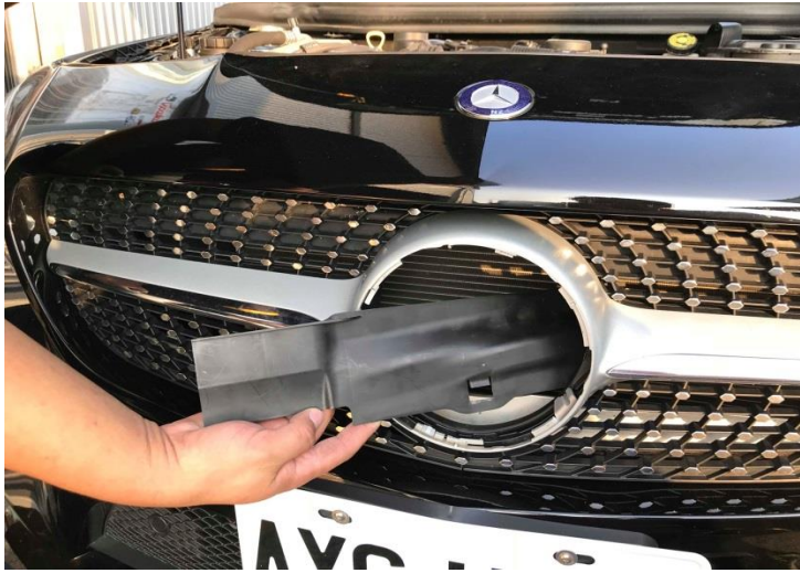
Figure 13: The inlet cover may now be removed through the emblem hole.
