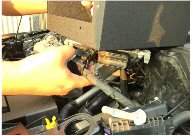
Figure 16: Plug in the ECU. Please note: unbuckle wires along the airbox, pull and arrange wires, make the ECU install under the Heat Shield.
