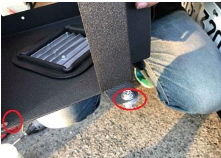
Figure 15: Install mount on the heat shield. M6 Bolt x2
