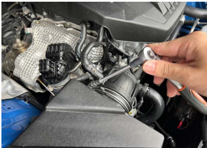
Figure 2: Loosen the stock tube hose clamp. 鬆開軟管夾
