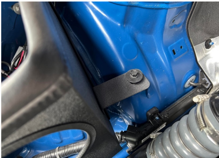
Figure 8: Secure with bolt. 用螺栓固定
