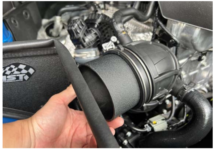
Figure 10: Install the 100mm MST intake pipe. 安裝100mm MST進氣管
