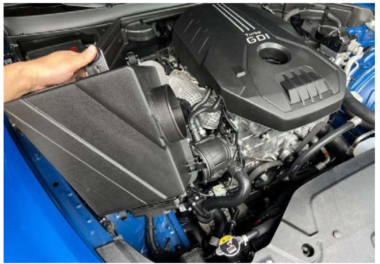
Figure 4: Remove the stock air box. 拆下原廠集氣箱
