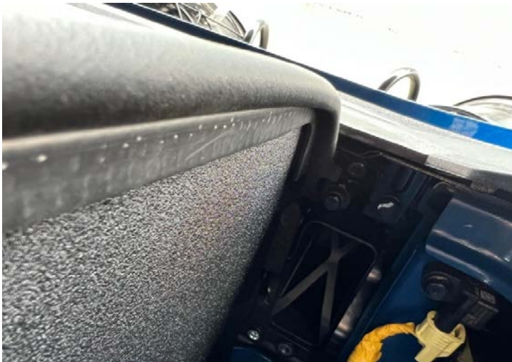
Figure 9: Secure the heat shield bracket with bolt. 用螺栓固定隔熱罩支架
