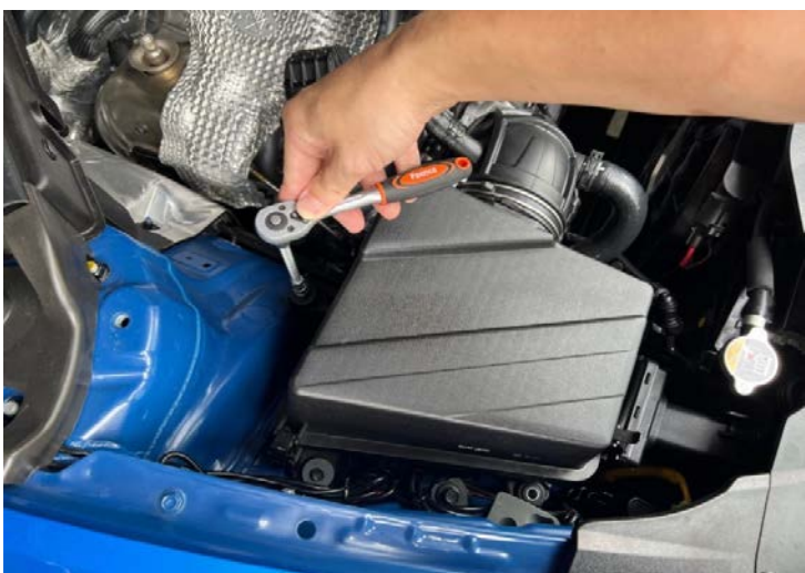
Figure 3: Remove the air box muffler screw. 拆下集氣箱消音器螺絲
