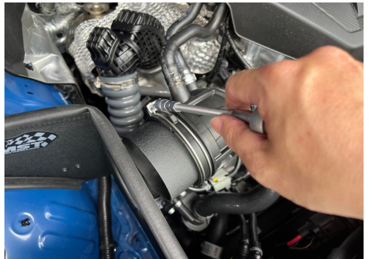
Figure 11: Tighten the hose clamp. 擰緊軟管夾
