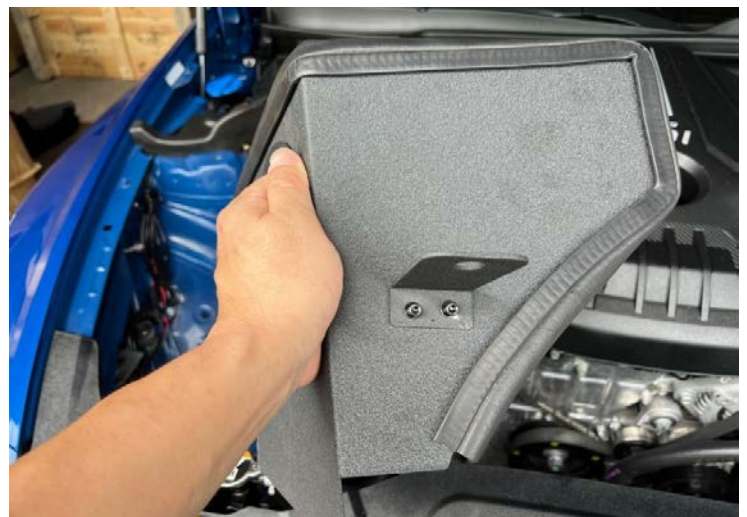
Figure 6: Install the heatshield bracket 安裝隔熱罩支架
