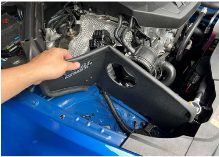
Figure 7: Install the heat shield. 安裝隔熱罩
