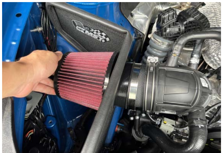
Figure 12: Install the MST air filter. 安裝 MST 空氣濾芯
