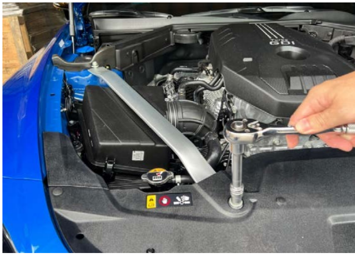
Figure 1: Remove the stock strut bar. 拆下支柱桿
