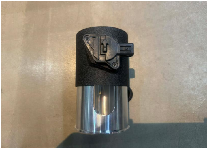
Figure 8: A sleeve is install inside the MST tube and install the MAF sensor. Note the installation orientation of the sleeve, incorrect orientation will cause errors in CEL.
