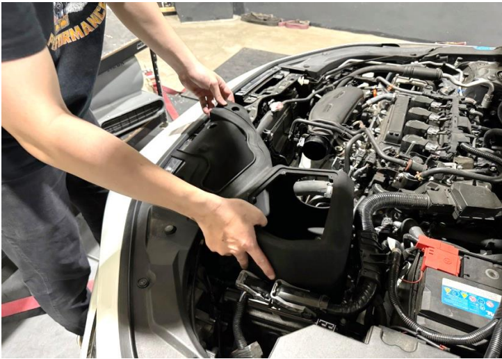
Figure 9: Install the MST air box.
