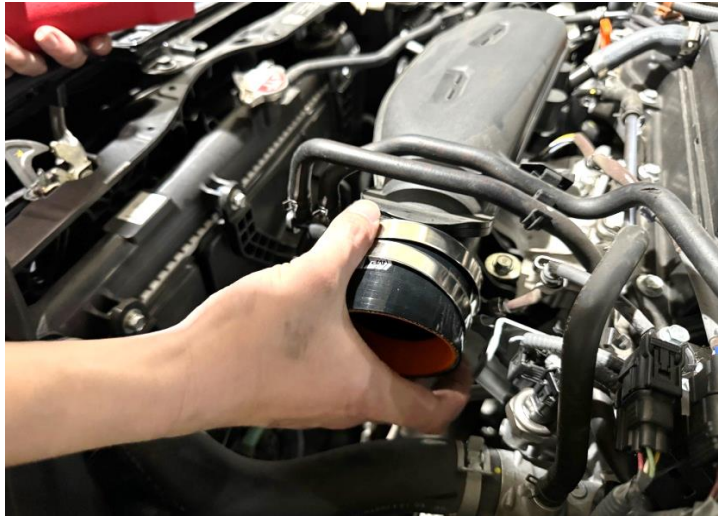
Figure 11: Install the silicone hose.
