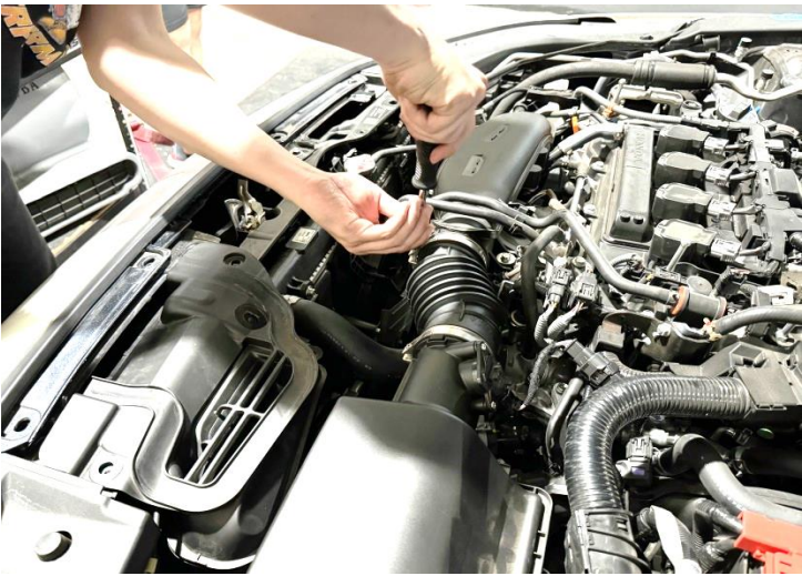
Figure 2: Loosen the stock inlet hose clamp.
