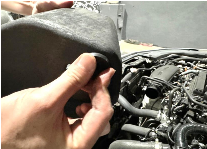
Figure 8: Install the rubber on the air box.
