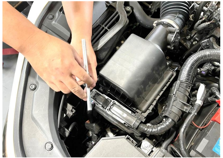
Figure 5: Remove the air box bolts.
