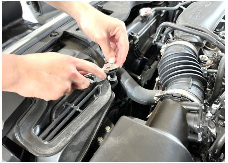
Figure 4: . Remove the air scoop bolts.
