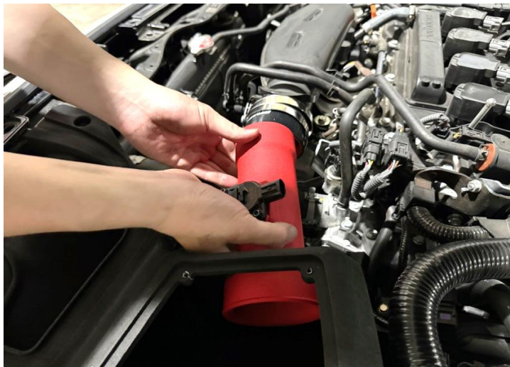
Figure 12: Remove the stock air tube.
