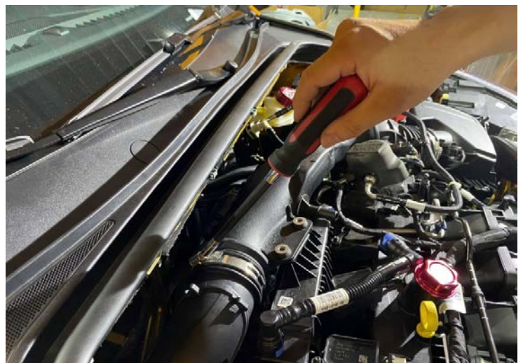
Step 6. Use 7mm socket to loosen the stock induction pipe hoseclamp as shown 步驟 6: 使用7號六角工具鬆開原廠進氣管管束
