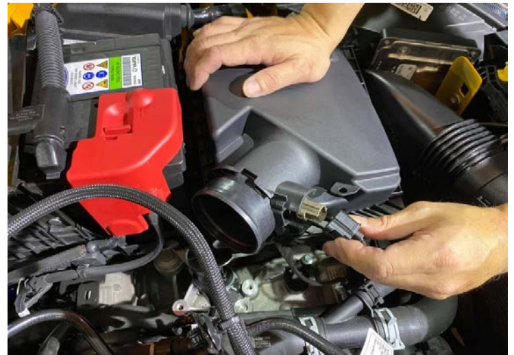
Step 10. unplug the air temperature sensor plug on the air box as shown 步驟 10: 斷開集氣箱上方溫度感應器插頭
