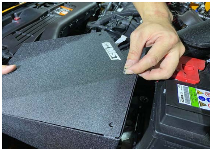
Step 28. fit the MST Heat Shield Cover onto the bottom half of the air box and secure with fasteners, all the related hose clamps can now be tightened, make sure to tighten and check all of the related hose connections, hose clamps and spring clips 步驟 28: 蓋上MST集氣箱上蓋鎖緊螺絲
