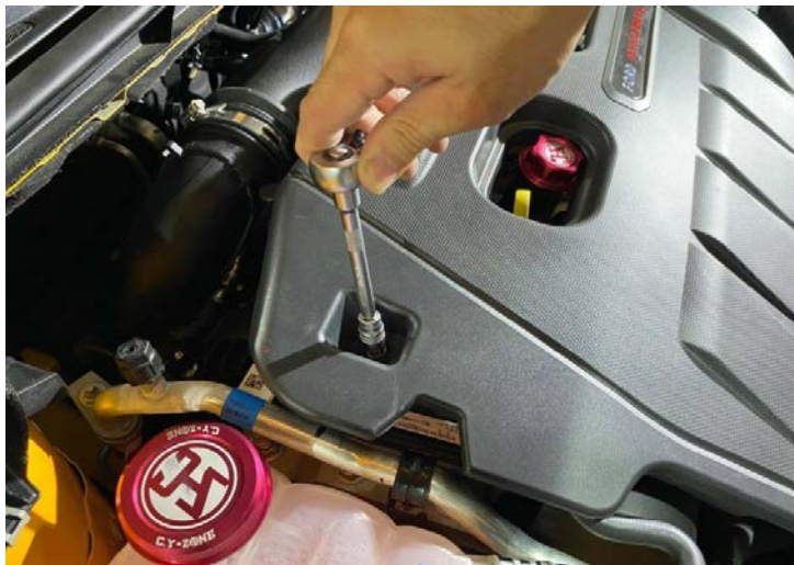
Step 2. Use 10mm socket to remove plastic engine trim cover retainer as shown 步驟 2: 使用10號六角取下螺絲
