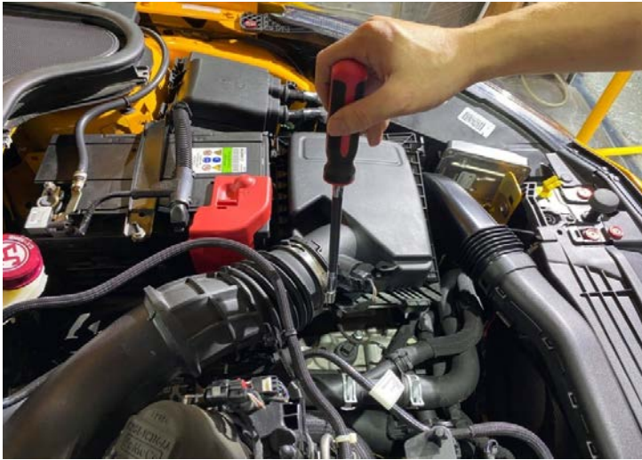
Step 7. Use 7mm socket to loosen the stock induction pipe hose clamp (air box side) as shown 步驟 7: 使用7號六角工具鬆開原廠進氣管管束
