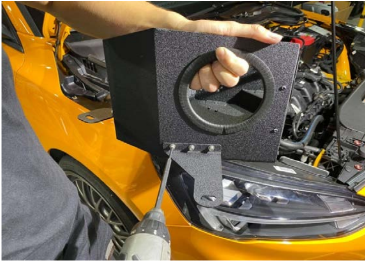
Step 13. Install the MST heat shield mounting bracket with M4 bolts onto the heat shield as shown 步驟 13: 安裝MST隔熱罩吊板,使用M4螺絲固定
