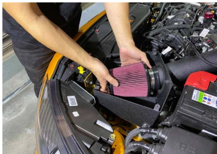
Step 27. Slide the 89mm hose clamp over the MST air filter and fit the air filter onto the induction pipe as shown, tighten the air filter hose clamp 步驟 27: 安裝MST高流量濾心
