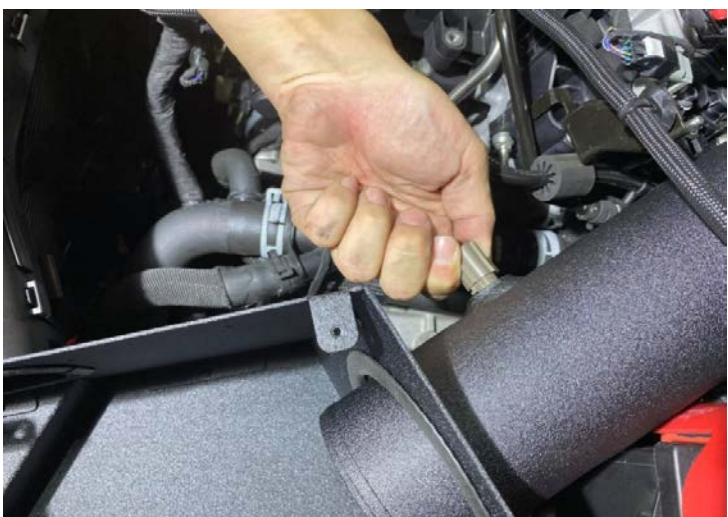
Step 26. Refit the factory air temperature sensor removed back in Step 12 onto the MST induction pipe as shown 步驟 26: 安裝溫度感應器至MST進氣管上
