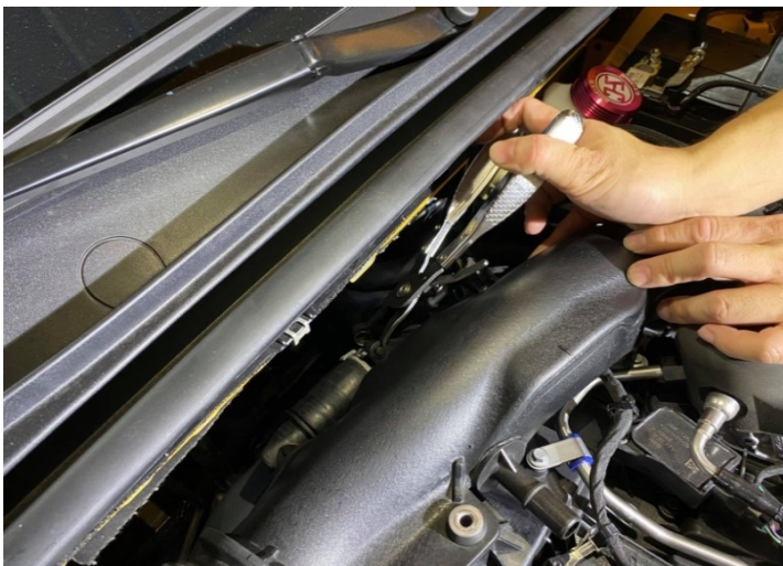
Step 8. Use spring clamp pliers to release spring clamp and pull off the rubber pipe behind the stock induction pipe 步驟8用夾子將原廠進氣管後方橡膠管鬆開
