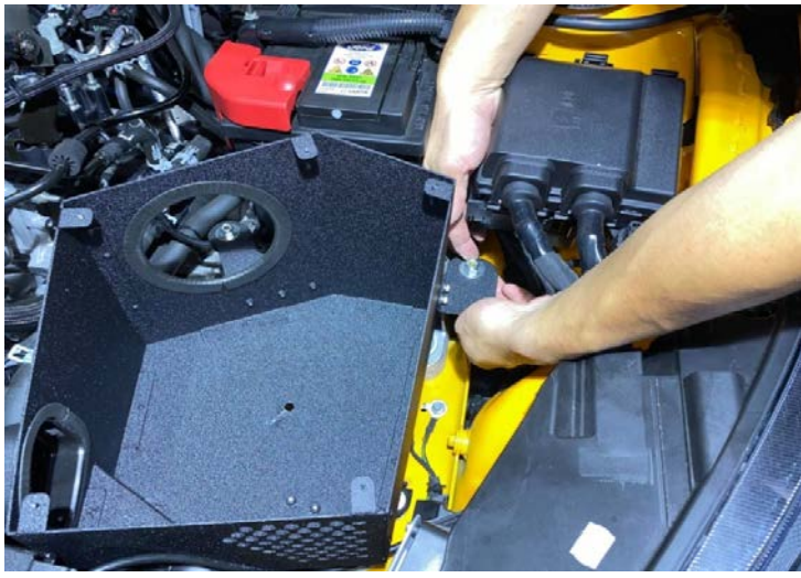
Step 19. secure the mounting bracket with M8 fasteners as shown 步驟 19: 使用M8螺絲固定隔熱罩
