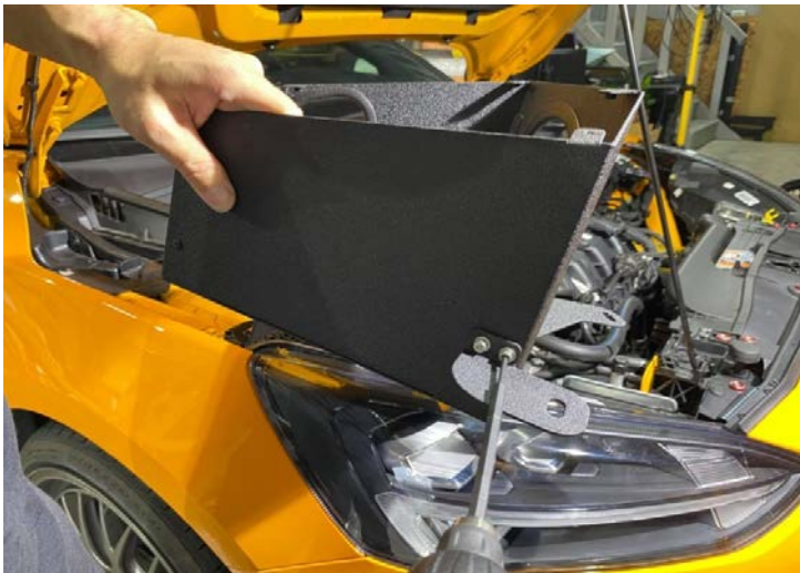
Step 14. Install the MST heat shield mounting bracket with M4 bolts onto the heat shield as shown 步驟 14: 安裝MST隔熱罩吊板,使用M4螺絲固定
