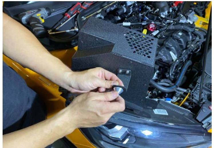
Step 16. Use M6 fasteners to mount the aluminium cone shape anchor head to the mounting bracket 步驟 16: 將錐形鋁座安裝至吊板上,使用M6螺絲固定
