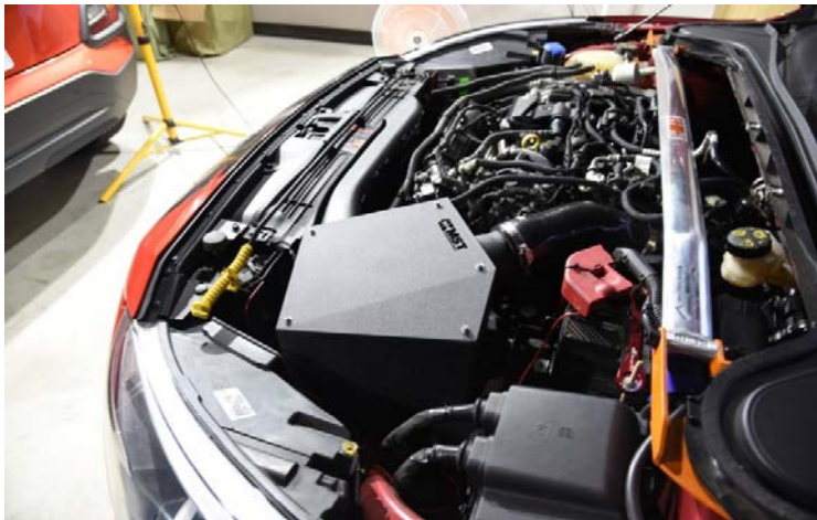
Figure 14: Congratulations! You have just completed the installation of this intake system. Periodically, check the alignment of the intake, normal wear and tear can cause nuts and bolts to come loose.
