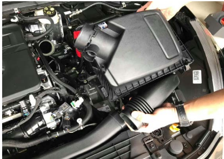
Figure 4: Loosen stock air box cover spring. 鬆開原裝空氣箱蓋彈簧
