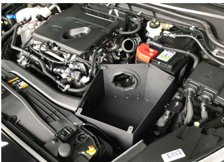
Figure 8: Install the heat shield.
