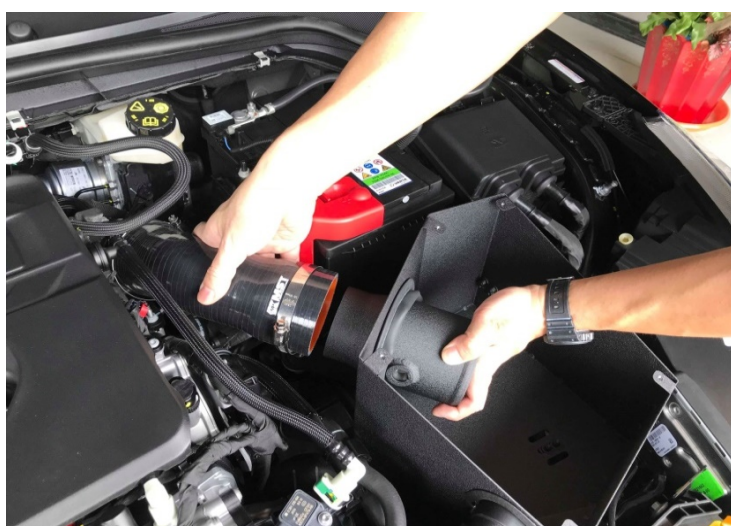
Figure 11: Install the air pipe.
