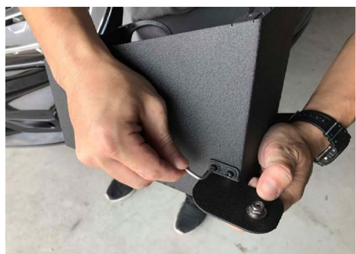
Figure 6: Install the bracket on the heat shield. 將支架安裝在隔熱罩上
