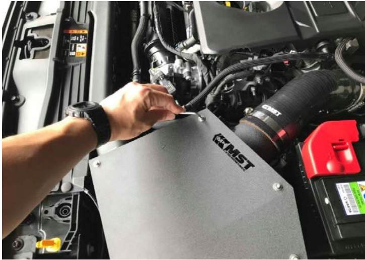
Figure 13: Install the heat shield cover and secure with bolt. 安裝隔熱罩蓋並用螺栓固定
