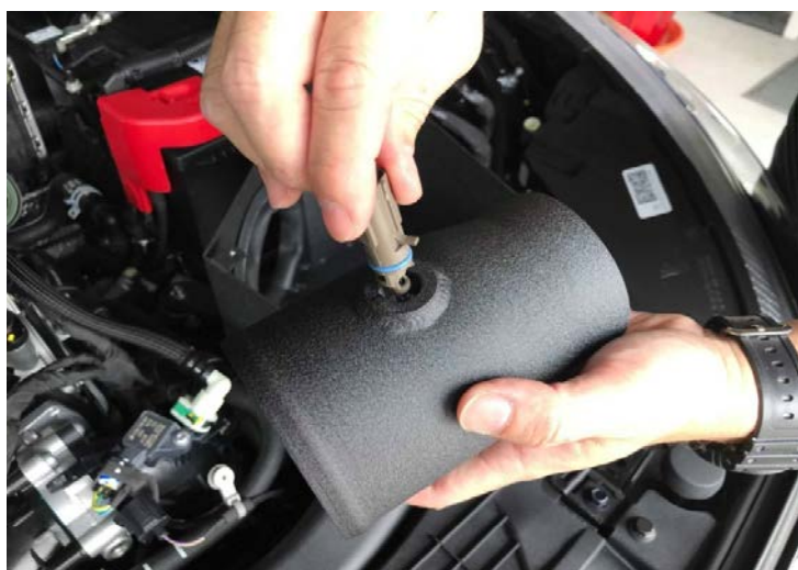
Figure 9: Install the air tempure sensor.
