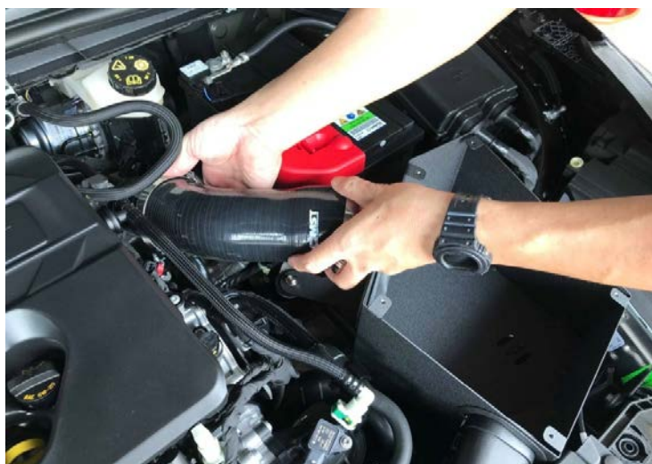
Figure 10: Install the silicone hose.
