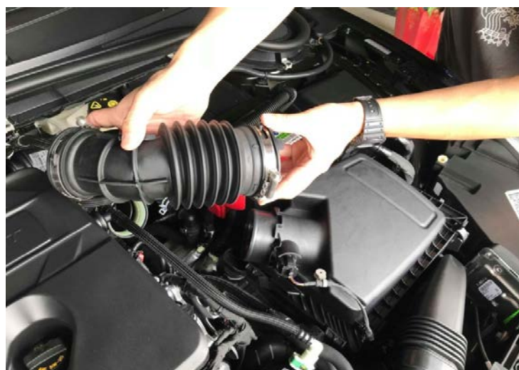
Figure 2: Remove the stock hose. 拆下原廠軟管
