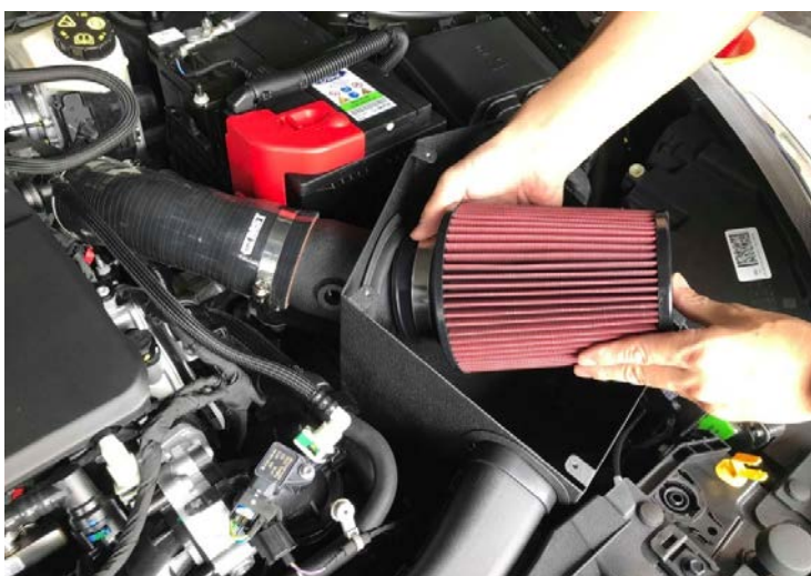
Figure 12: Install air filter.
