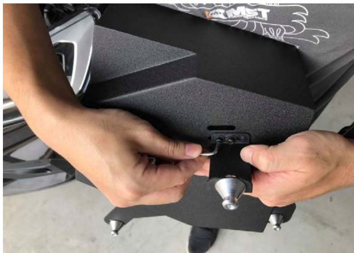
Figure 7: Install the bracket and mount on the heat shield.
