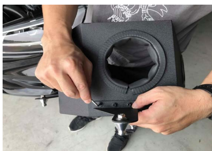
Figure 5: Install the bracket on the heat shield. 將支架安裝在隔熱罩上
