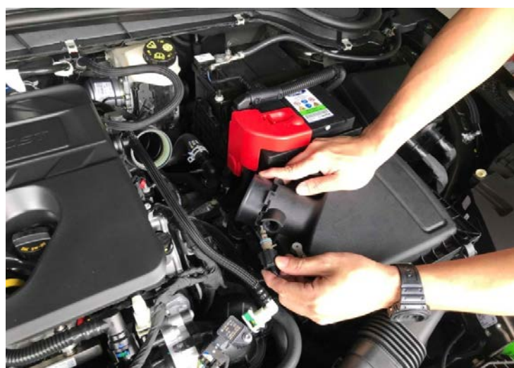
Figure 3: Disconnect the air temperature sensor. 斷開空氣溫度傳感器
