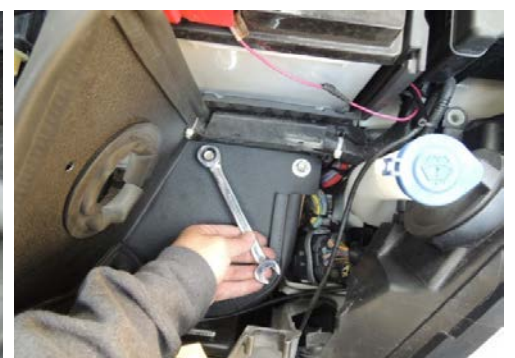
Figure 12: Secure thw washer and m8 locknut. Tighten the 2 bolts using 13mm socket and wrench. 固定墊圈和 m8 鎖緊螺母。使用 13mm 套筒和扳手擰緊 2 個螺栓
