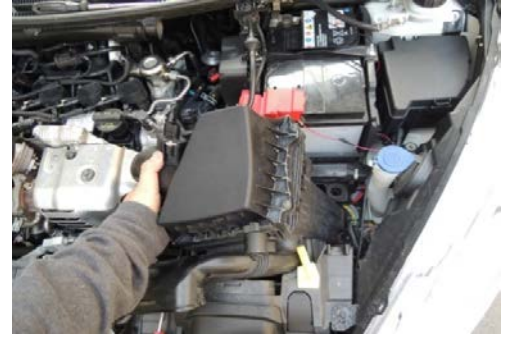
Figure 6: Now lift up and remove the stock air box out of vehicle. 現在抬起並從車輛中取出備用空氣箱
