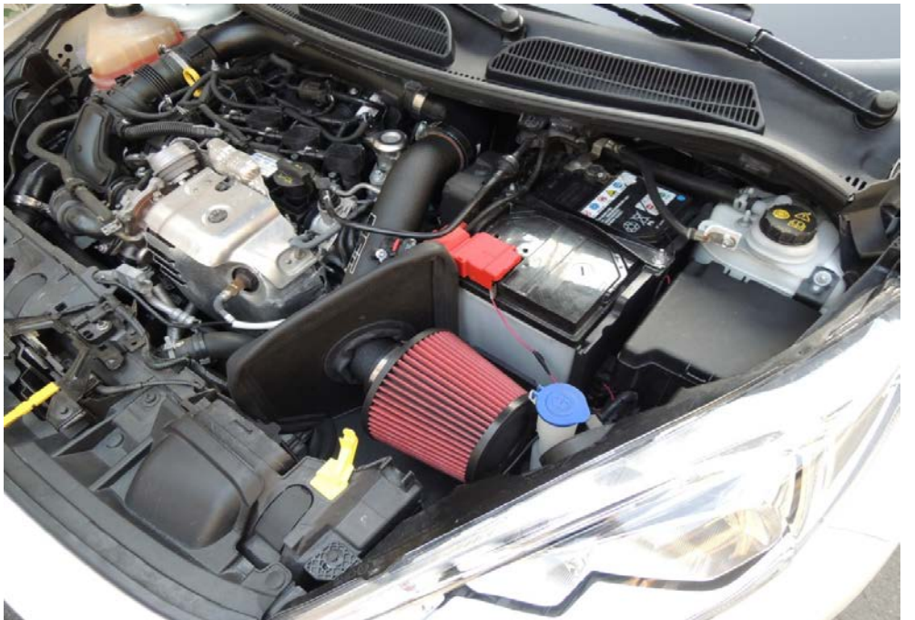
Figure 17: Congratulations! You have just completed the installation of this intake system. Periodically, check the alignment of the intake, normal wear and tear can cause nuts and bolts to come loose. 恭喜！您剛剛完成了該進氣系統的安裝。定期檢查進氣口的對齊情況，正常磨損會導致螺母和螺栓鬆動
