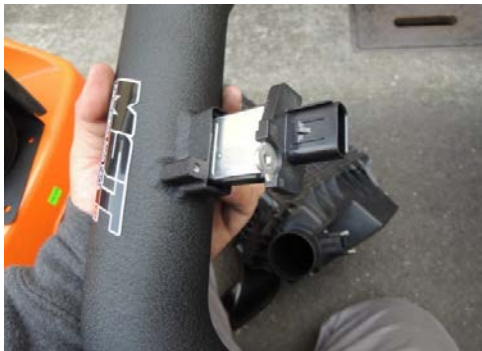
Figure 8: Now install the MAF sensor into the new intake tube. 現在將 MAF 感應器安裝到新的進氣管中
