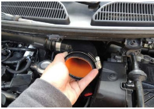
Figure 13: Now install the straight hose with clamps on the tube. Tighten the clamp on the tube side only. 現在將帶夾子的直管安裝到管子上。僅擰緊管側的夾具
