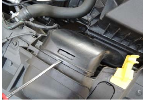
Figure 5: Pull back the ram air scoop from radiator support. 拔掉導風罩
