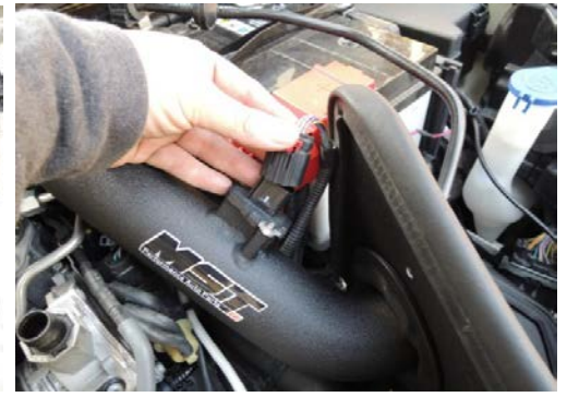
Figure 15: Connect the MAF sensor harness. 連接 MAF 感應器線
