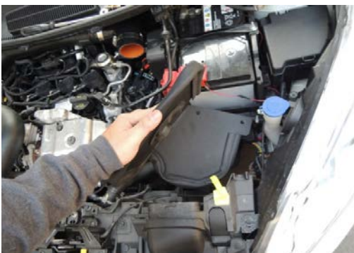
Figure 10: Install the heatshield and position into vehicle. Locate the 2 holes on heatshield to the grommets. 安裝隔熱罩並放入車內。將隔熱罩上的 2 個孔定位到索環
