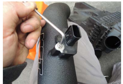
Figure 9: Secure and tighten using provided M4 screws. 使用提供的 M4 螺絲固定並擰緊
