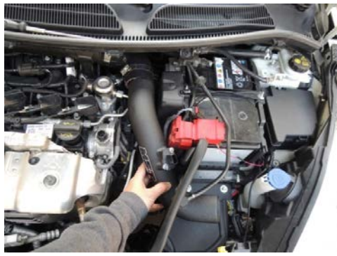
Figure 14: Now install the intake tube to the hose on tube. 現在將進氣管安裝到管上的軟管上
