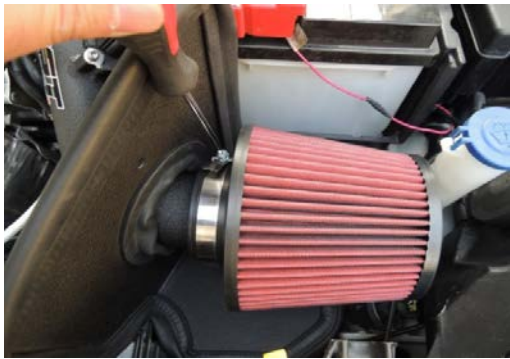
Figure 16: Install the filter to the intake tube and tighten. 將過濾器安裝到進氣管上並擰緊
