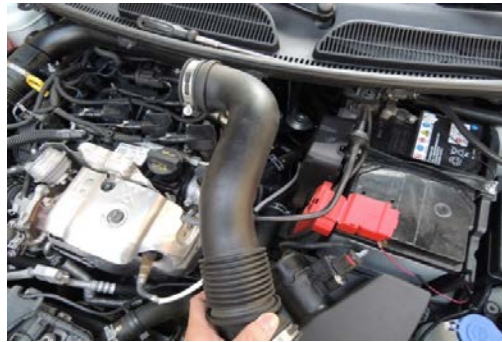
Figure 4: Remove the intake tube from vehicle.從車輛上拆下進氣管
