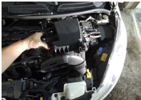
Figure 5: Now lift up and remove the stock air box out of vehicle. 現在抬起並從車輛中取出備用空氣箱
