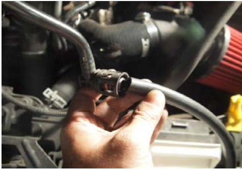
Figure 16: When equipped with vent hose, install the vent hose to the npt vent fitting. 配備排氣軟管時，將排氣軟管安裝到 npt 排氣接頭上
