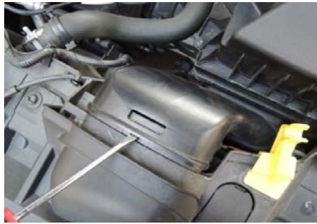
Figure 4: Pull back the ram air scoop from radiator support. 拔掉導風罩
