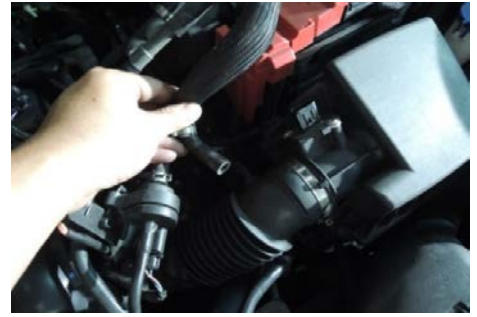
Figure 3: When equipped with EVAP, disconnect the EVAP vent line from the factory intake tube as shown. 配備 EVAP 時，如圖所示斷開 EVAP 排氣管與原廠進氣管的連接
