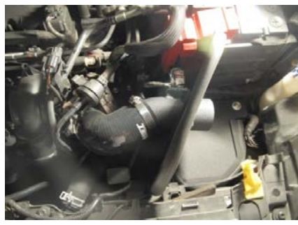
Figure 14: Now install the intake tube to the hose on tube. 現在將進氣管安裝到管上的軟管上
