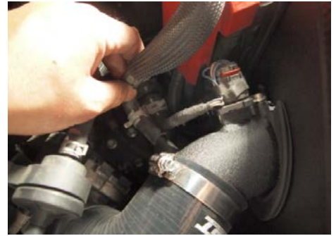
Figure 18: Install the EVAP vent hose to the npt vent fitting. 將 EVAP 排氣軟管安裝到 npt 排氣接頭上
