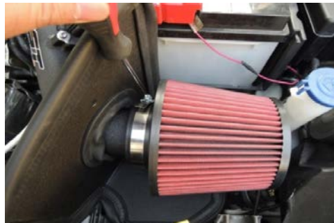
Figure 19: Install the filter to the intake tube and tighten. 將過濾器安裝到進氣管上並擰緊
