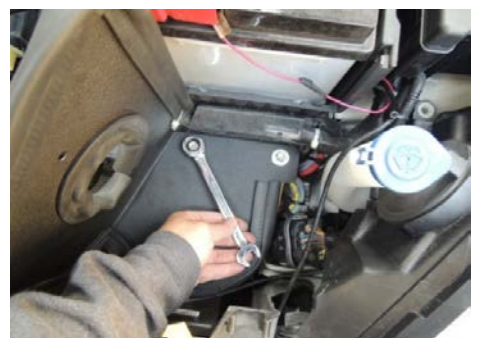
Figure 12: Secure the washer and m8 locknut. Tighten the 2 bolts using 13mm socket and wrench. 固定墊圈和 m8 鎖緊螺母。使用 13mm 套筒和扳手擰緊 2 個螺栓
