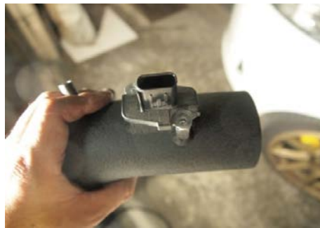
Figure 8: Now install the MAF sensor into the new intake tube. 現在將 MAF 感應器安裝到新的進氣管中
