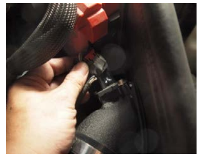
Figure 15: Connect the MAF sensor harness. 連接 MAF 感應器線束
