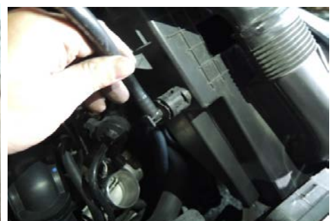
Figure 6: disconnect the vent hose from air box. 斷開通風軟管與空氣箱的連接
