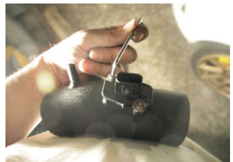
Figure 9: Secure and tighten using provided M4 screws. 使用提供的 M4 螺絲固定並擰緊
