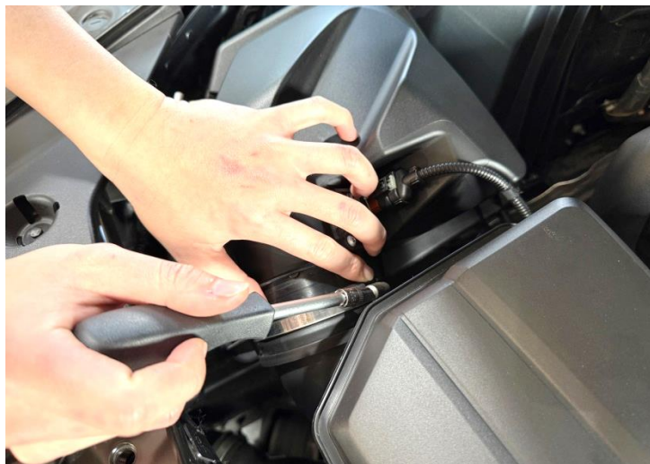
Figure 3: Loosen the hose clamp.
