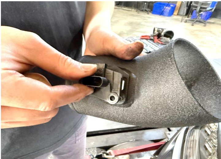
Figure 8: Install the MAF sensor on MST tube.
