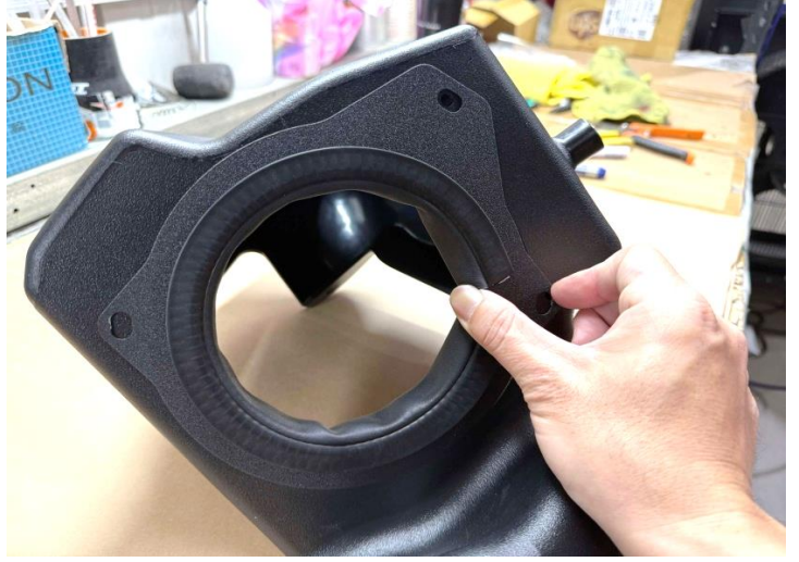
Figure 10: Install the air box cover.
