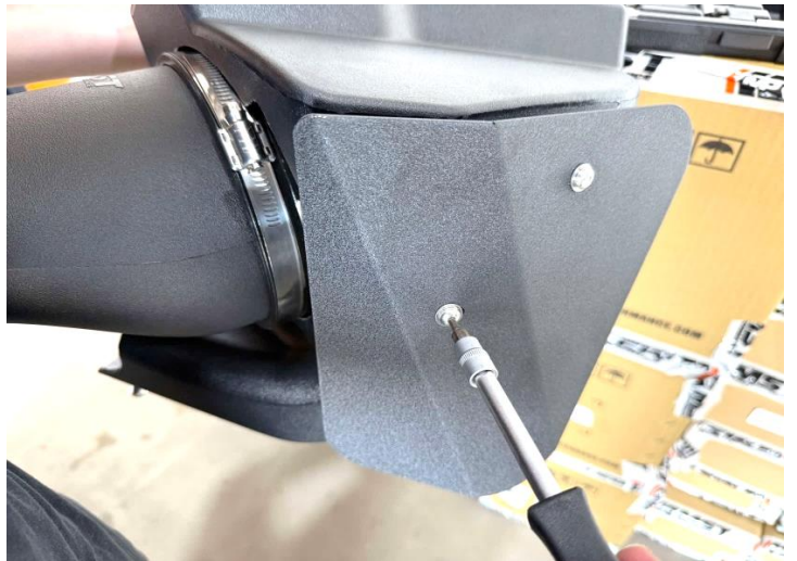
Figure 11: Install the heat shield on the air box.
