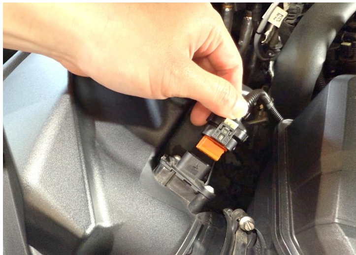
Figure 2: Disconnect the mass air sensor.
