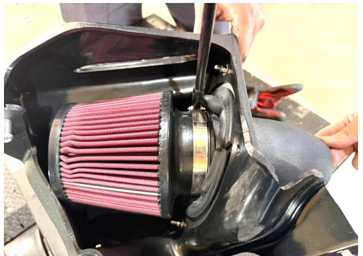
Figure 12: Install the filter,tube and aluminum mont on the air box.
