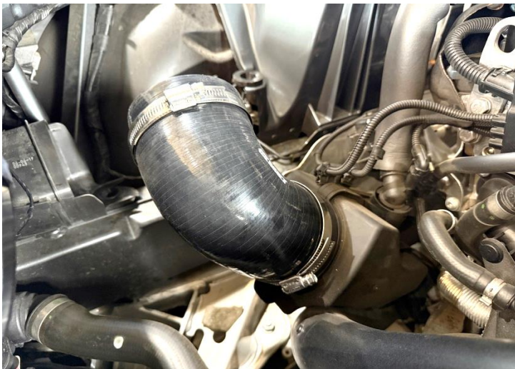
Figure 9: Install the silicone hose.
