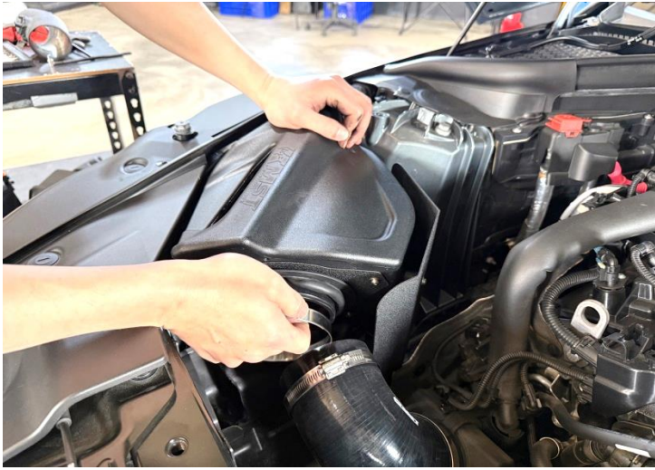
Figure 13: Install the air box.
