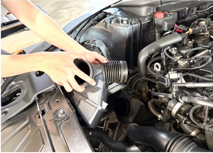
Figure 7: Remove the stock tube.
