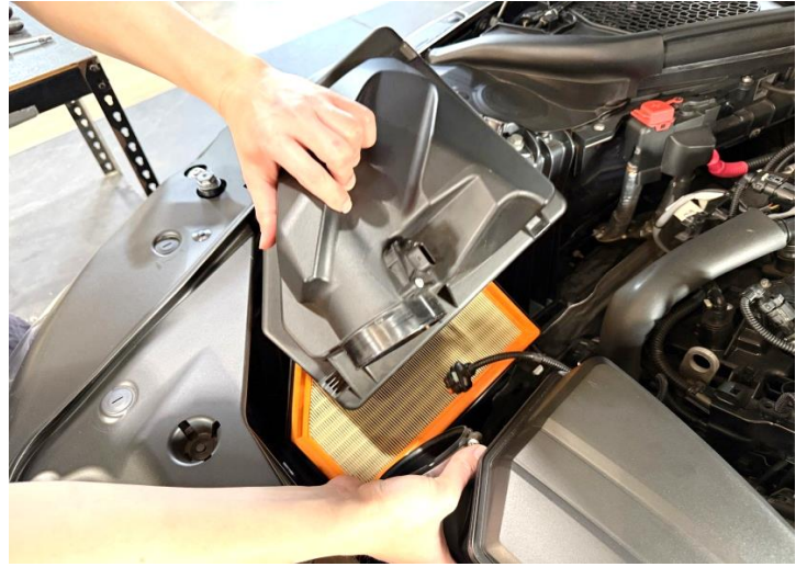
Figure 4: Remove stock air box cover.
