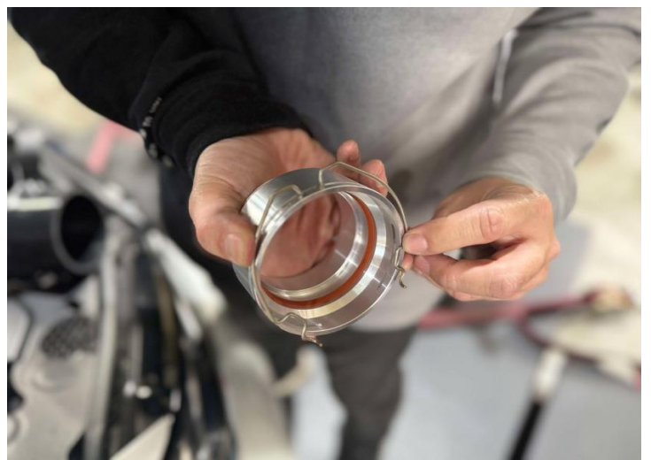
Figure 12: Install the spring clip clamp.
