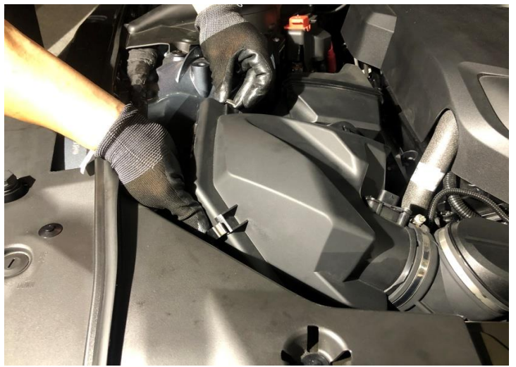
Figure 4: Loosen stock air box cover spring.
