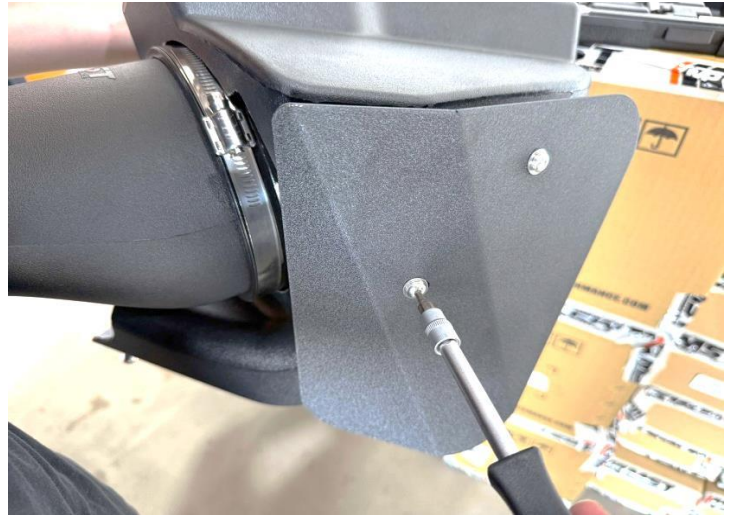
Figure 16: Install the heat shield on the air box.
