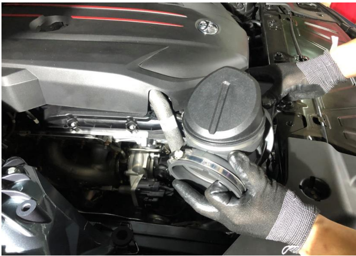
Figure 8: Remove the stock turbo inlet pipe.
