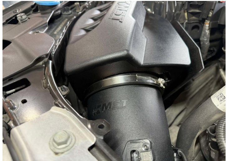
*This clip is installed on the outside of the air box for 3.0 BMW G-Chassis
