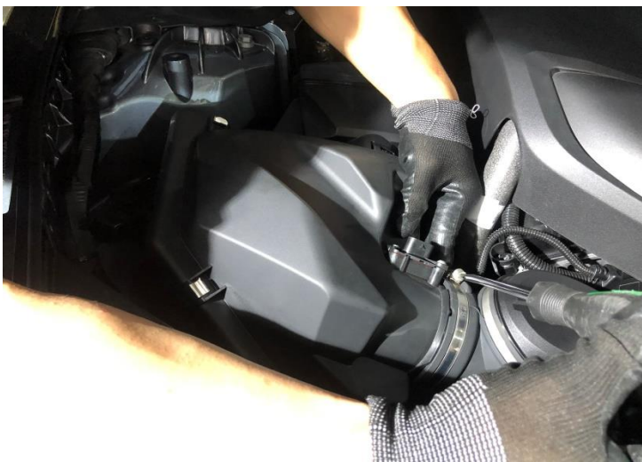
Figure 3: Loosen the hose clamp.
