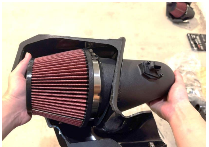
Figure 18: Install the filter, tube and aluminum mount on the air box.
