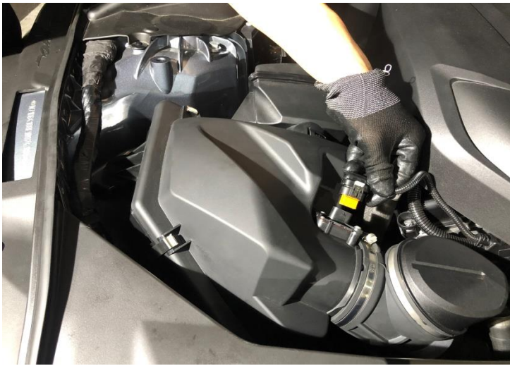
Figure 2: Disconnect the mass air sensor.
