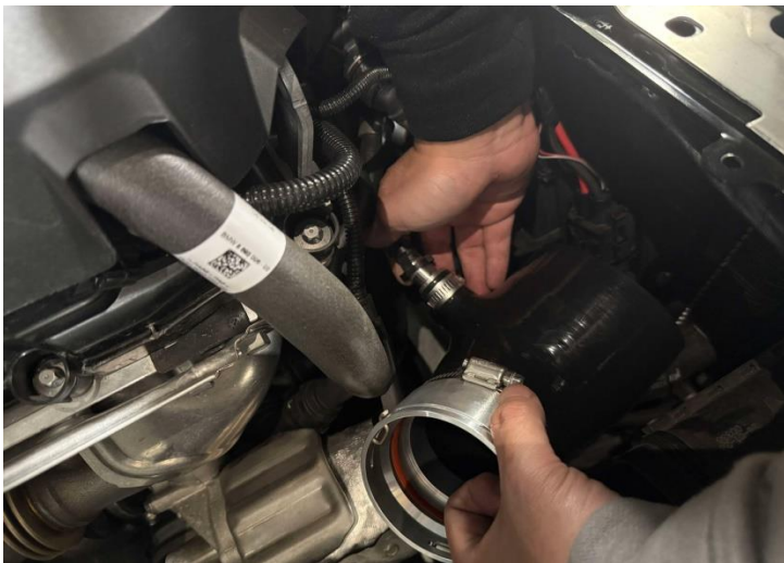
Figure 14: Before installing silicone turbo inlet, please connect the PCV hose first.
