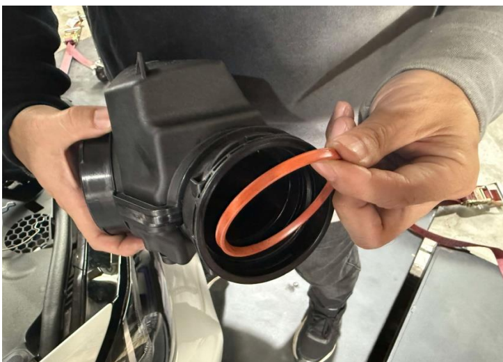
Figure 9: Remove the stock turbo inlet tube seal.
