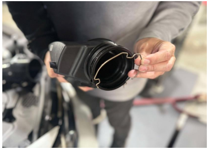
Figure 10: Remove the spring clip clamp.
