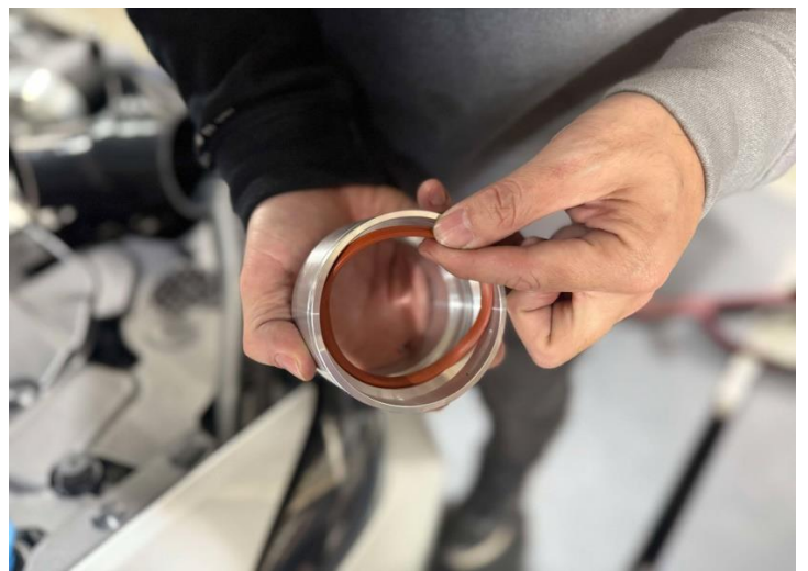
Figure 11: Install stock seal on the MST inlet adapter.
