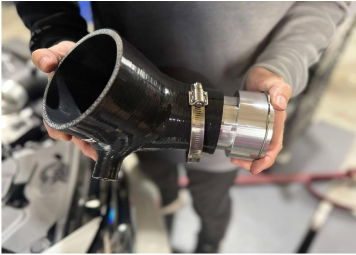
Figure 13: Install adapter on the MST silicone hose.
