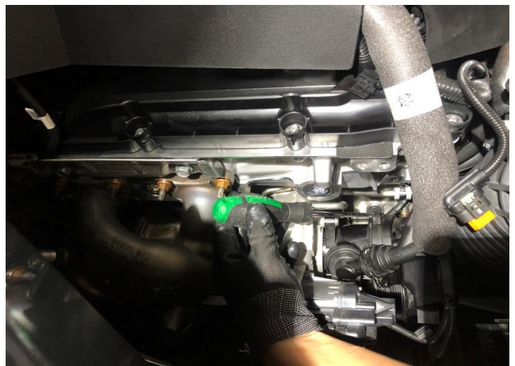
Figure 6: Remove the stock turbo inlet pipe spring.
