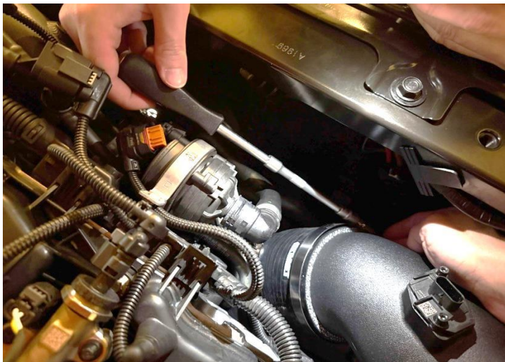
Figure 20: Tight the clamp.
