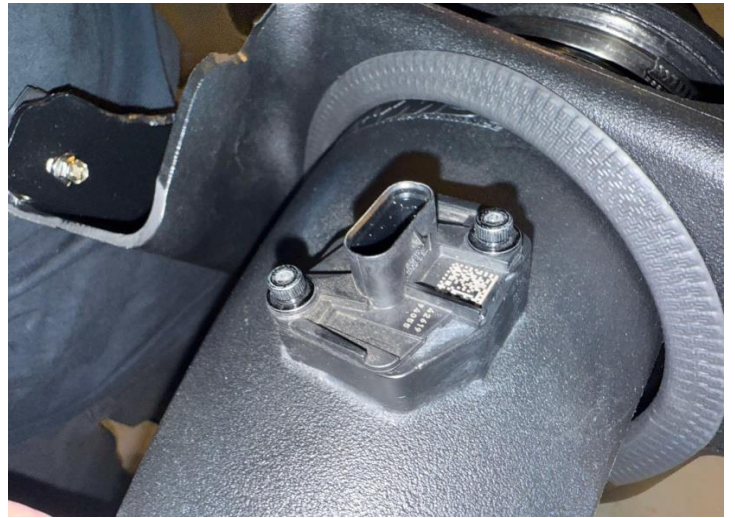
Figure 17: Install the MAF sensor on the tube.
