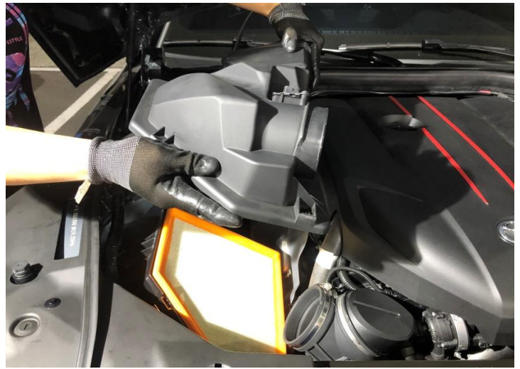
Figure 5: Remove stock air box cover.
