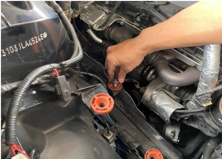
Figure 13: Install the alu mount.
