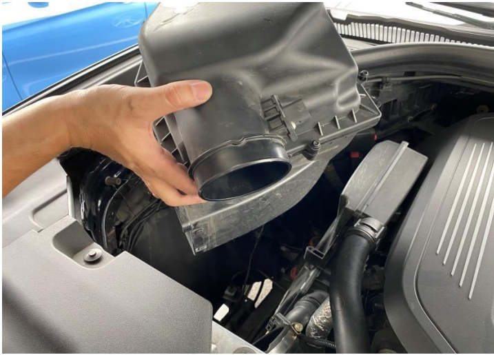
Figure 7: Remove stock air box.
