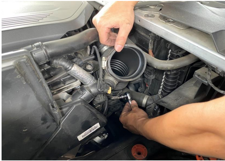
Figure 8: Remove the stock hose.
