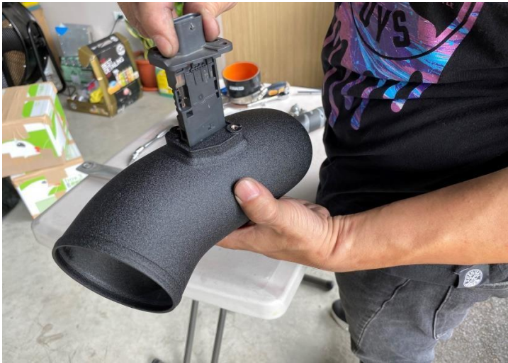
Figure 19: Install stock mass air sensor into the intake pipe and secure the m4bolt.
