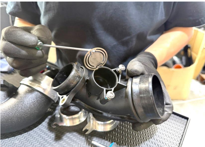
Figure 14: Remove the breather assembly from the inlet. There is also a metal shim inside the breather hole of the inlet.
