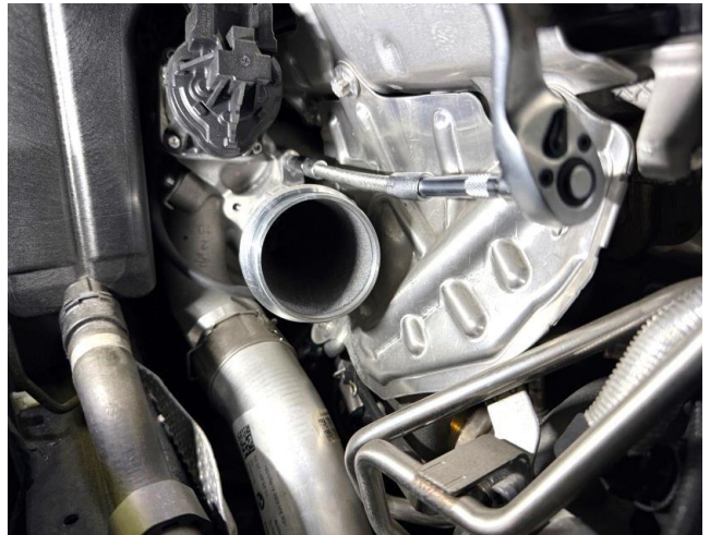
Figure 10: Remove the bolts and stock turbo inlet from the turbo.
