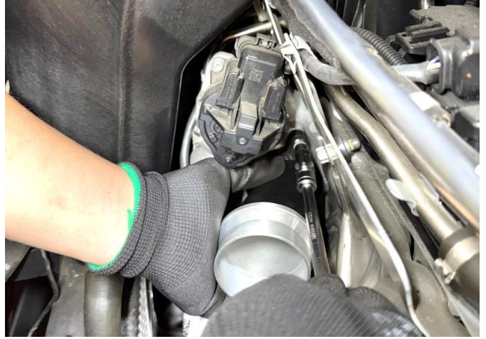
Figure 22: Install the MST turbo inlet and use M6 bolts to tighten
