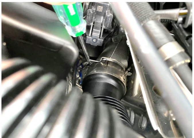
Figure 6: Remove the wire clips.
