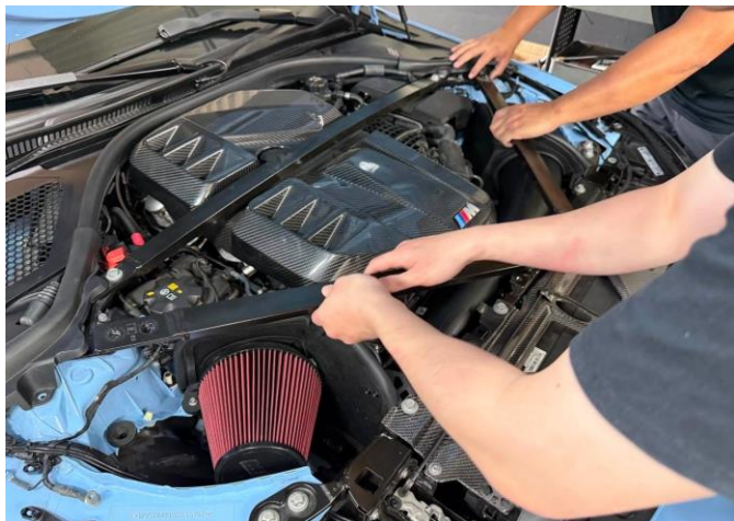
Figure 39: Reinstall the engine strut bar.
