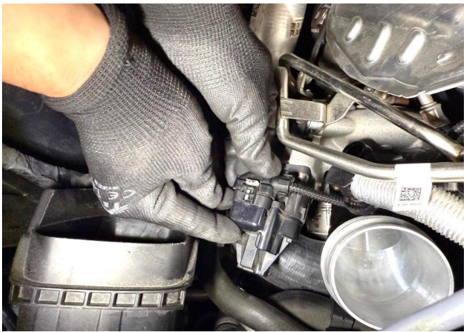
Figure 20: Connect the breather hose and sensor.
