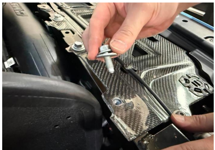
Figure 36: Remove the OEM radiator cover bolt.
