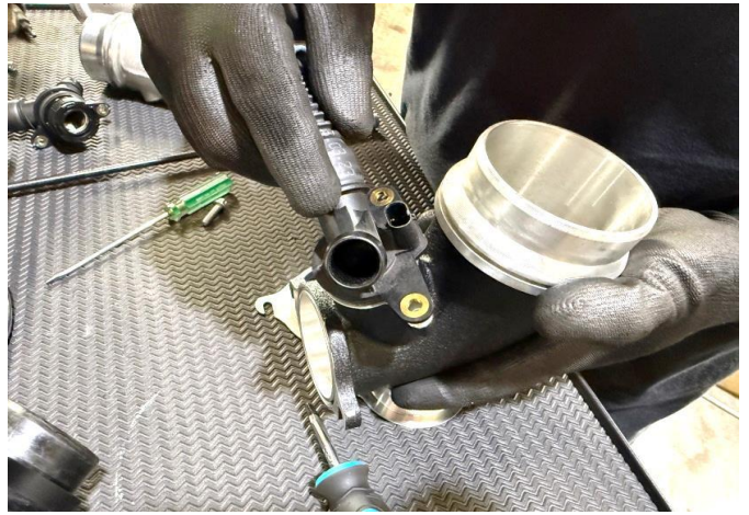
Figure 16: Secure the breather assembly onto the inlet using the OEM bolts.
