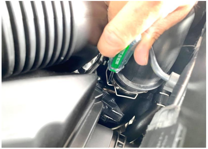
Figure 4: Remove the wire clips.
