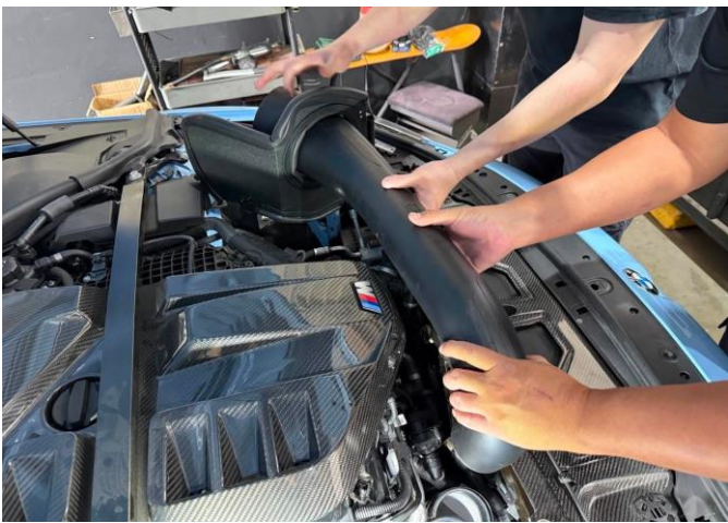
Figure 26: Install the right-side intake tube. First, insert the intake tube into the heat shield.
