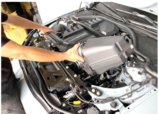
Figure 5: Remove the tube and air box.
