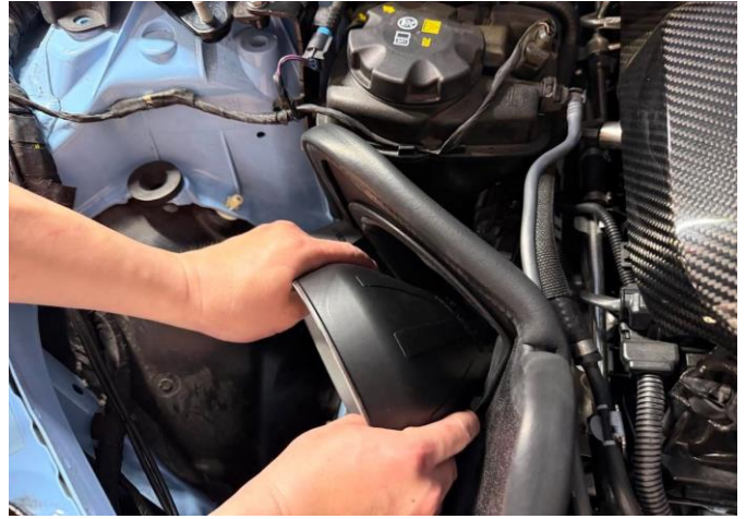
Figure 34: Install the intake tube and connect the turbo inlet.
