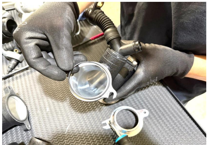
Figure 17: Install the o-ring on the MST turbo inlet.
