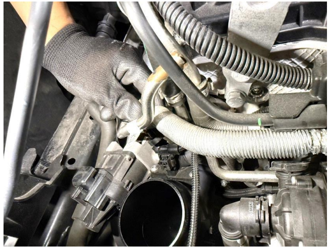
Figure 11: Disconnect the breather tube.
