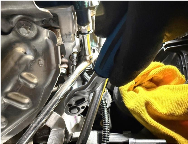
Figure 13: Remove the breather hose bolt, unclip from the engine side and you can pull this out
