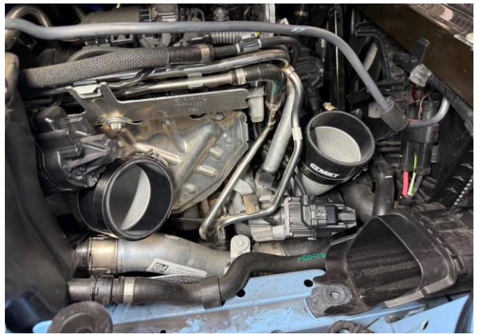
Figure 23: Install the silicone hose onto the turbo inlet.
