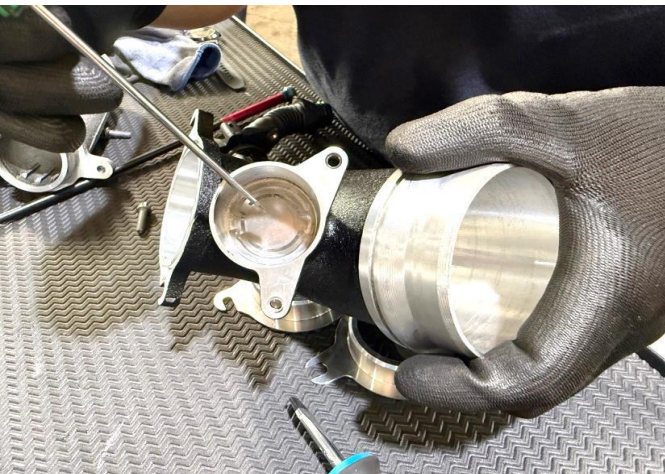
Figure 15: Insert the metal shim into the new inlet as shown. The notch should line up with the tab on the inside.
