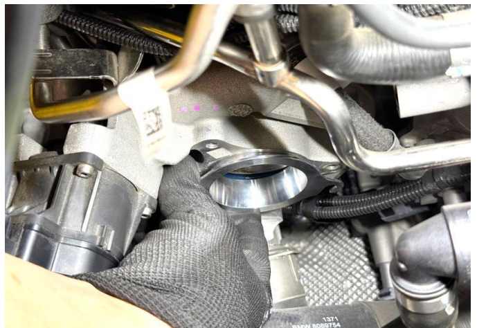
Figure 18: If the vehicle is a stock turbo, please install the MST adapter to ensure the best air flow rate. If it is a hybrid turbo, do not need to install it.
