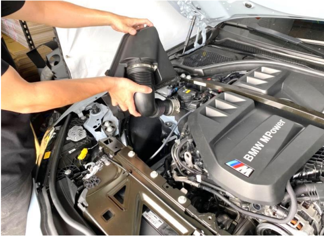
Figure 7: Remove the tube and air box.
