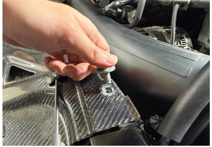
Figure 28: Remove the OEM radiator cover bolt.
