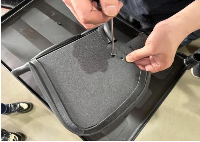
Figure 25: Install the bracket onto the heat shield.
