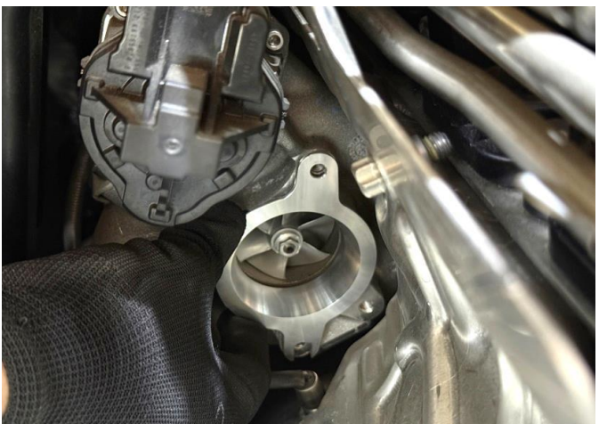
Figure 21: If the vehicle is a stock turbo, please install the MST adapter to ensure the best air flow rate. If it is a hybrid turbo, do not need to install it.
