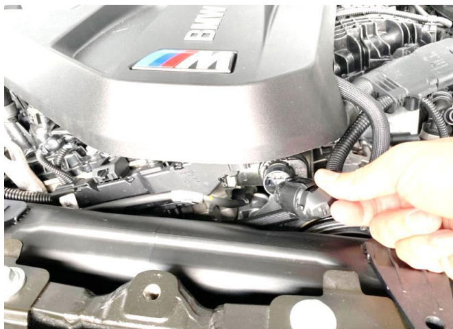
Figure 3: Disconnect the sensor.
