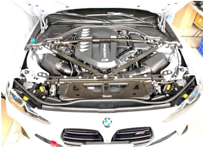
Figure 1: Stock air box. Remove 15mm 13mm bolts center and the strut brace.
