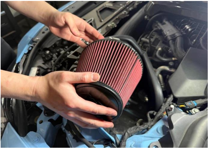
Figure 32: Install the MST filter.
