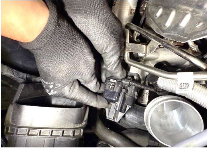
Figure 13: Connect the breather hose and sensor.
