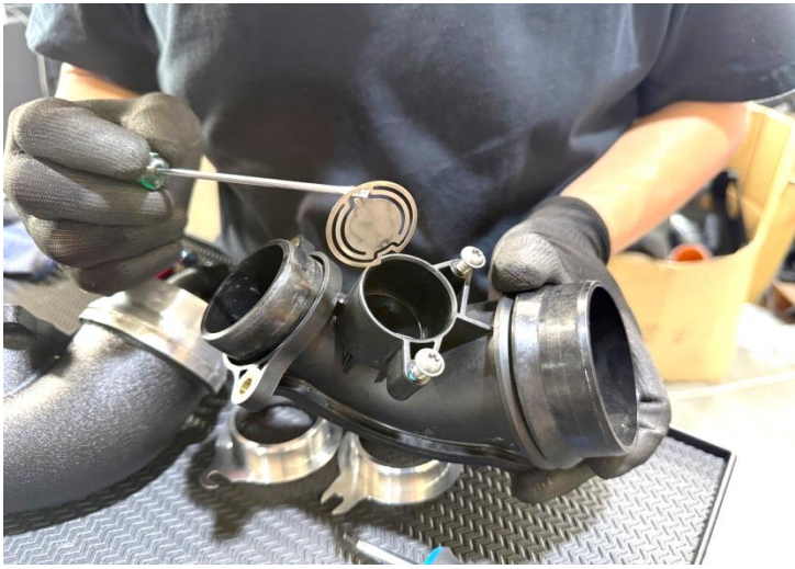
Figure 7: Remove the breather assembly from the inlet. There is also a metal shim inside the breather hole of the inlet.
