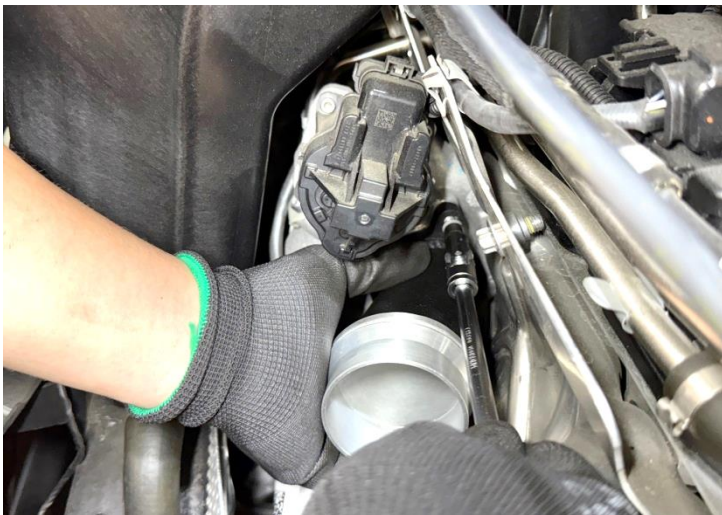
Figure 15: Install the MST turbo inlet and use M6 bolts to tighten
