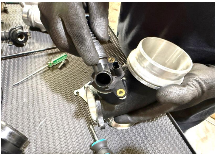
Figure 9: Secure the breather assembly onto the inlet using the OEM bolts.
