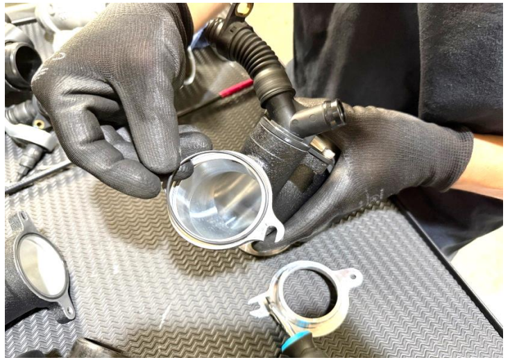
Figure 10: Install the o-ring on the MST turbo inlet.
