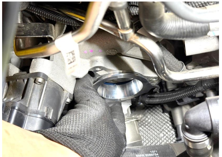
Figure 11: If the vehicle is a stock turbo, please install the MST adapter to ensure the best air flow rate. If it is a hybrid turbo, do not need to install it.
