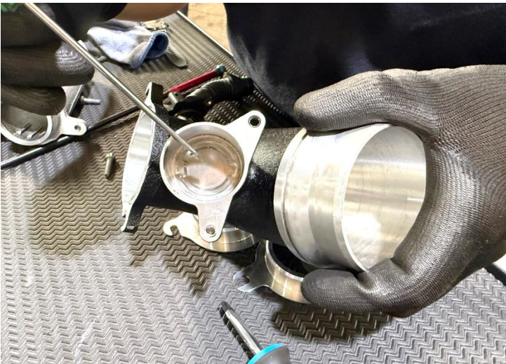
Figure 8: Insert the metal shim into the new inlet as shown. The notch should line up with the tab on the inside.
