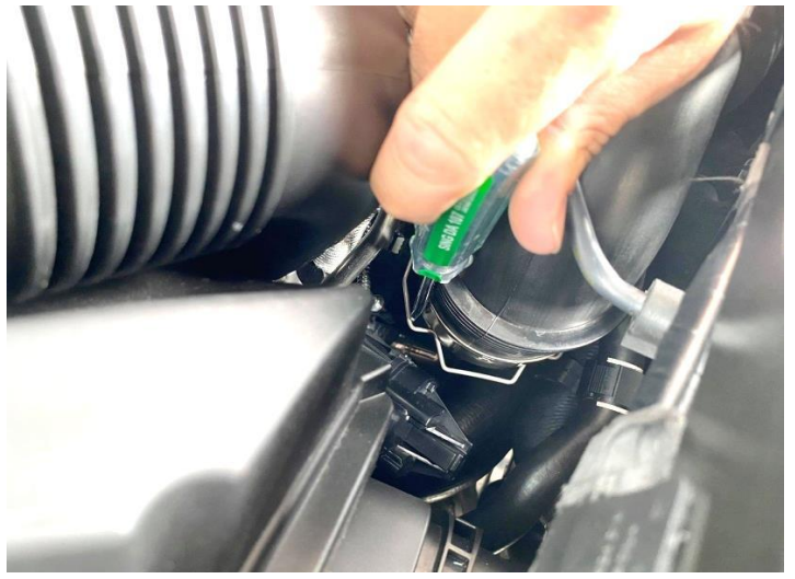
Figure 4: Remove the wire clips.
