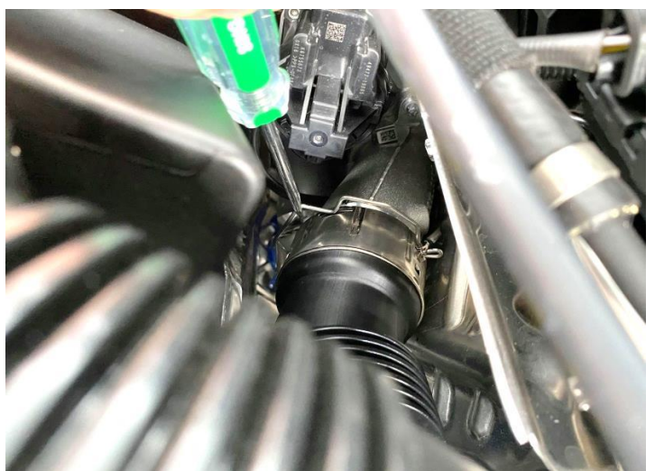
Figure 6: Remove the wire clips.
