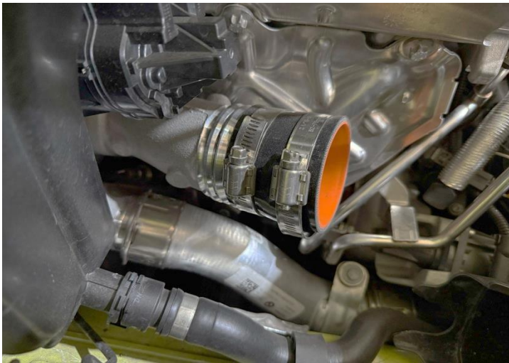
Figure 8: Install silicone hose on the turbo.
