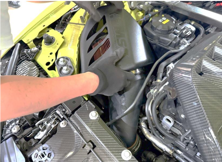
Figure 12: Install the MST tube and heatshield.
