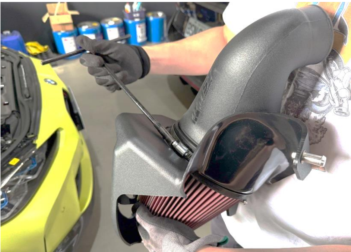
Figure 11: Install the MST air filter.
