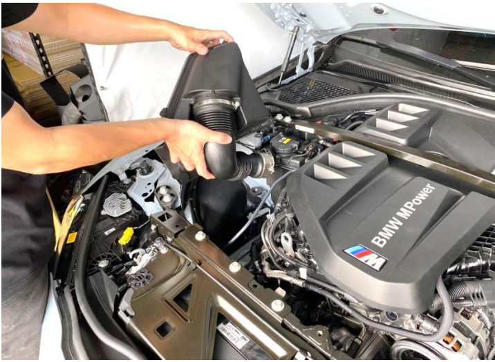
Figure 7: Remove the tube and air box.
