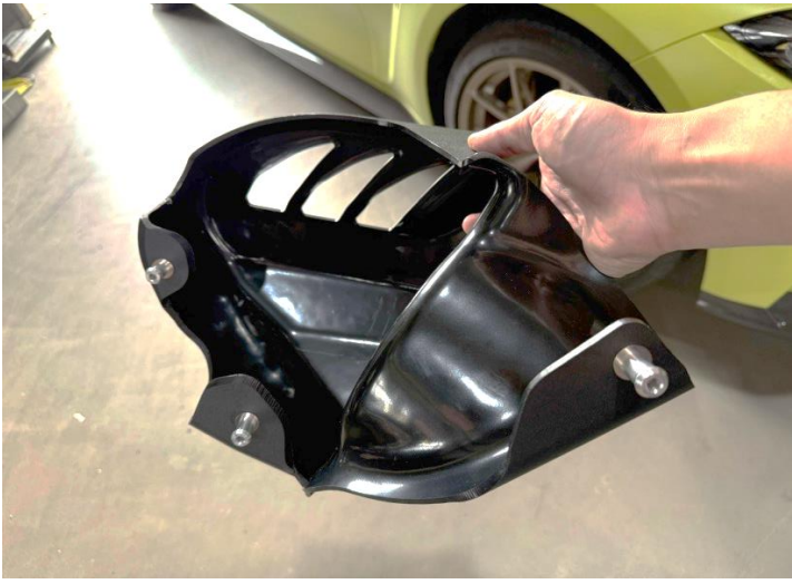
Figure 10: Install the ALU mount on heatshield. x 3.
