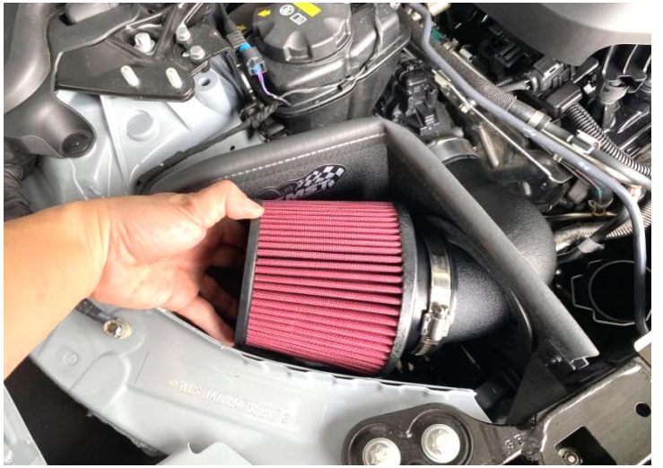
Figure 16: Install the MST air filter.
