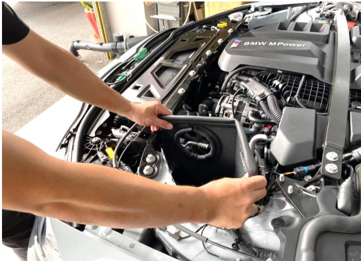
Figure 9: Install the heatshield x 2.
