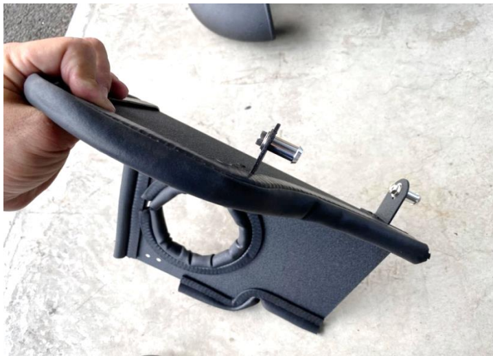
Figure 8: Install the ALU mount on heatshield.
