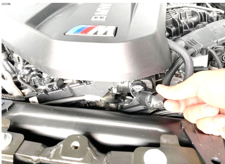
Figure 3: Disconnect the sensor.
