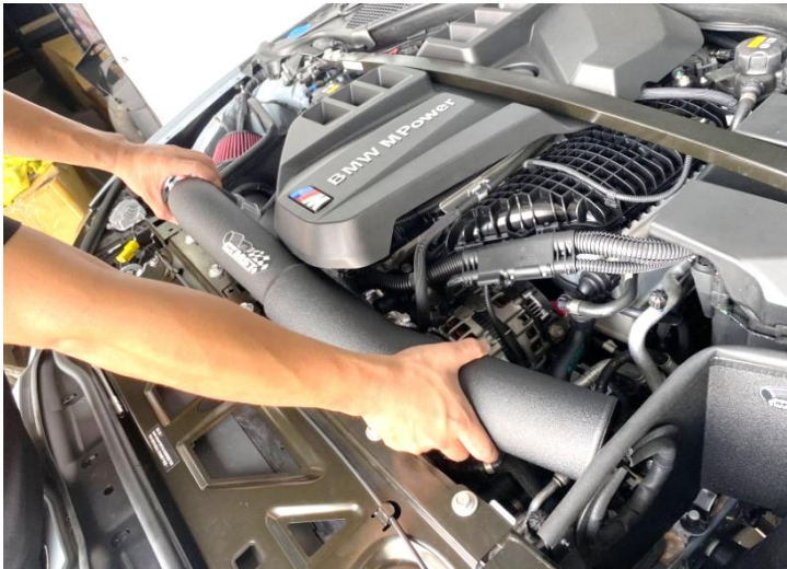
Figure 14: Install the MST tube.
