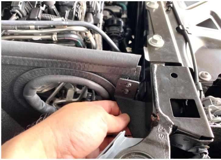
Figure 10: Install the heatshield bracket x 2.
