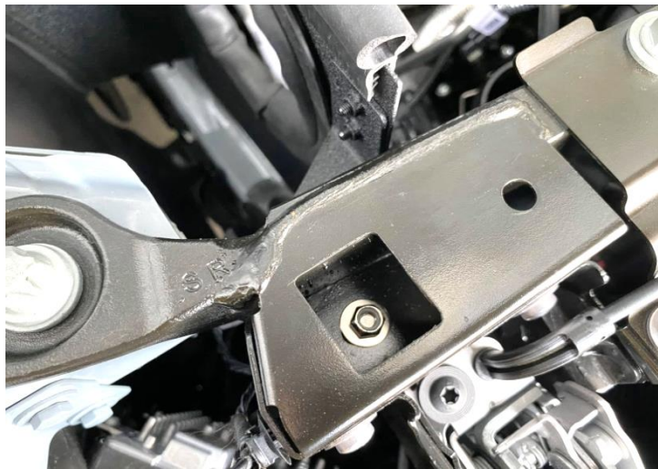
Figure 11: Secure the M6 nut.
