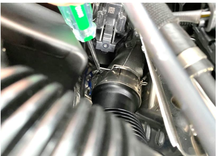
Figure 6: Remove the wire clips.
