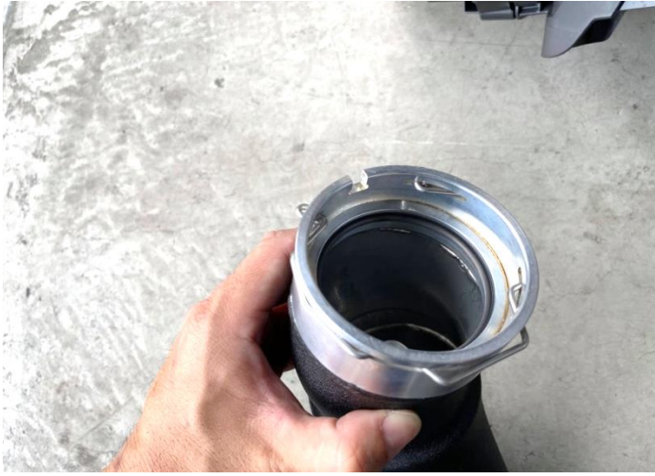
Figure 13: install the wire clips and o-ring on MST tube x 2.
