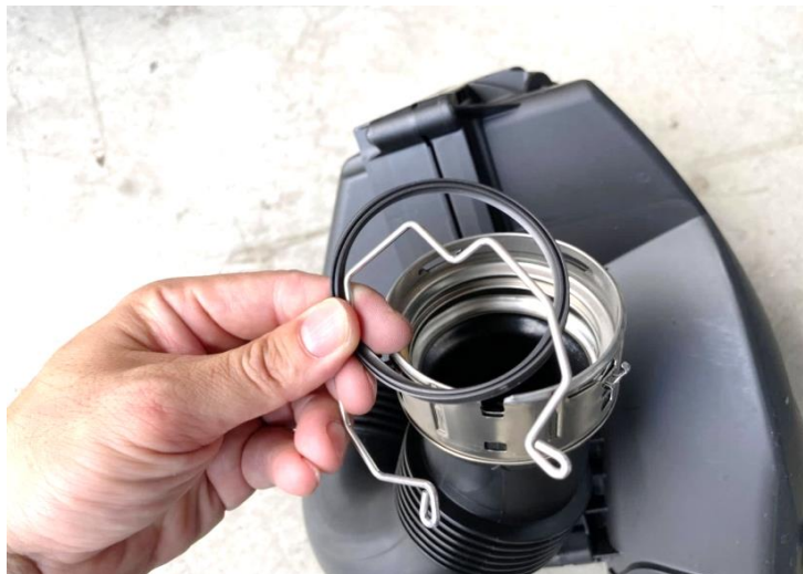
Figure 12: Remove the wire clips and o-ring from stock tube x 2.
