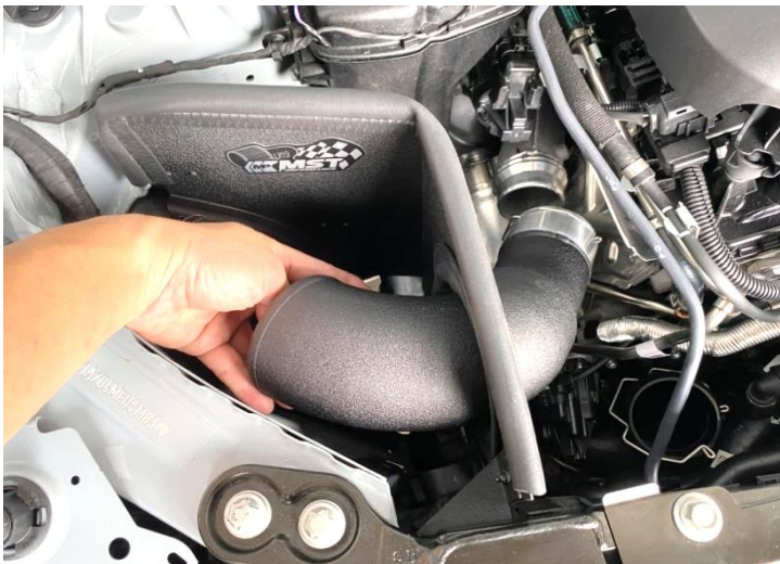
Figure 15: Install the MST tube.
