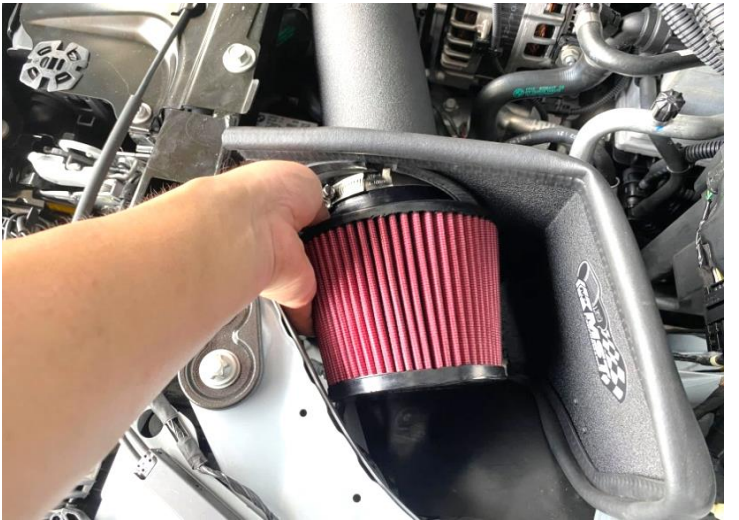
Figure 17: Install the MST air filter.
