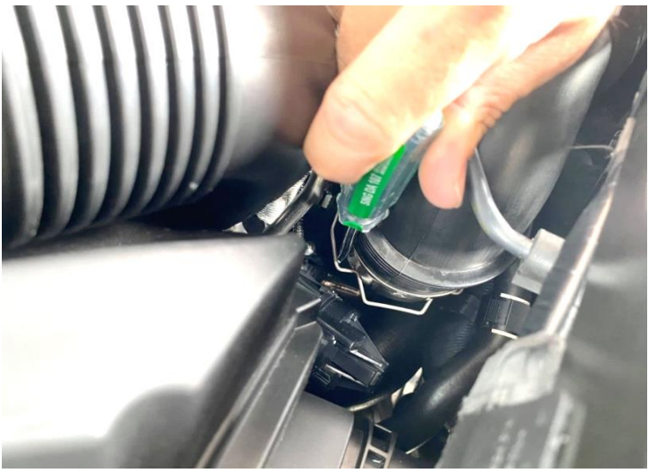
Figure 4: Remove the wire clips.
