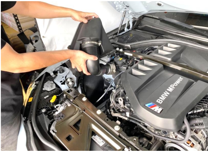
Figure 7: Remove the tube and air box.
