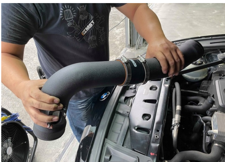
Figure 11: Install the intake pipe.安裝進水管
