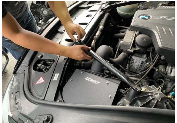
Figure 16: Install the strut bar.安裝支撐桿
