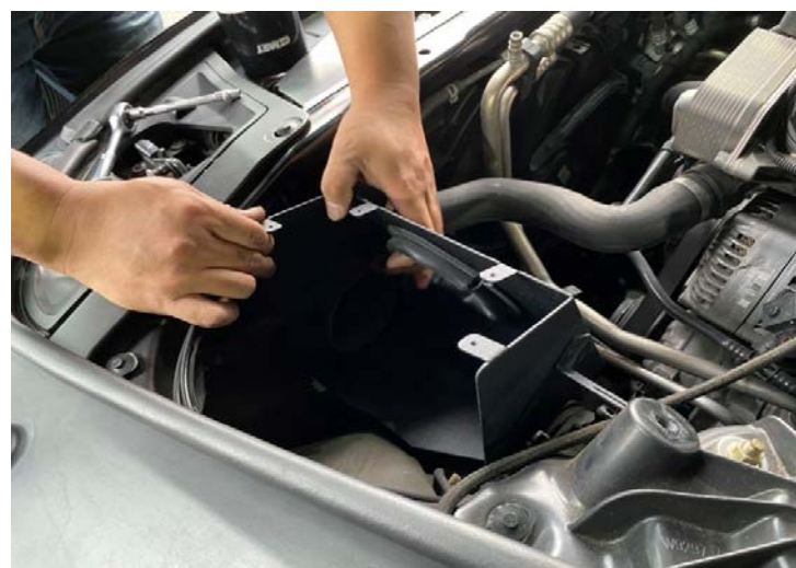
Figure 9: Install the heat shield.安裝隔熱罩
