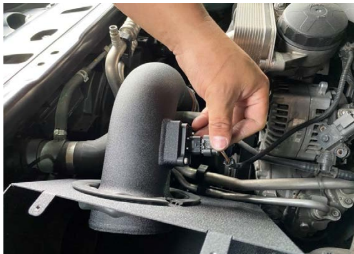
Figure 14: Connect the MAF sensor.連接MAF感應器
