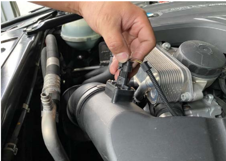
Figure 3: Disconnect the MAF sensor. 斷開MAF感應器的連接
