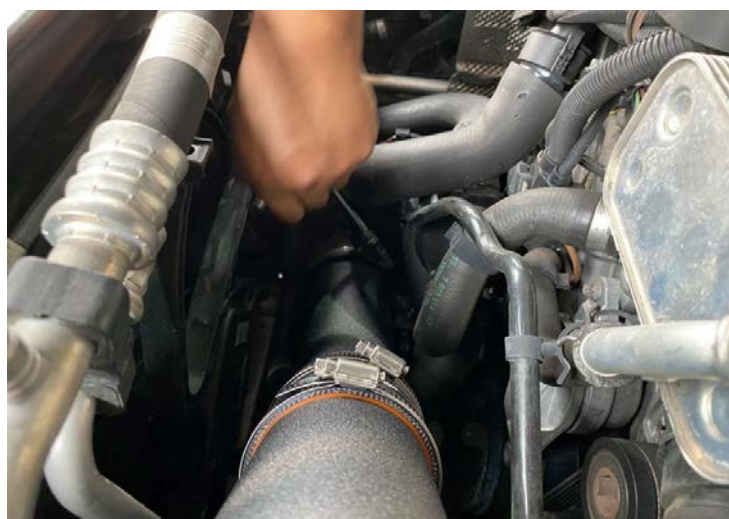
Figure 12: Tight the clamp.擰緊夾子
