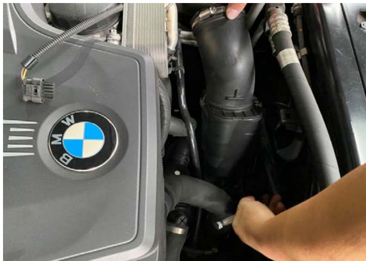
Figure 7: Remove the stock tube.拆下原廠管
