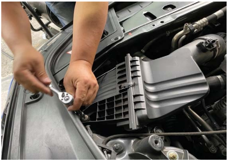
Figure 5: Remove the air box bolt. 拆下集氣箱螺栓
