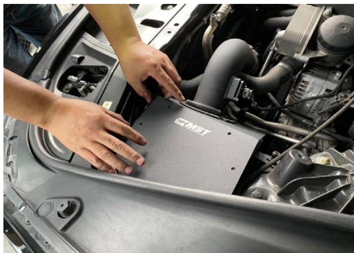
Figure 14: Connect the MAF sensor.連接MAF感應器
