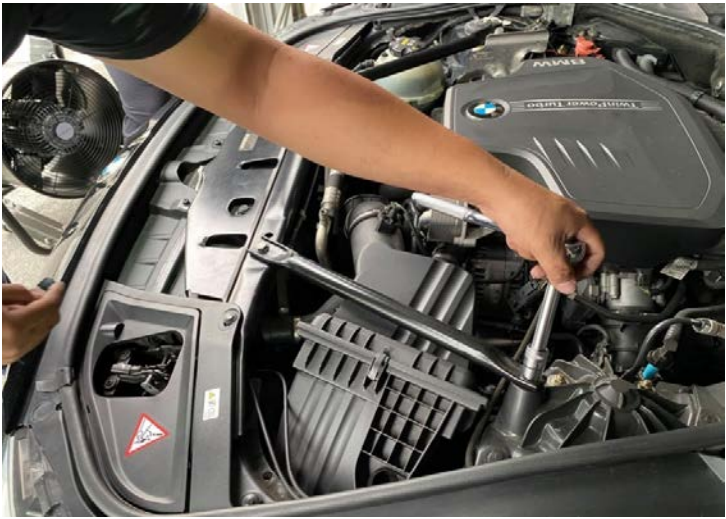
Figure 2: Remove the strut bar. 拆下支柱桿
