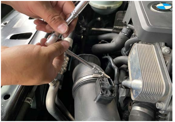
Figure 4: Loosen the stock tube clamp. 鬆開原廠管夾
