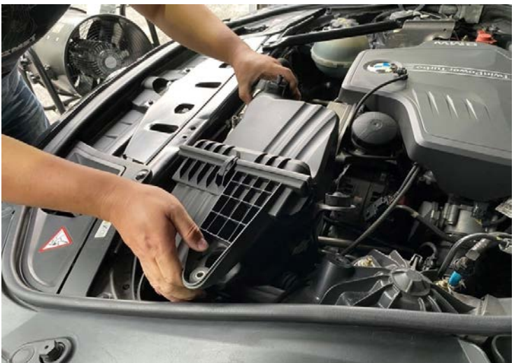
Figure 6: Remove the stock air box. 拆下原廠集氣箱
