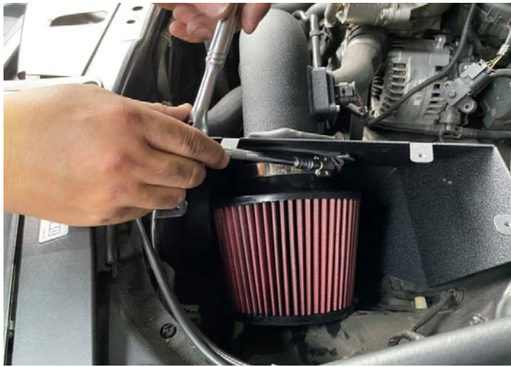
Figure 13: Install the air filter.安裝空氣過濾器
