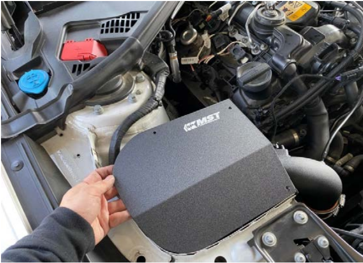
Figure 30: Install the heat shield cover .安裝隔熱罩
