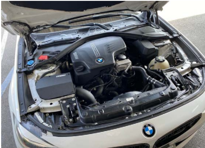
Figure 31: Congratulations! You have just completed the installation of this intake system. Periodically, check the alignment of the intake, normal wear and tear can cause nuts and bolts to come loose. 恭喜！您剛剛完成了此進氣系統的安裝。定期檢查進氣口的對準情況，正常磨損會導致螺帽和螺栓鬆脫
