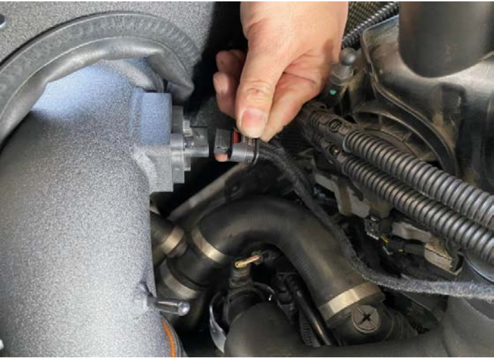
Figure 27: Connect the sensor.連接感應器
