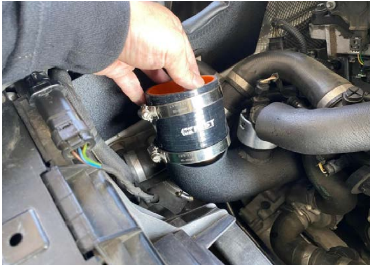
Figure 24: Install the silicone hose.安裝矽膠管
