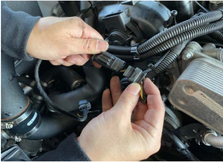
Figure 26: Electrical extensions to plug them back in to the factory wiring harness. 電氣擴充裝置可將其插回線束
