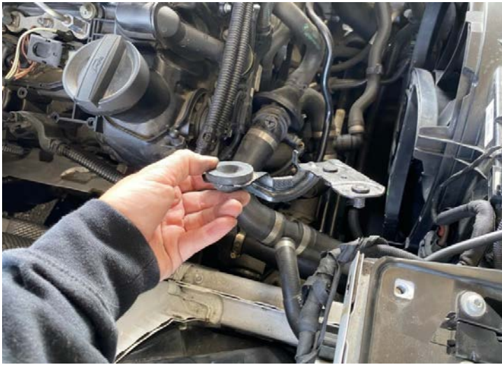
Figure 13: Remove the stock air box bracket. 拆下備用集氣箱支架
