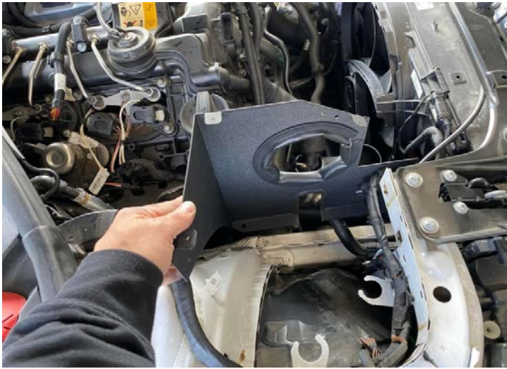
Figure 19: Install the heat shield.安裝隔熱罩
