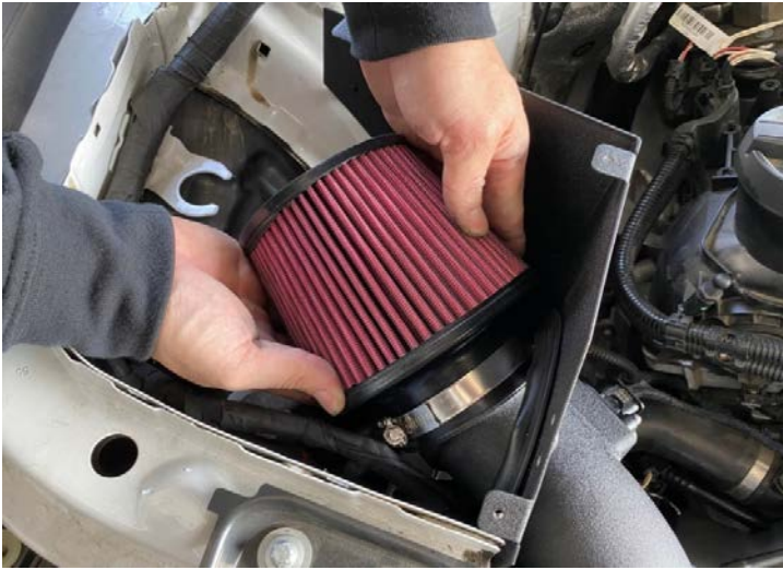
Figure 29: Install the MST filter.安裝MST高流量濾芯
