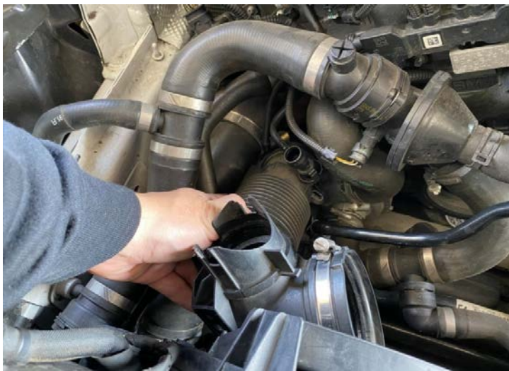
Figure 10: Remove the stock turbo inlet. 拆下原廠渦輪進口
