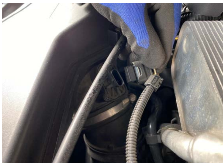
Figure 2: Disconnect the sensor. 斷開感應器連接
