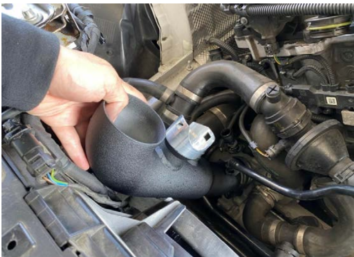
Figure 15: Install the MST turbo inlet tube. 安裝 MST 渦輪進氣管
