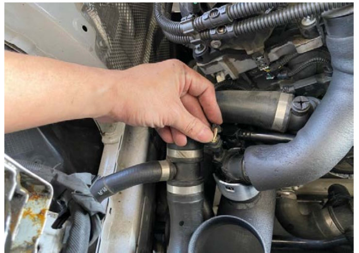
Figure 18: Connect the sensor. 連接感應器
