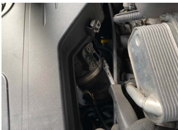
Figure 3: Loosen the stock tube clamp. 鬆開原廠管夾
