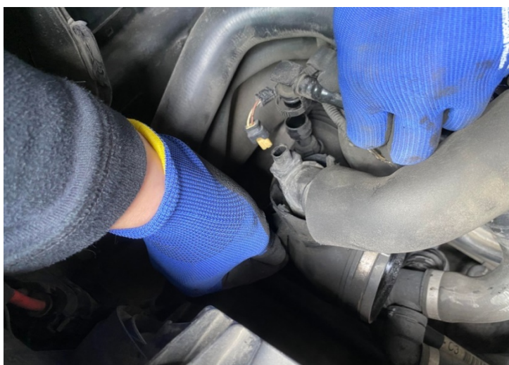
Figure 8: Remove the PCV hose.拆下 PCV 軟管
