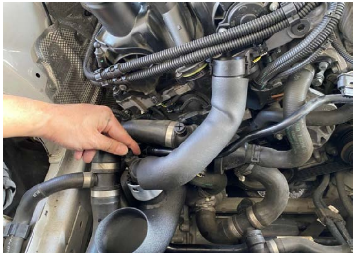
Figure 17: Install the PCV breather hose. 安裝 PCV 軟管
