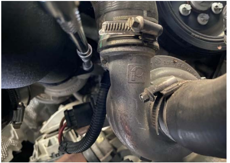
Figure 16: Tighten the turbo inlet screw. 擰緊渦輪進口螺絲
