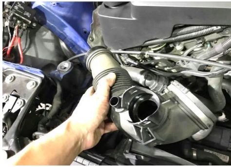
Figure 13 Once removed the nut(put it aside), pull the factory inlet tube off
