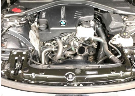
Figure 5. The appearance of after removing the airbox
