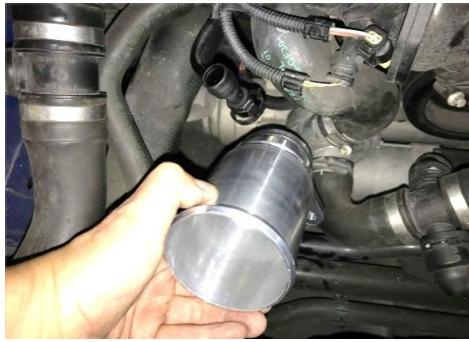
Figure 14 Take the provided piece of aluminum and install to the turbo
