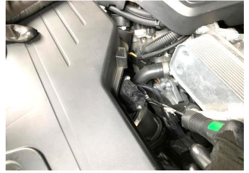
Figure 3. Loosen the band clamp as shown
