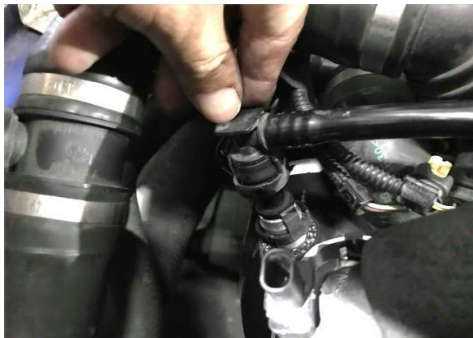
Figure 19 Then clip the other vacuum line in.
