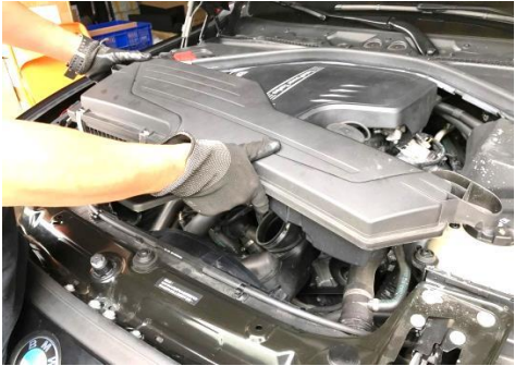
Figure 4 Remove the airbox by gently lifting up
