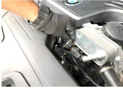
Figure 2. Gently unplug the MAF sensor connection from the MAF sensor.
