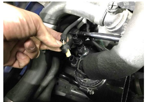
Figure9 Simply press down the tab to disconnect the connection
