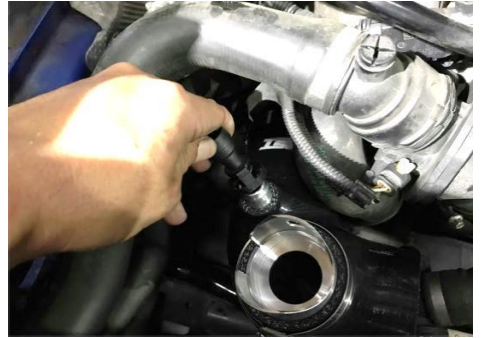
Figure 18 Take one vacuum line and put it into the hole.
