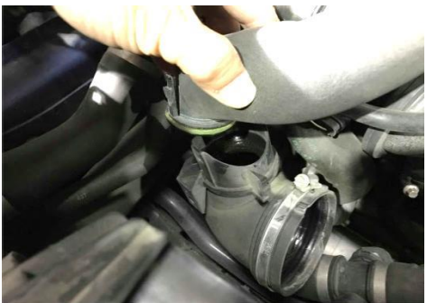
Figure 10 A little clip on the front and a little clip on the back, SQUEEZE them together and pull up the tube.
