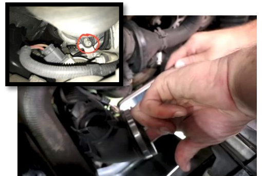
Figure12 You'll see a 10mm nut behind the OEM pipe, remove it by an 8 inch drive extension bar. *Do not do this after drove your car
