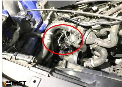
Figure 8. The appearance after remove the hose
