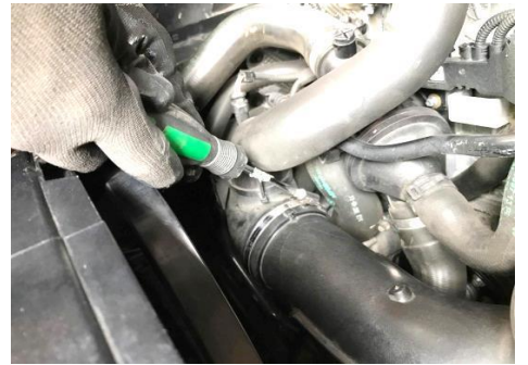
Figure 6. Loosen the fasteners that tighten the clamp
