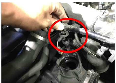
Figure 11 Remove the vacuum lines (one each on the top and bottom) by squeezing the little ring and pull it right out.
