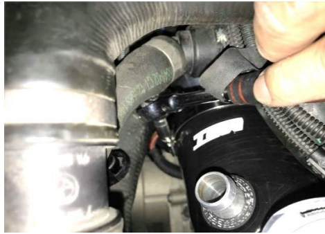
Figure 17 Secure with a provided clamp (2 3/4). (Do not overtighten)
