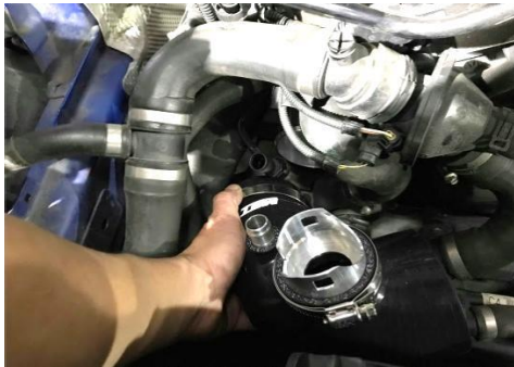
Figure 16 Slide on the MST silicone elbow to the turbo aluminum piece.
