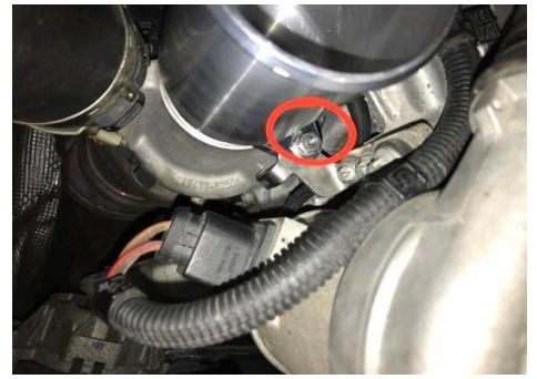
Figure 15 Once you have the thread run, secure it by tightening back the 10mm nut.
