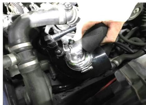
Figure 20 Install the tube with the two clips on the aluminum piece, and line that up, pop the clips back.
