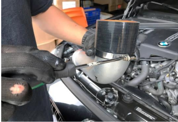
Figure 11 . Fit on the silicone hose (with a clamp on) to the pipe A and tighten them up (Do not overtighten)
