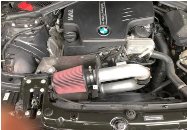
Figure 19. Secure the air filter by tightening the clamp (Do not overtighten )
