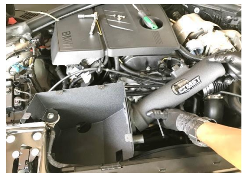
Figure 15 Install the MST intake pipe
