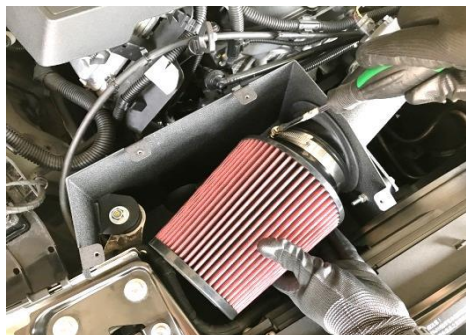
Figure 20 Tighten the clamp (Do not overtighten)
