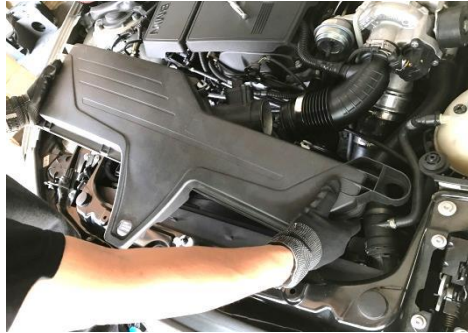
Figure 5 Remove the engine cover
