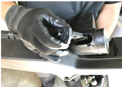
Figure 8 Saperate the sensor from the engine cover
