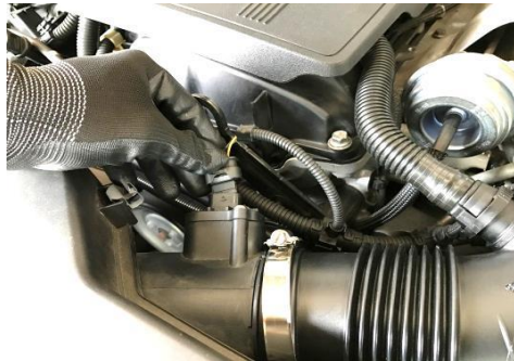
Figure 4 Disconnect the MAF sensor
