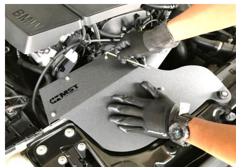
Figure 22 Install the MST heat shield cover and secure with the screws
