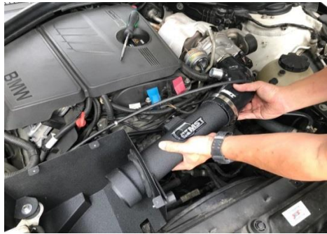
Figure 16 Connect the silicone hose and the intake pipe properly, tight the clamp (Do not overtighten)
