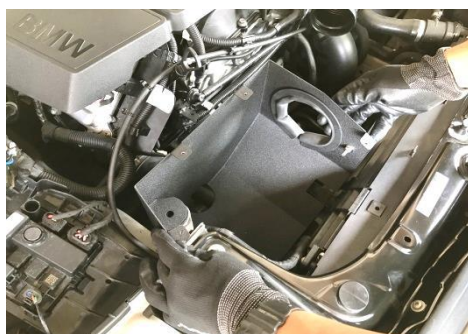
Figure 11 Install the MST heat shield
