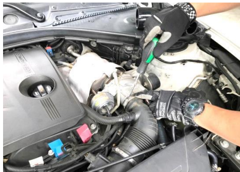
Figure 2 Loosen the clamps of stock hose
