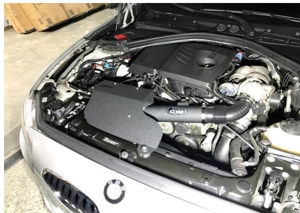
Figure 22 Install the MST heat shield cover and secure with the screws
