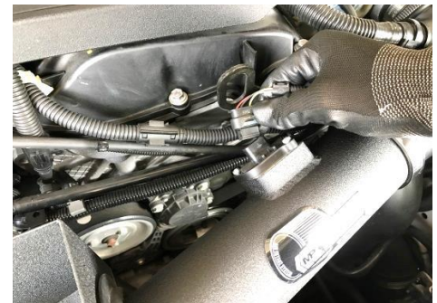
Figure 18. Connect the MAF sensor to the MST intake pipe
