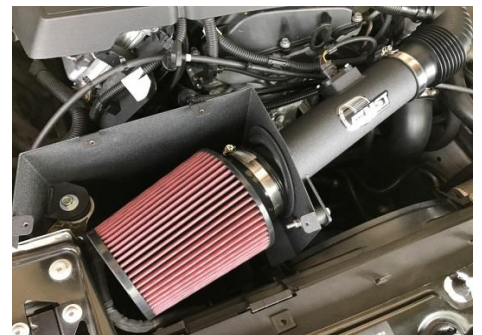
Figure 21 The overall apperance of the MST intake system
