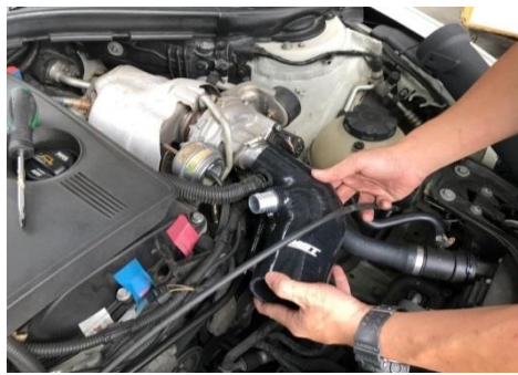
Figure 14 Install the MST silicone hose, and slide a clamp to it
