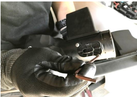
Figure 7 Unscrew the screws from the MAF sensor
