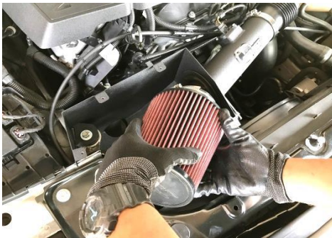
Figure 19 Install the MST filter with a provided clamp.
