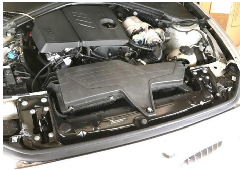
Figure 1 The stock Intake system
