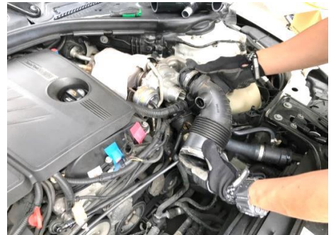
Figure 6 Remove the stock turbo inlet hose
