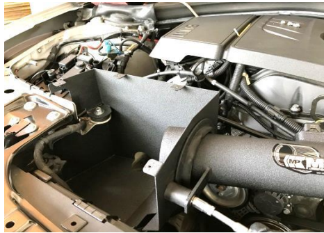
Figure 17 Overview when pipe and heat shield base are all set
