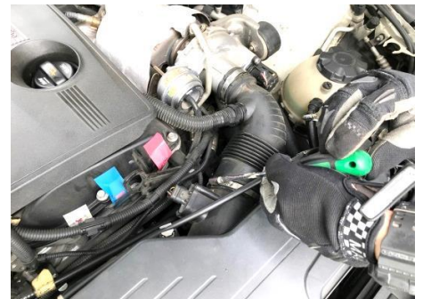
Figure 3 Loosen the clamps of stock hose
