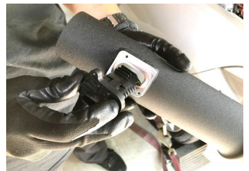
Figure9 Put the sensor to the MST intake pipe
