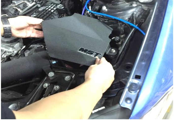
Figure 18. INSTALL TOP COVER OF HEAT SHILED. 安裝隔熱罩頂蓋
