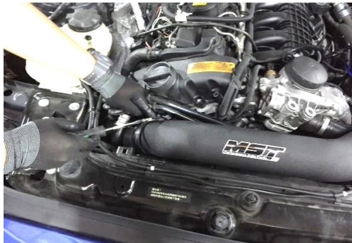
Figure 12. TIE UP HOSE CLAMP ON INTAKE PIPE. 將軟管夾固定在進氣管上
