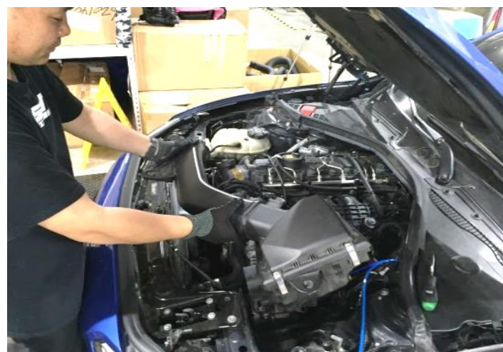
Figure 5. REMOVE STOCK AIR BOX 拆下原廠集氣箱
