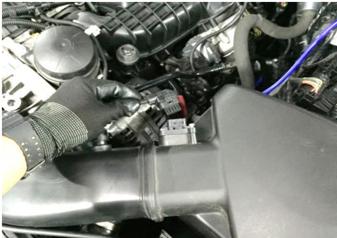
Figure 3. CAREFULLY DISCONNECT MAF SENSOR WIRING. 小心斷開 MAF 感應器接線
