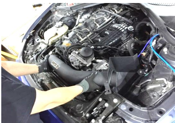
Figure 11. INSTALL INTAKE PIPE AS SHOWN. 如圖所示安裝進氣管
