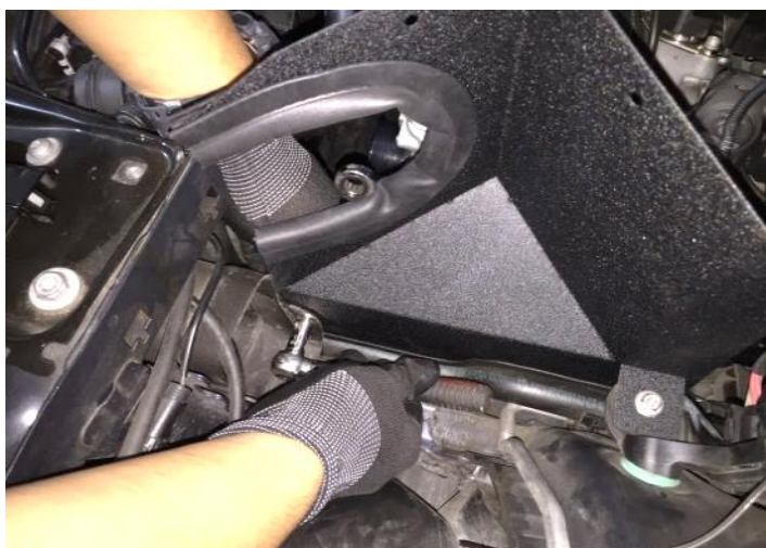
Figure 9. TIE UP M6 BOLT/NUT/WASHER(X2) AS SHOWN ONTO HEAT SHIELD. 如圖將 M6 螺栓/螺帽/墊圈 (X2) 固定在隔熱罩上
