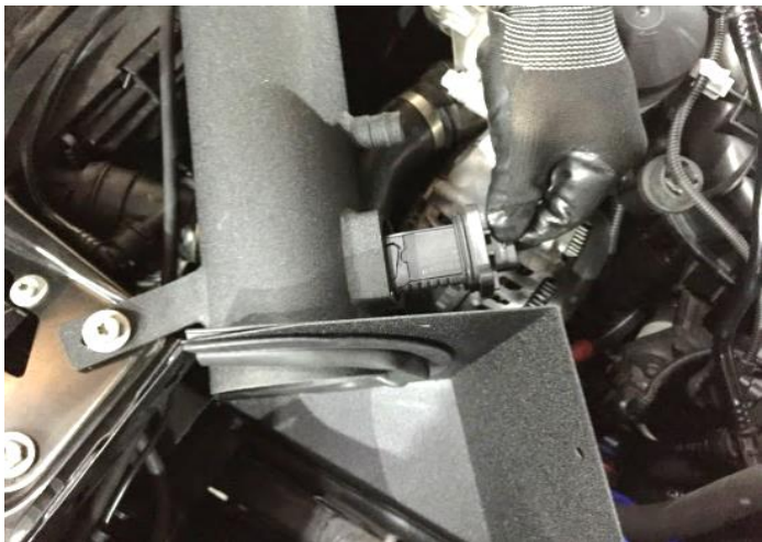
Figure 15. INSTALL MAF SENSOR INTO INTAKE PIPE. 將 MAF 感應器安裝到進氣管中
