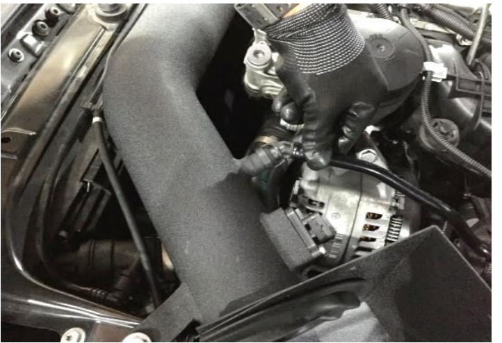
Figure 16. RECONNECT THE CRANK CASE VENT LINE ONTO INTAKE TUBE. 將曲軸箱通風管重新連接到進氣管上
