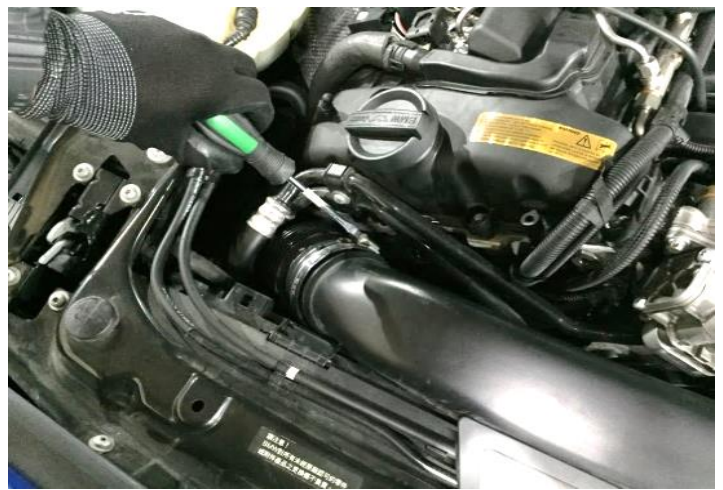
Figure 2. LOOSEN HOSE CLAMP OF THE INTAKE PIPE BY PROPER TOOL. 用適當的工具鬆開進氣管的軟管夾
