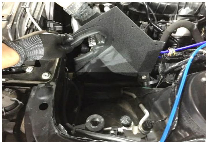
Figure 8. INSTALL HEAT SHIELD IN PLACE AS SHOWN. 如圖所示將隔熱罩安裝到位
