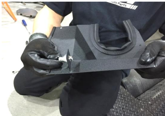
Figure 7. INSTALL ANOTHER HEAT SHIELD MOUNT ON HEAT SHIELD AS SHOWN. 如圖所示，在隔熱罩上安裝另一個隔熱罩安裝座
