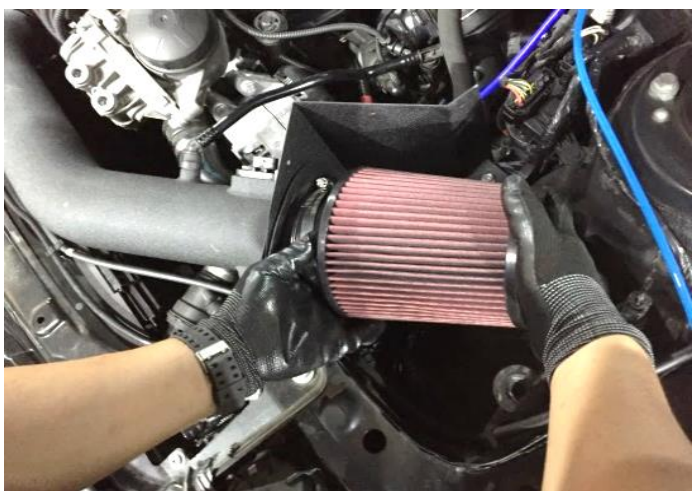
Figure 17. INSTALL AIR FILTER AND TIE UP HOSE CLAMP. 安裝高流量濾芯和紮緊軟管夾
