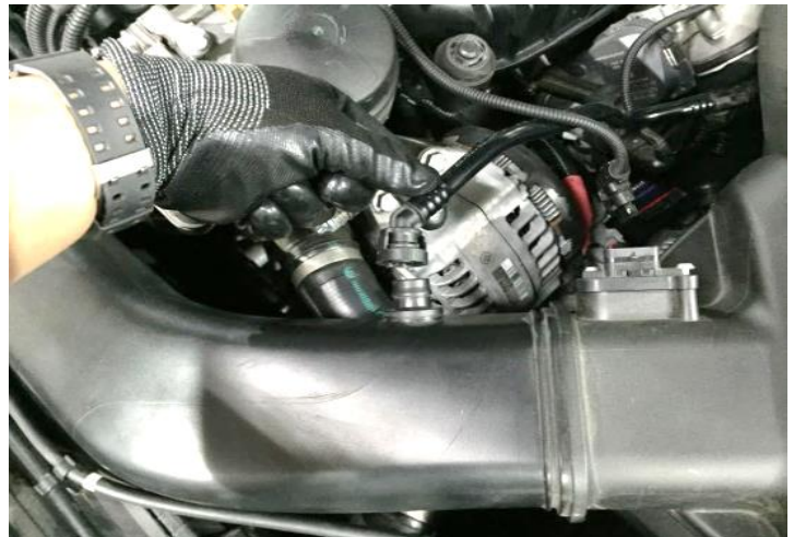
Figure 4. DISCONNECT THE CRANK CASE VENT LINE FROM FACTORY INTAKE PIPE. 斷開曲軸箱通風管與 FACTORY 進氣管的連接
