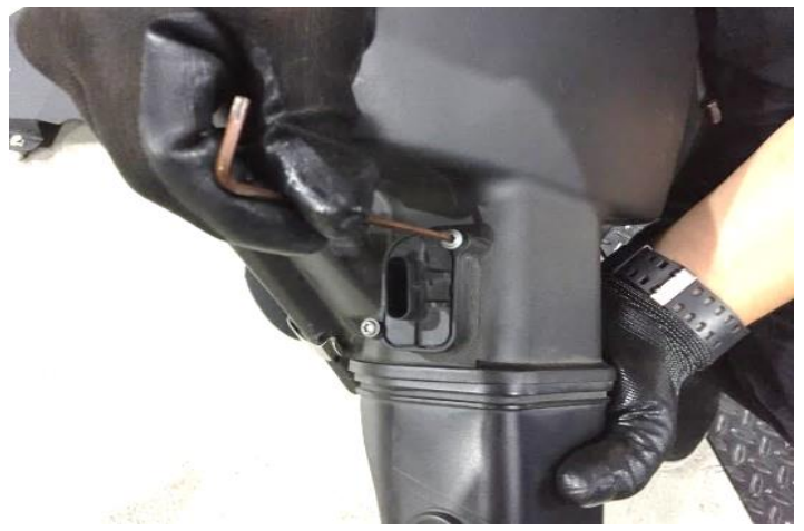
Figure 14. REMOVE MAF SENSOR FROM FACOTRY AIR BOX. 從工廠氣箱拆下 MAF 感應器
