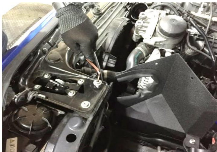
Figure 10. LOOSEN BOLT FROM FACTORY BRACKET AS SHOWN. 如圖所示，鬆開原廠支架上的螺栓
