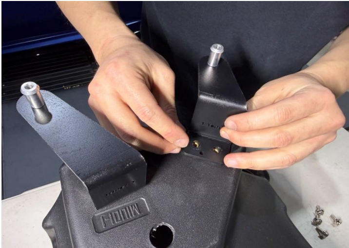
Figure 9: Install the bracket on the MST air box * 2.
