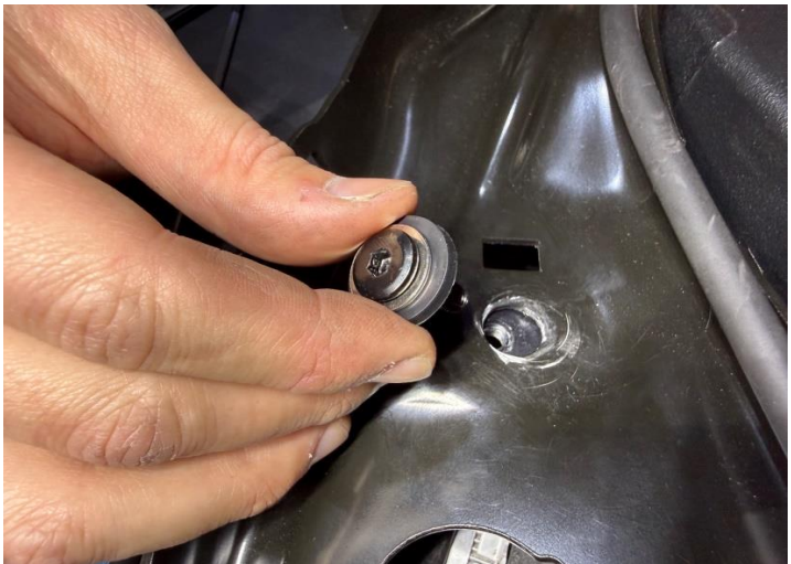
Figure 17: Secure the scoop using the bolts.
