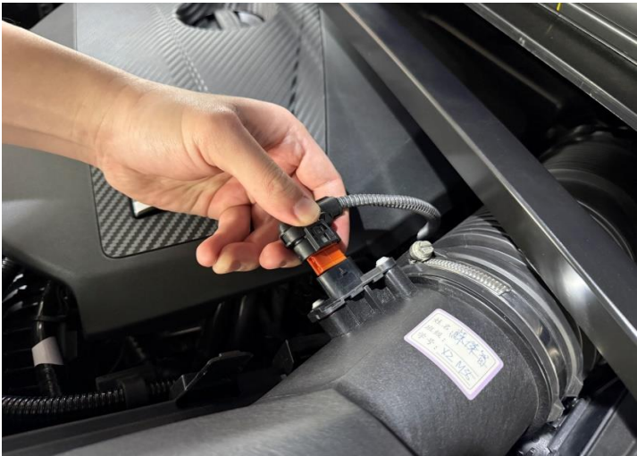
Figure 4: Disconnect the mass air sensor.
