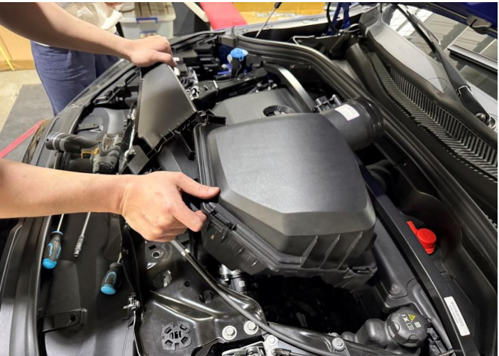
Figure 5: Remove the stock air box and scoop.
