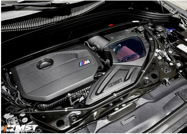
Figure 19: Congratulations! You have just completed the installation of this intake system. Periodically, check the alignment of the intake, normal wear and tear can cause nuts and bolts to come loose.
