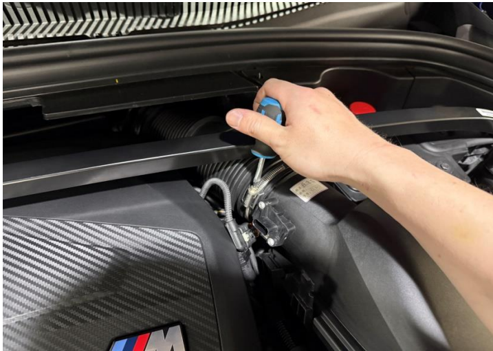
Figure 3: Loosen the hose clamp.
