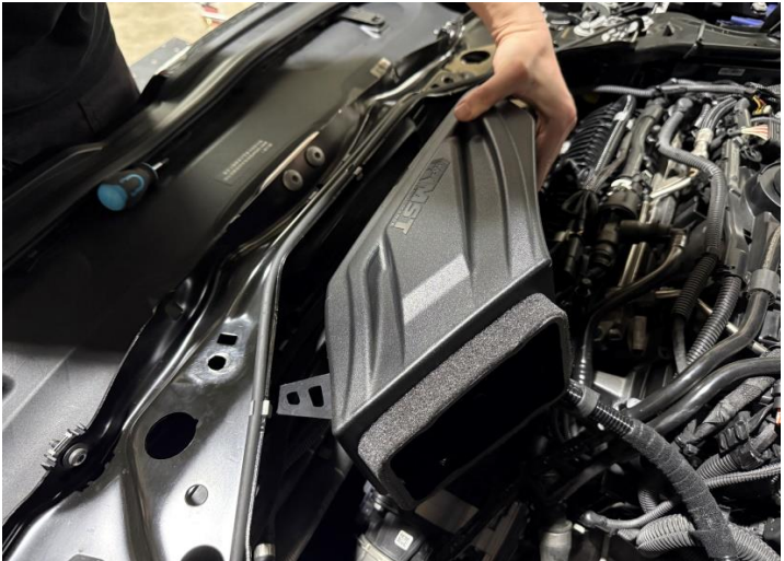
Figure 11: Install the MST scoop, but do not tighten the bolts yet.
