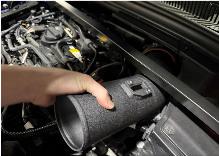
Figure 13: Install the MST tube.
