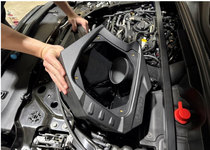
Figure 14: Install the MST air box.
