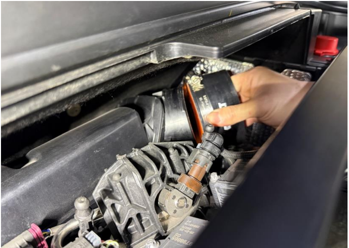
Figure 12: . Install the MST silicone hose.
