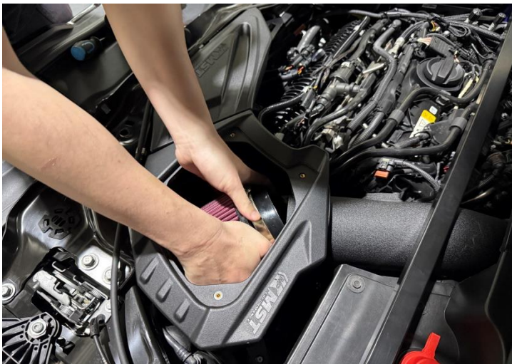
Figure 15: Install the MST air filter.
