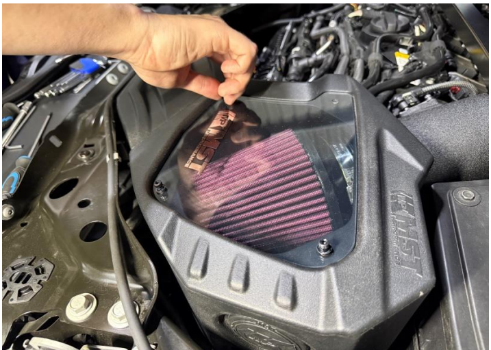
Figure 18: Install the air box cover.
