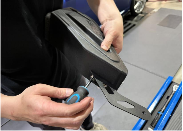
Figure 10: Install the bracket on the MST scoop * 2.
