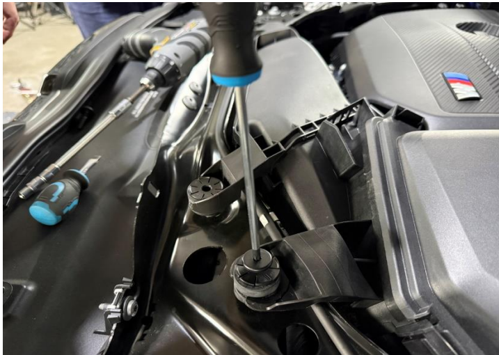
Figure 2: Remove the stock air box and scoop bolts x 3
