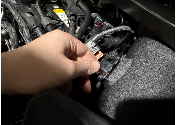
Figure 16: Install the stock MAF sensor and connect.
