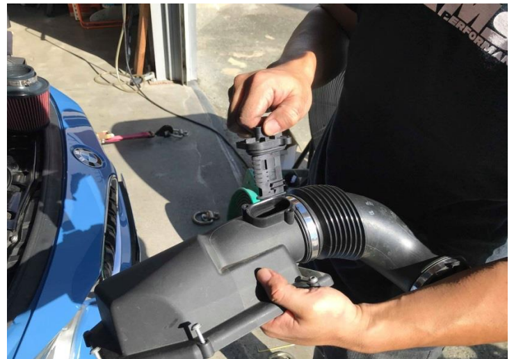
Figure 23: Remove the mass air flow sensor from the stock air box.
