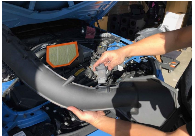
Figure 10: Remove the mass air flow sensor from the stock air box.
