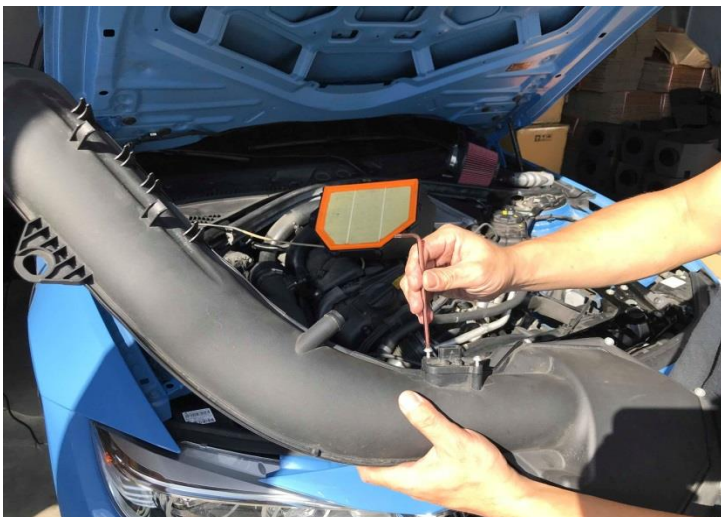
Figure 9: Remove the mass air flow sensor from the stock air box.
