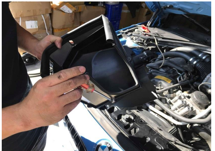
Figure 12: Install the heat shield on the top of air box and secure with bolts.
