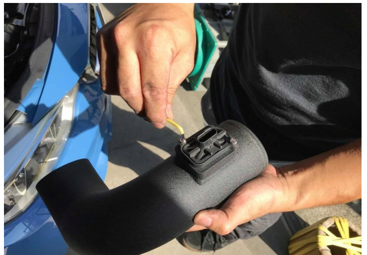
Figure 24: Install mass air sensor into the intake tube.
