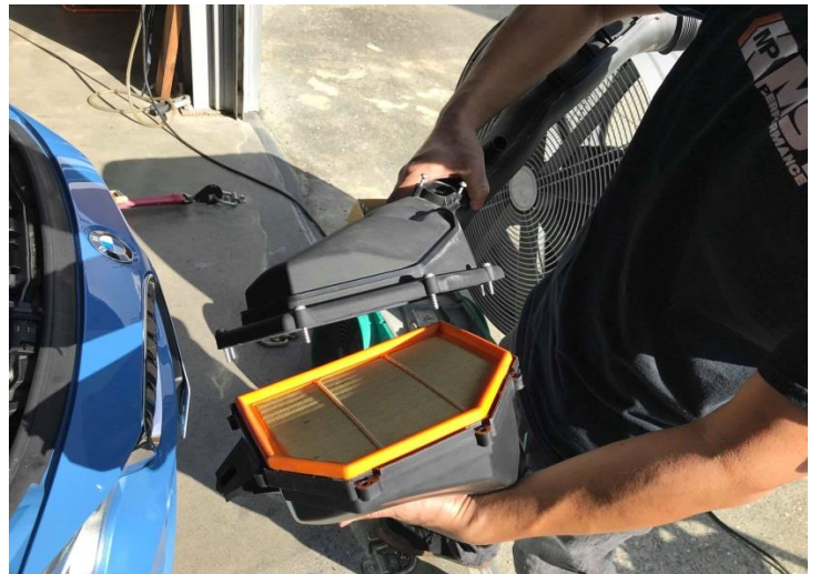
Figure 11: Remove the stock air box cover and filter.
