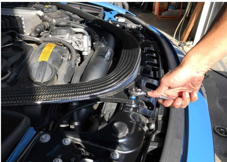
Figure 3: Remove the bolts on the struts bar. Total of 9 bolts.
