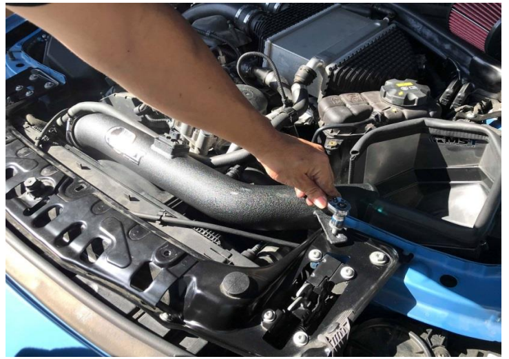
Figure 16: Secure intake tube breaket with bolt.
