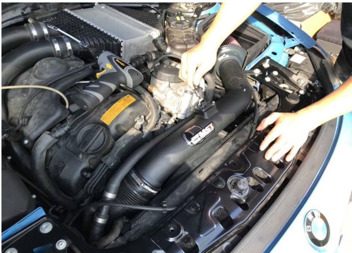
Figure 20: Plug in the mass air flow sensor connector.
