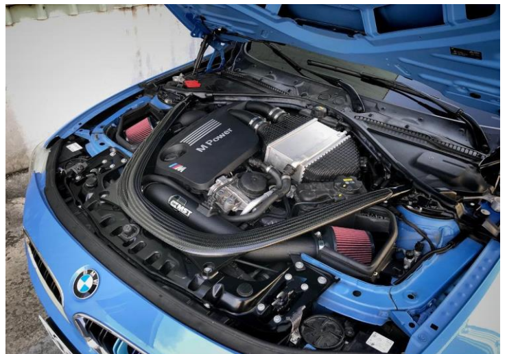
Figure 30: Congratulations! You have just completed the installation of this intake system. Periodically, check the alignment of the intake, normal wear and tear can cause nuts and bolts to come loose.
