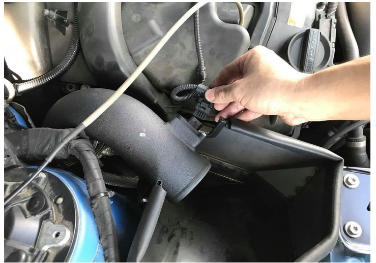
Figure 28: Plug in the mass air flow sensor connector.
