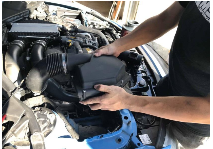
Figure 22: Remove the stock air box.
