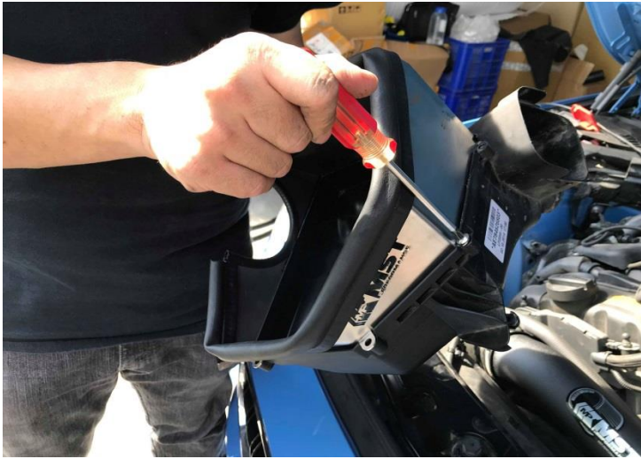
Figure 25: Install the heat shield on the top of air box and secure with bolts.
