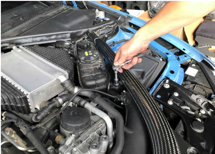
Figure 2: Remove the bolts on the struts bar. Total of 9 bolts.
