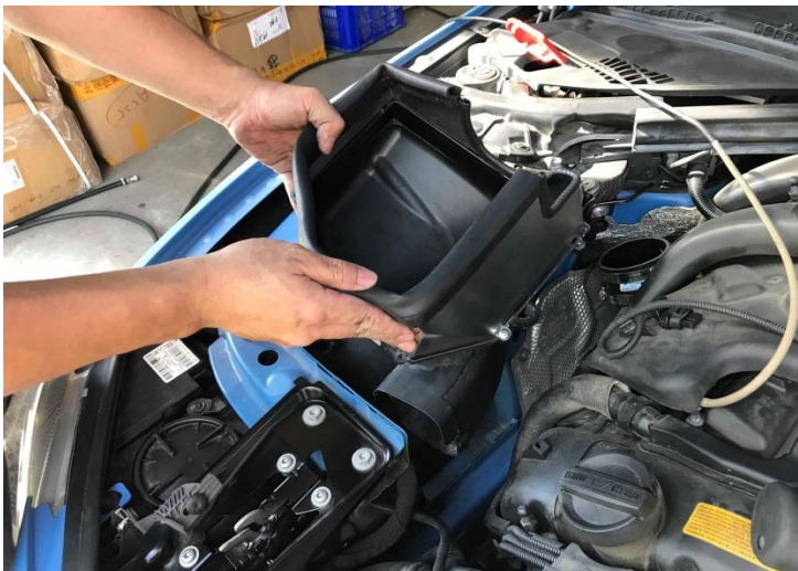
Figure 26: Set the heat shield.
