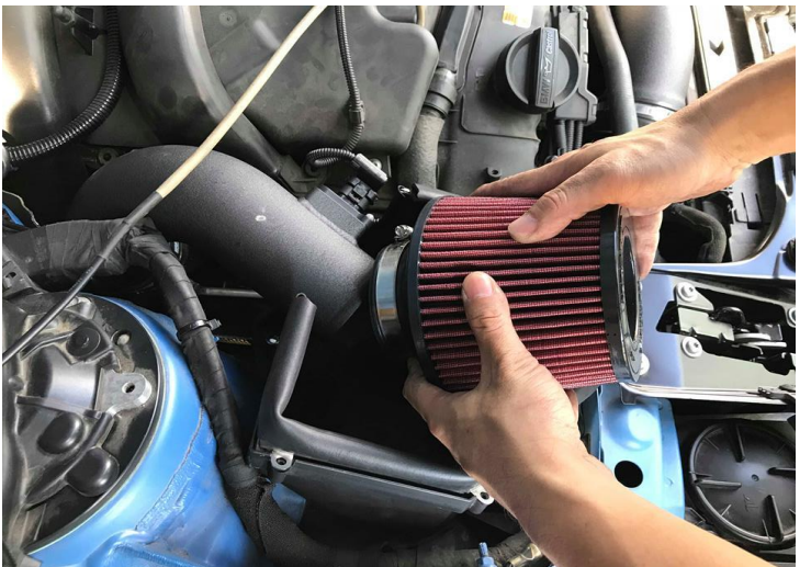
Figure 29: Install the air filter.
