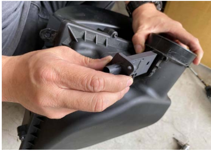
Figure 14: Remove the MAF sensor from the air box(BW-G5401). Remove IAT sensor from the air box(BW-G5301). 從集氣箱中取出 MAF 感應器 (BW-G5401) 從集氣箱中取出 IAT 感應器(BW-G5301)
