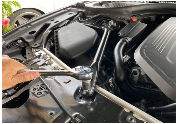
Figure 4: Remove the stock strut bar.拆下原廠支柱桿
