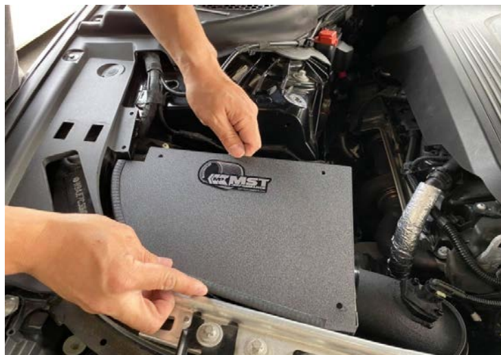
Figure 20: Install the heat shield cover and secure with M4 bolt. 安裝隔熱罩並用 M4 螺栓固定
