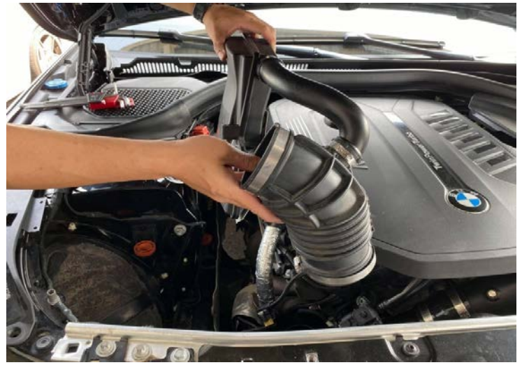
Figure 10: Remove the stock hose and muffler. 拆下原廠軟管和消音器
