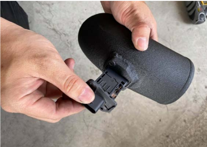
Figure 15: Install the MAF sensor on MST tube(BW-G5401). Install IAT sensor on MST tube(BW-G5301). 將MAF感應器安裝在MST管上(BW-G5401) 將IAT感應器安裝在MST管上(BW-G5301)
