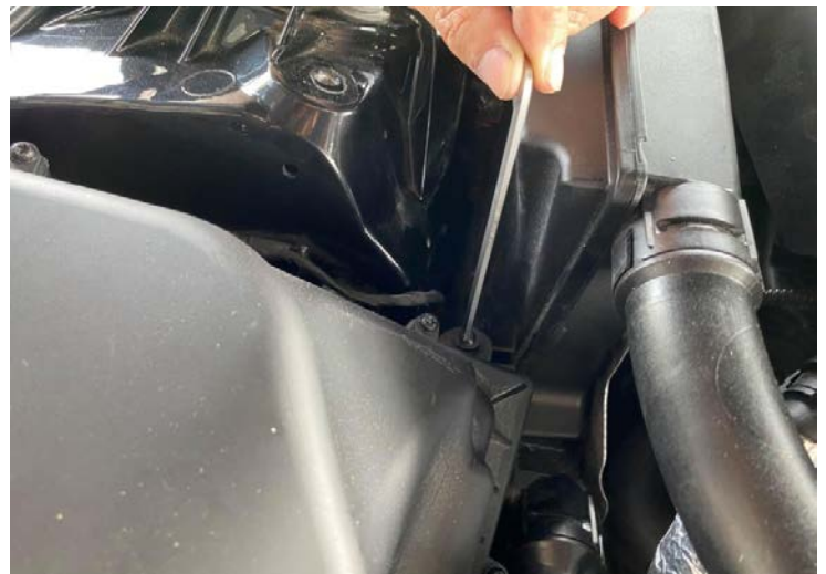
Figure 5: Remove the air box muffler screw. 拆下集氣箱消音器螺絲
