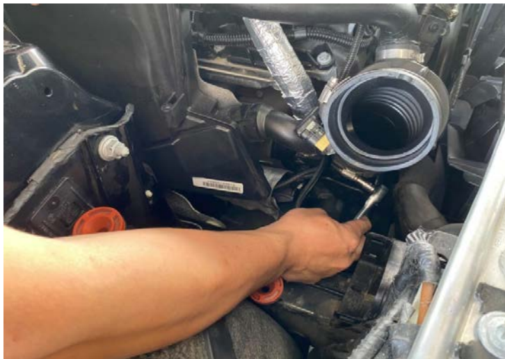
Figure 9: Loosen the stock tube hose clamp. 鬆開原廠管軟管夾
