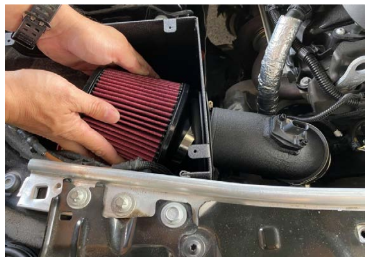
Figure 17: Install the MST tube.安裝 MST 管 (Do not install the tube upside down, or the error code- air mess may occur.) (請勿將管子倒置安裝，否則可能會出現錯誤代碼-空氣混亂。)
