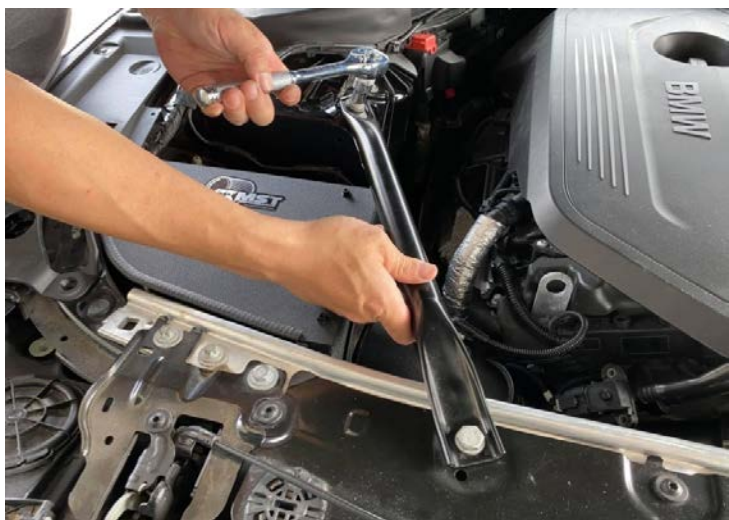
Figure 21: Reinstall the stock strut bar.重新安裝原廠支柱桿
