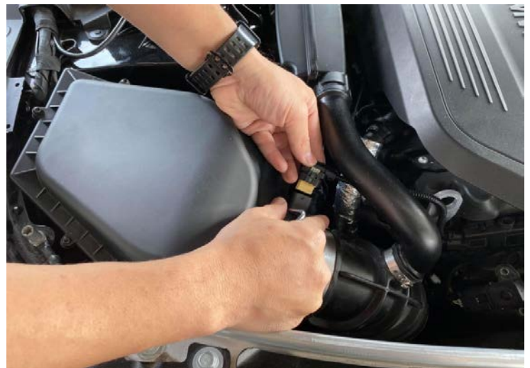
Figure 6: Disconnect the MAF sensor. 斷開MAF感應器的連接
