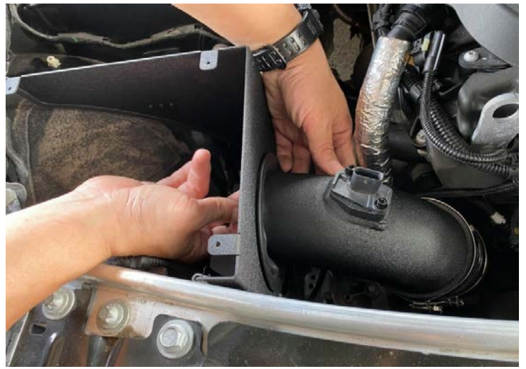
Figure 17: Install the MST tube.安裝 MST 管 (Do not install the tube upside down, or the error code- air mess may occur.) (請勿將管子倒置安裝，否則可能會出現錯誤代碼-空氣混亂。)
