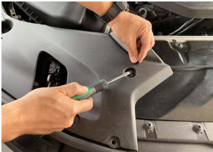
Figure 2: Remove the retainer clip x 3.拆下固定夾 x 3
