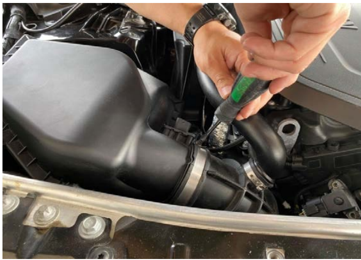
Figure 7: Loosen the stock tube hose clamp. 鬆開原廠管軟管夾
