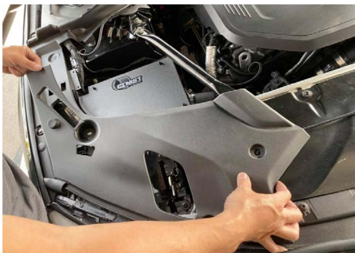
Figure 22: Reinstall the engine compartment protective cover.重新安裝引擎室防護罩
