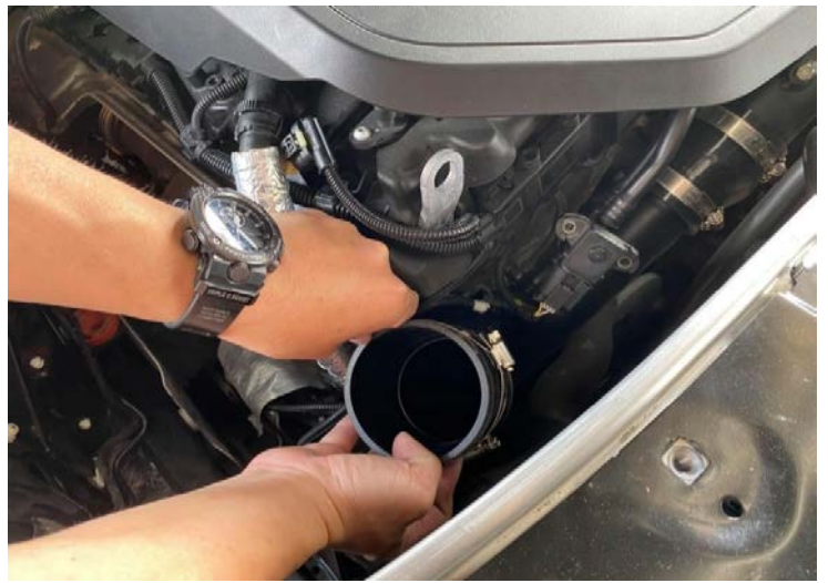
Figure 11: Install the 89-83mm(L76) silicone hose.(BW-G5401) /Install the 89-83mm(L55) silicone hose.(BW-G5301) 安裝89-83mm(L76)矽膠管
