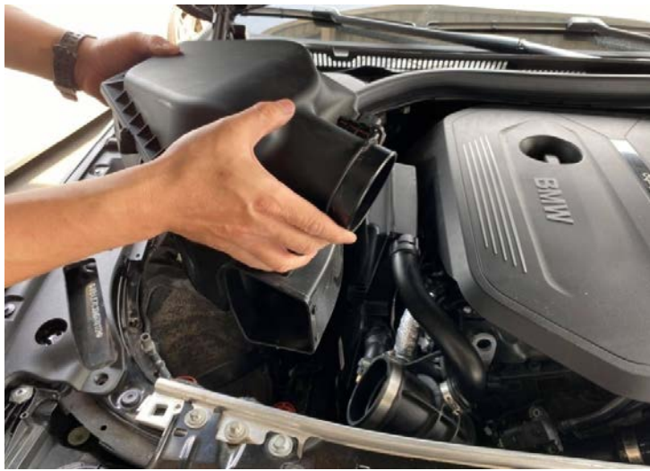
Figure 8: Remove the stock air box. 拆下集氣箱
