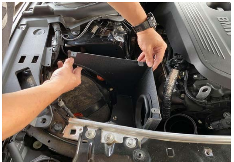
Figure 12: Install the heat shield. 安裝隔熱罩
