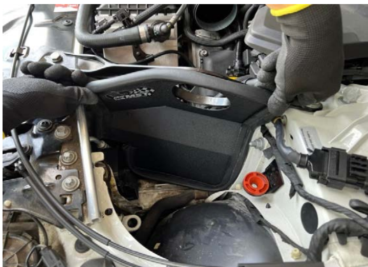
Figure 9: Install the heatshield x 2.安裝隔熱罩 x 2
