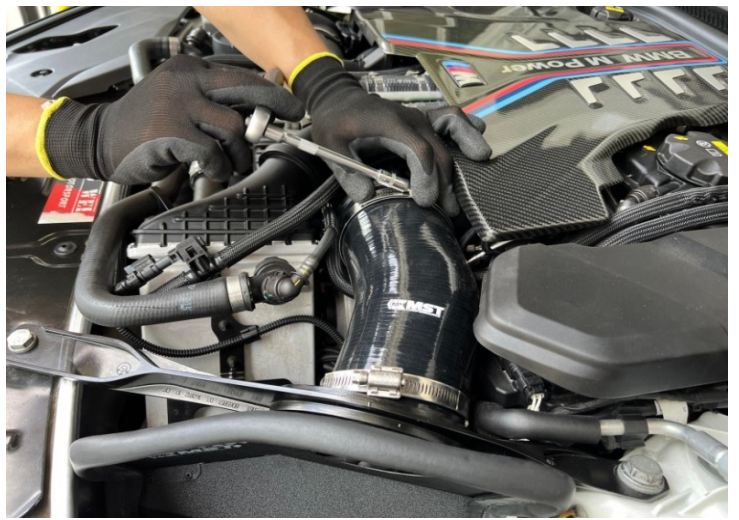
Figure 11: Tight the clamps.擰緊夾子
