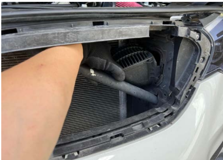
Figure 16: Remove the stock air scoop. 拆下原廠空氣勺
