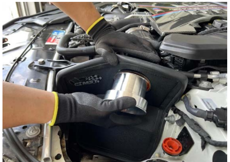
Figure 12: Install the MST adapter x 2. (can use some oil) 安裝 MST 轉接器 x 2。(可用點油)
