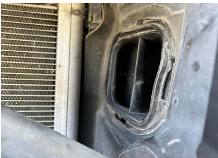
Figure 16: Remove the stock air scoop. 拆下原廠空氣勺
