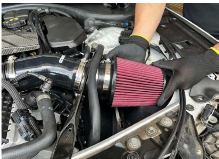
Figure 14: Install the MST filter.安裝MST高流量濾芯
