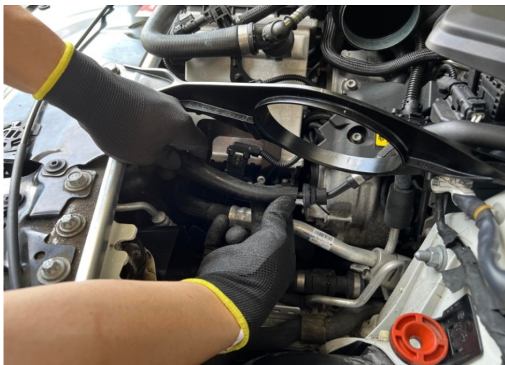
Figure 8: Use foam pipe to protect hot water tube. 使用泡沫管保護熱水管
