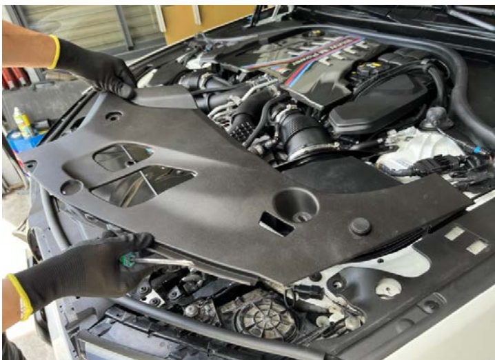
Figure 2: Remove the engine compartment protective cover.拆下引擎室防護罩
