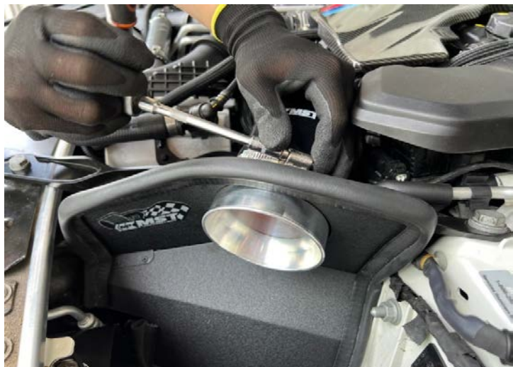
Figure 13: Tight the clamps.擰緊夾子
