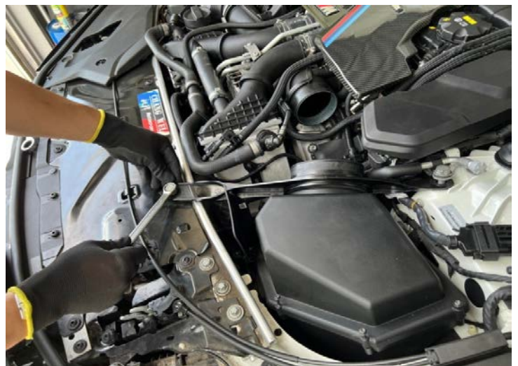
Figure 5: Remove the stock strut bar. 拆下庫存支柱桿
