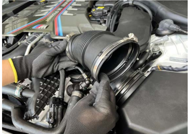
Figure 4: Remove the wire clips.拆下線夾
