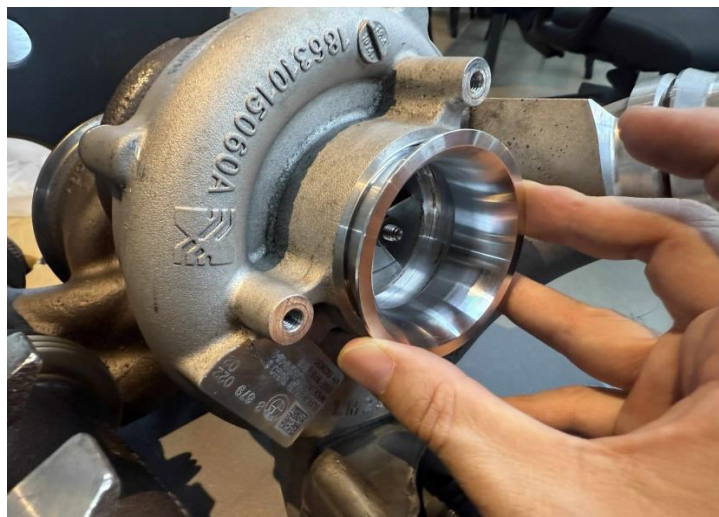
Figure 5: For stock turbo, please install velocity adapter. Hybrid turbo does not need to install it. (Velocity adapter need to install o-ring) 驟5: 原廠渦輪請安裝渦輪口墊片, 加大渦輪不需要安裝
