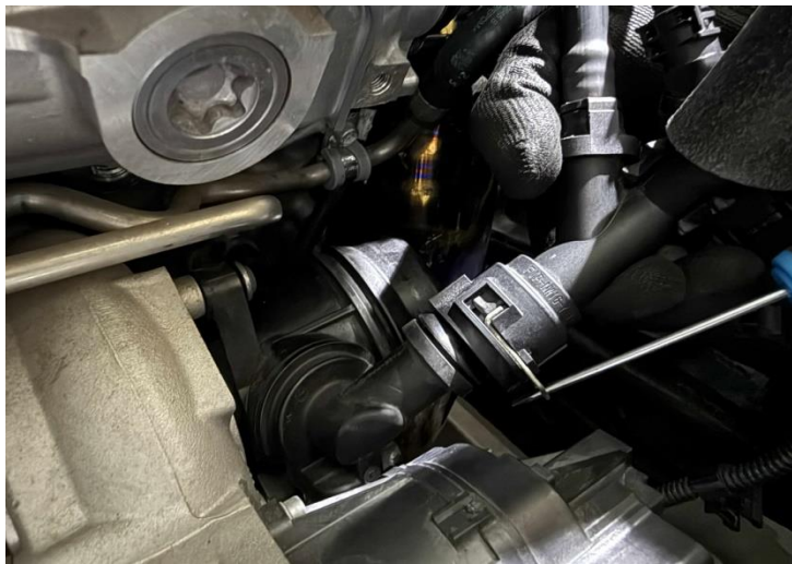
Figure 1: Stock turbo inlet. Remove the PCV plug. 驟1: 移除PCV接頭
