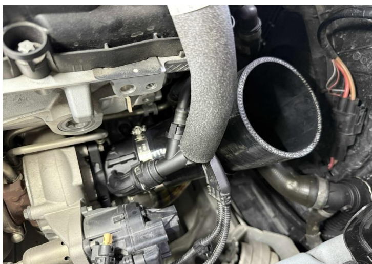
Figure 9: Please note that the PCV heater is removed when installing this intake system, which will result in a stored error code. While this typically does not illuminate the check engine light, certain vehicle models may display a check engine light depending on their system sensitivity.
