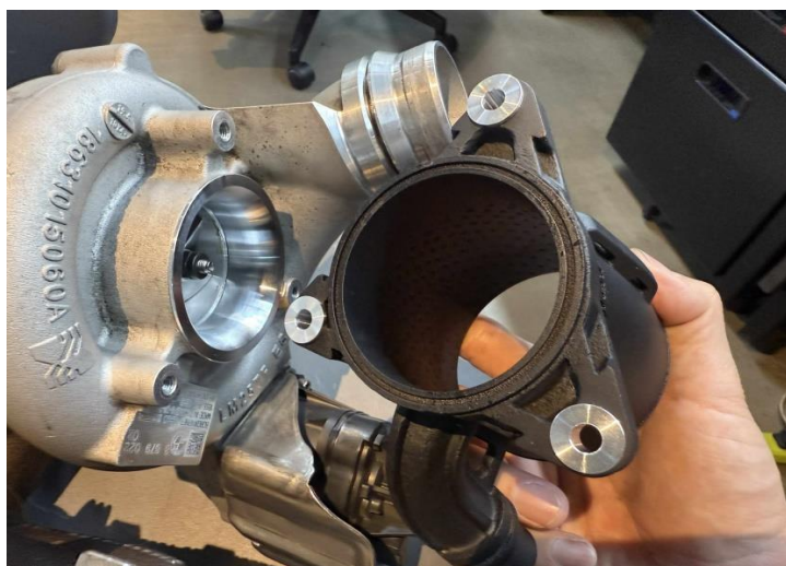
Figure 6: If installed a velocity adapter, please install a spacer above the inlet. If not, it is not necessary. (Turbo inlet need to install o-ring) 步驟6: 如有安裝渦輪口墊片, 請在增流管底座安裝墊片, 注意安裝方向, 如加大渦輪無安裝渦輪口墊片則無須安裝
