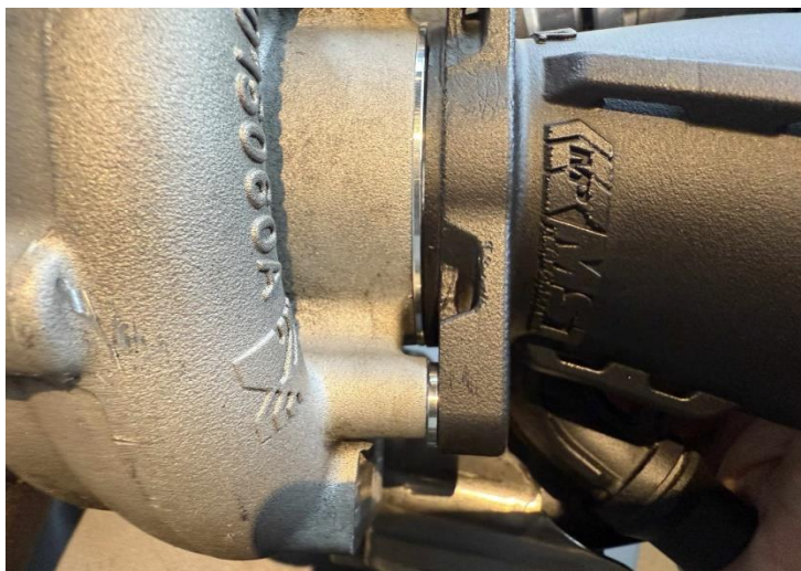
Figure 7: Stock turbo connected to MST turbo inlet. 步驟7: 渦輪口墊片和增流管結合示意圖
