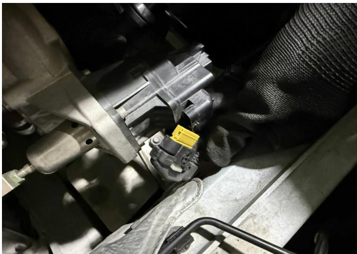
Figure 2: Disconnect the wastegate plug. 驟2: 斷開wastegate接頭
