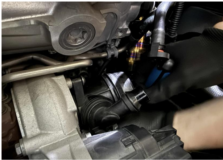
Figure 4: Loosen the bolts on the stock inlet and remove the inlet. 驟4: 鬆開原廠渦輪進氣管螺絲 取下進氣管
