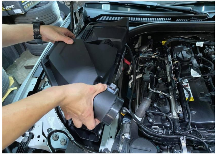
Figure 4: Remove stock air box.拆下原廠集氣箱
