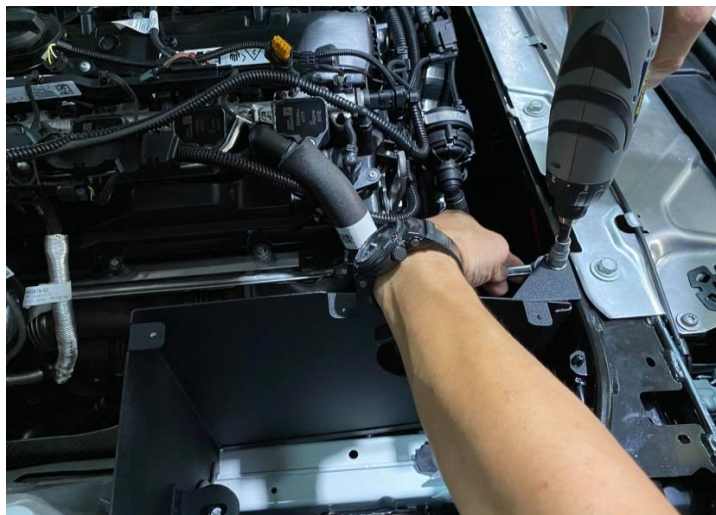
Figure 10: Secure the heat shield breaket with M6 bolt. 用 M6 螺栓固定隔熱罩支架
