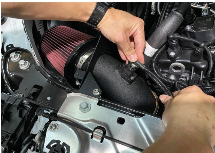
Figure 14: Plug in the mass air flow sensor connector. 插入空氣流量感應器連接器
