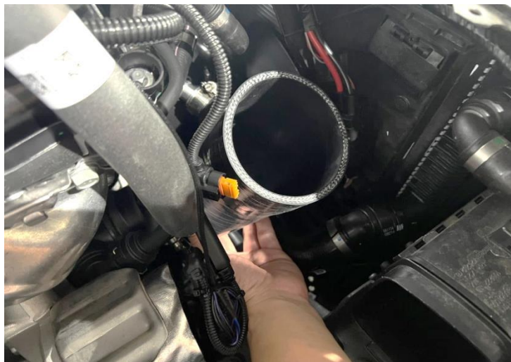
Figure 7: Install the MST silicone hose and connect PCV. 安裝MST矽膠管並連接PCV
