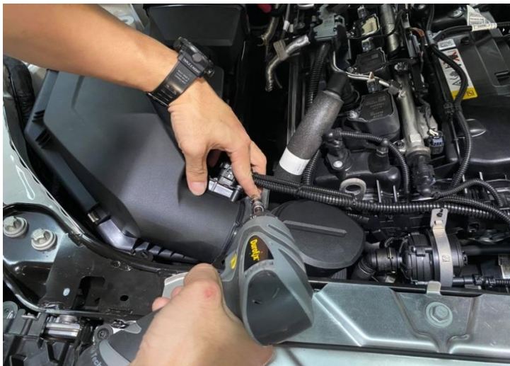
Figure 2: Loosen the stock tube hose clamp. 鬆開原廠管軟管夾
