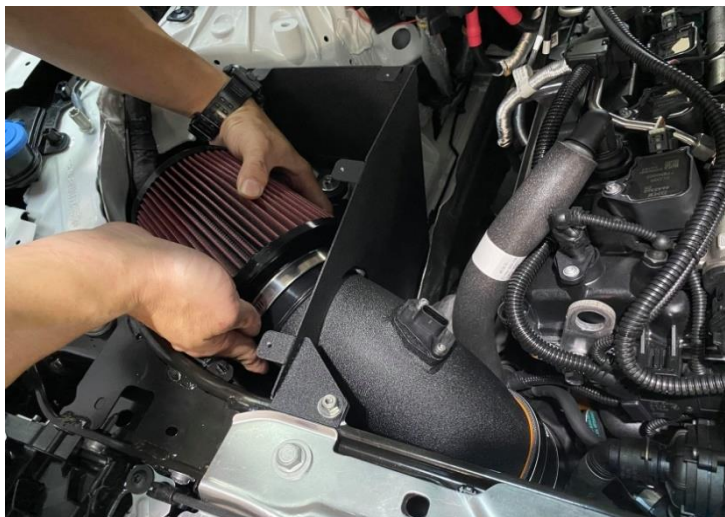
Figure 13: Install the air filter.安裝高流量濾芯
