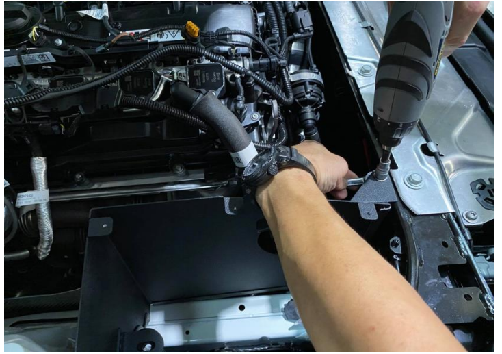
Figure 10: Secure the heat shield bracket with M6 bolt.
