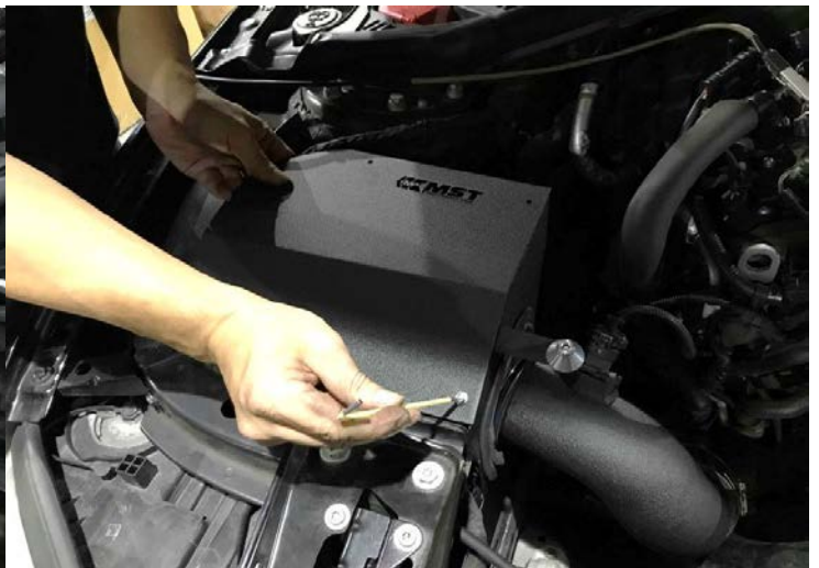
Figure 17: Secure with bolt.用螺栓固定
