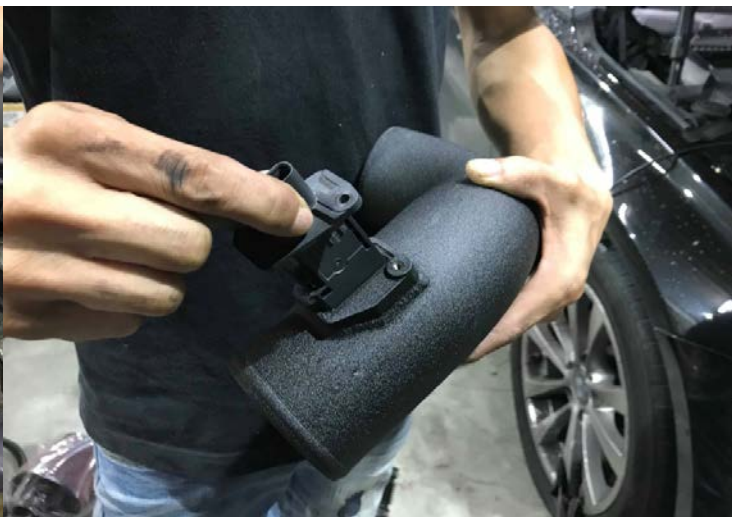
Figure 10: Install mass air sensor into the mst intake tube. 將空氣品質感測器安裝到 mst 進氣管中
