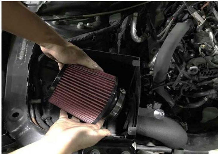
Figure 13: Install air filter.安裝空氣過濾器
