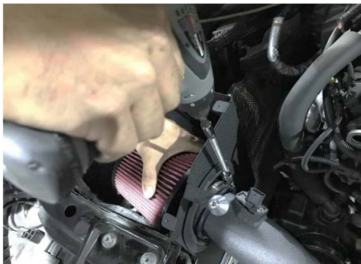
Figure 14: Tighten the hose clamp. 擰緊軟管夾
