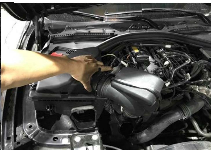
Figure 4: Remove stock air box. 拆下集氣箱
