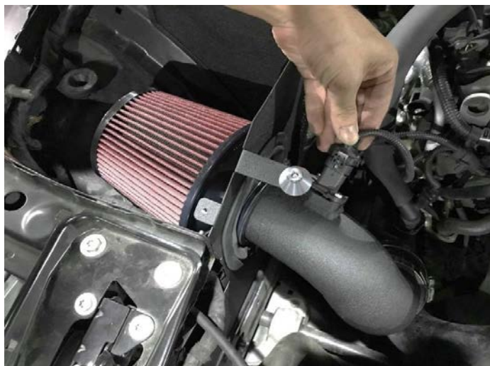
Figure 15: Plug in the mass air flow sensor connector.插入空氣流量感測器連接器
