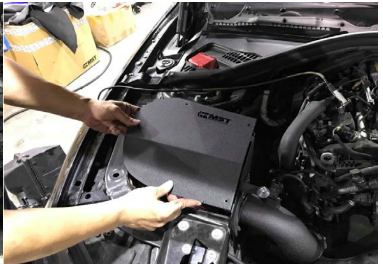
Figure 16: Install heat shield cover.安裝隔熱罩
