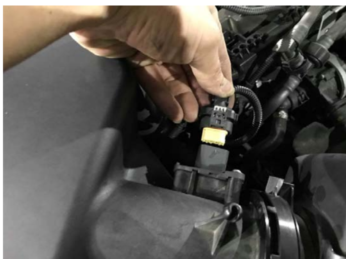
Figure 2: Disconnect the mass air sensor. 斷開空氣品質感應器
