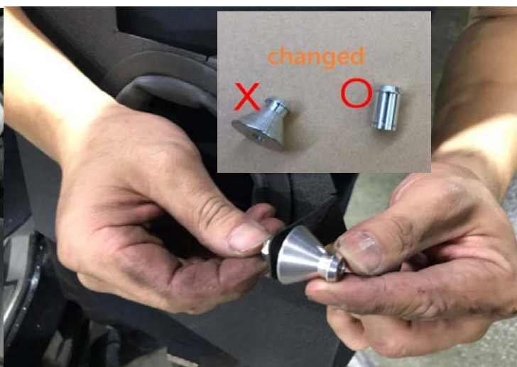
Figure 5: Install the heat shield mount. 安裝隔熱罩安裝座
