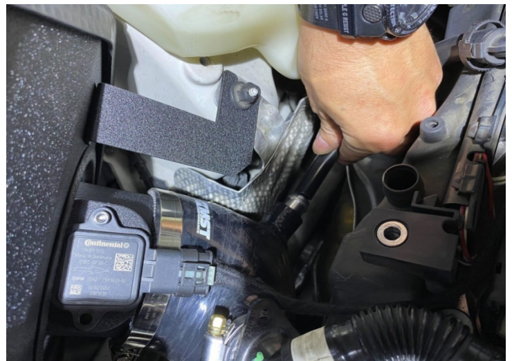
Figure 24: Reinstall the PCV.重新安裝 PCV
