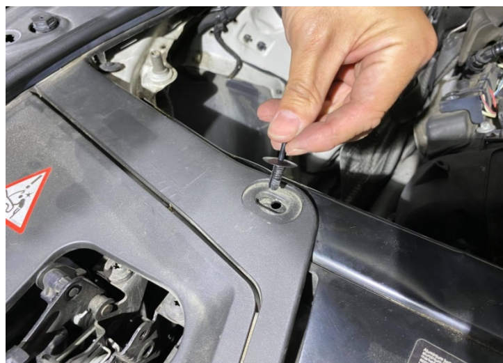
Figure 18: Remove the retainer clip.取下固定夾
