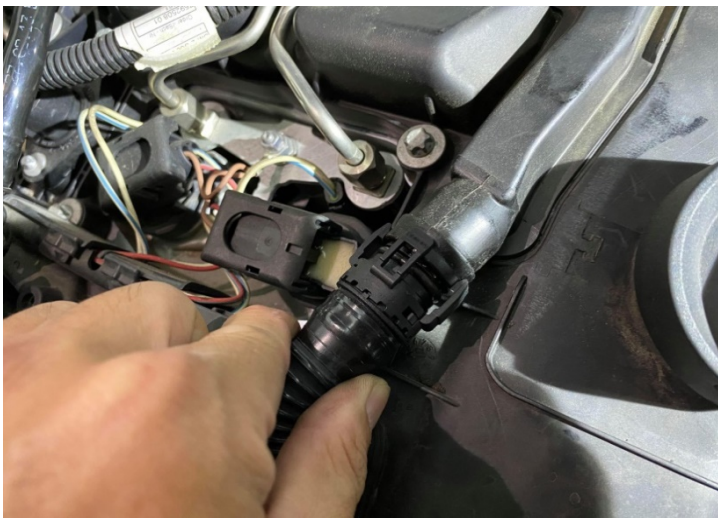
Figure 8: Remove the PCV. 移除 PCV
