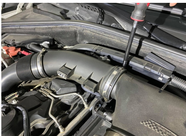
Figure 2: Loosen the stock tube hose clamp. 鬆開原廠管軟管夾
