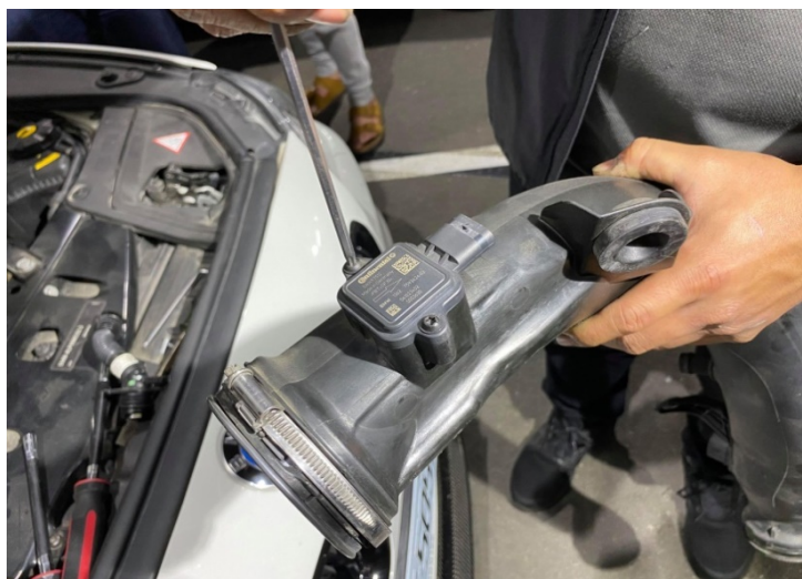
Figure 13: Remove the MAF sensor from the stock intake pipe.從進氣管拆下 MAF 感應器
