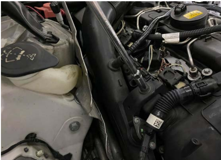
Figure 9: Remove the M6 bolt. 拆下M6螺栓
