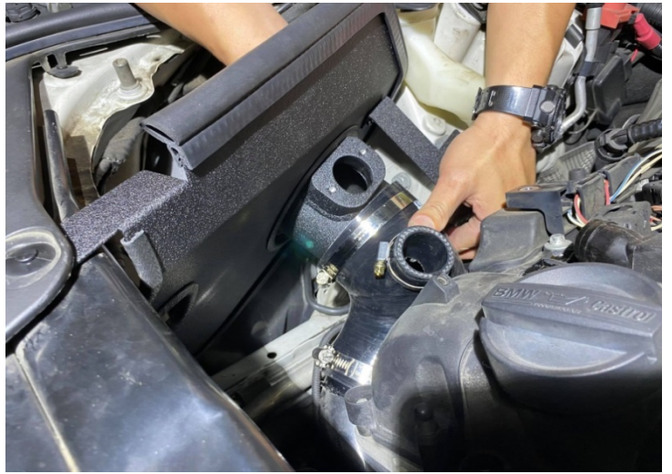
Figure 22: Install the silicone hose and tube. 安裝矽膠軟管和管子
