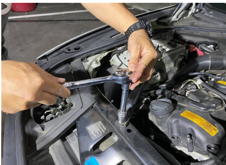
Figure 5: Remove the strut bar.拆下支柱桿
