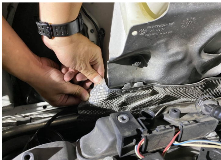
Figure 16: Bend the heat insulation plate.將隔熱板折彎
