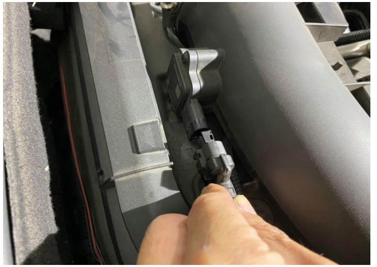
Figure 10: Unclip the sensor. 鬆開感應器
