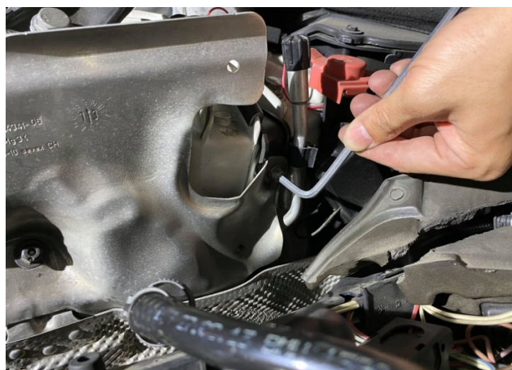
Figure 14: Remove the heat shield's bolt.拆下隔熱罩的螺栓
