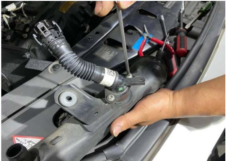
Figure 12: Remove the PCV from the stock intake pipe. 從原廠進氣管拆下 PCV
