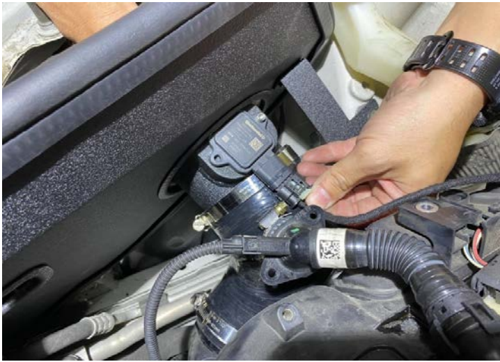
Figure 26: Connect the mass air sensor. 連接空氣品質感測器
