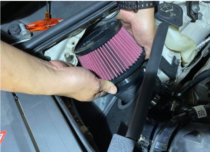
Figure 27: Install the MST air filter.安裝 MST 空氣濾芯
