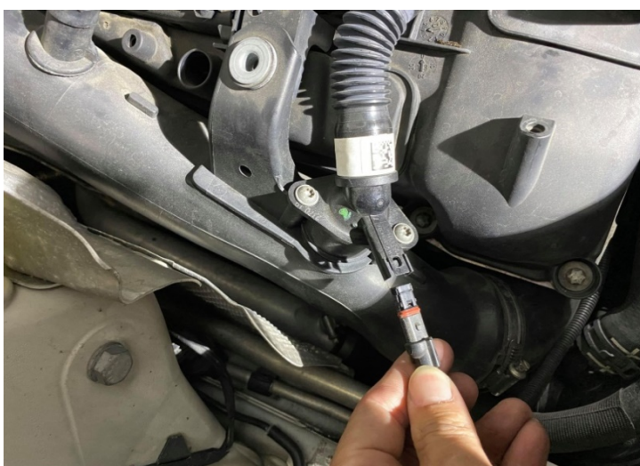
Figure 6: Remove the PCV clip.拆下PCV 夾
