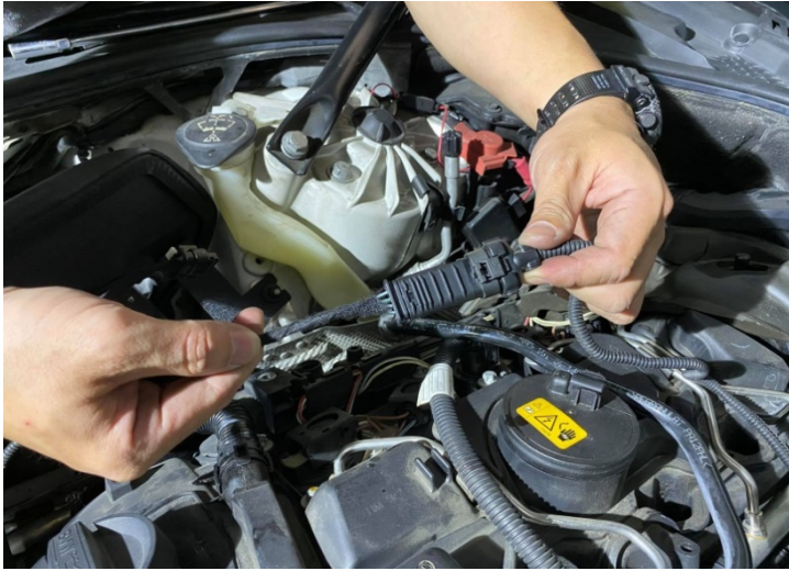
Figure 25: Electrical extensions to plug them back in to the factory wiring harness. 用於將它們插回工廠線束的電氣擴充件
