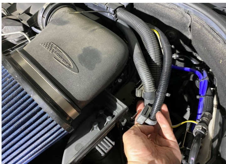
Figure 3: Remove the rubber that fixes the cords. 取下固定電線的橡膠
