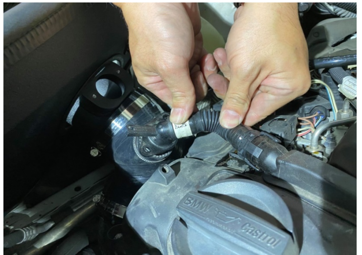
Figure 23: Reinstall the PCV.重新安裝 PCV
