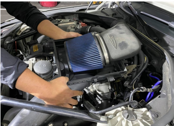
Figure 4: Remove the air box.拆下原廠集氣箱
