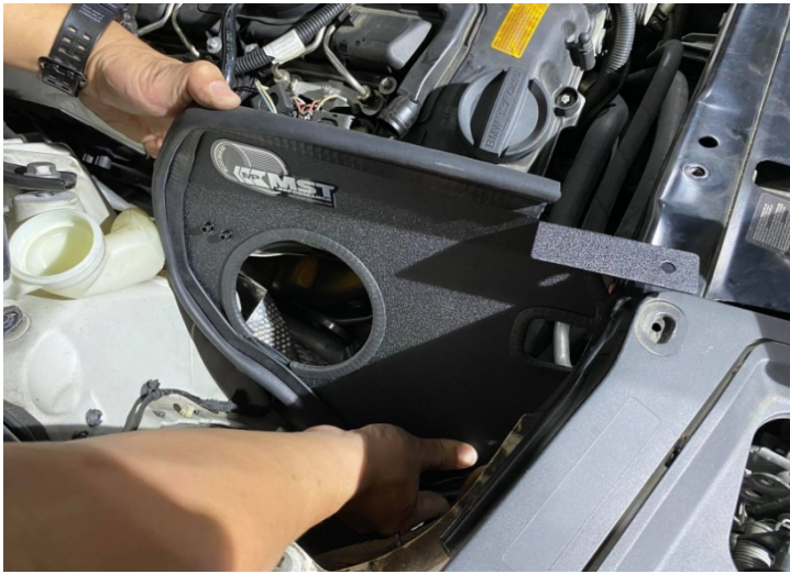
Figure 19: Install the heat shield.安裝隔熱罩
