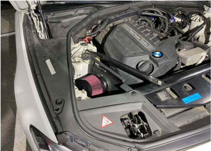
Figure 28: Congratulations! You have just completed the installation of this intake system. Periodically, check the alignment of the intake, normal wear and tear can cause nuts and bolts to come loose. 恭喜！您剛剛完成了此進氣系統的安裝。定期檢查進氣口的對準情況，正常磨損會導致螺帽和螺栓鬆動
