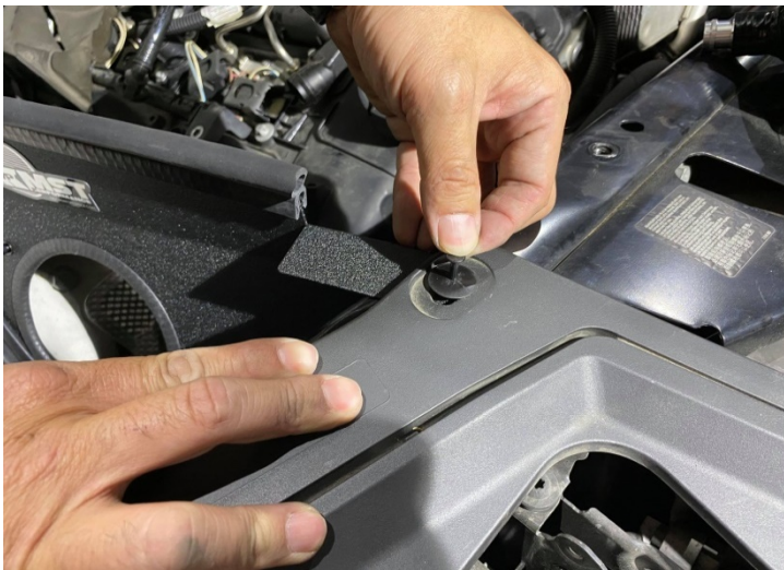
Figure 20: Install the retainer clip.安裝固定夾
