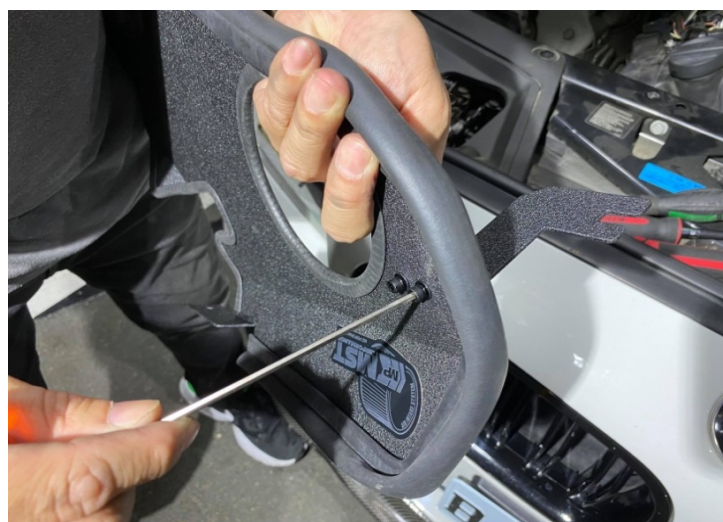
Figure 17: Install the bracket.安裝支架
