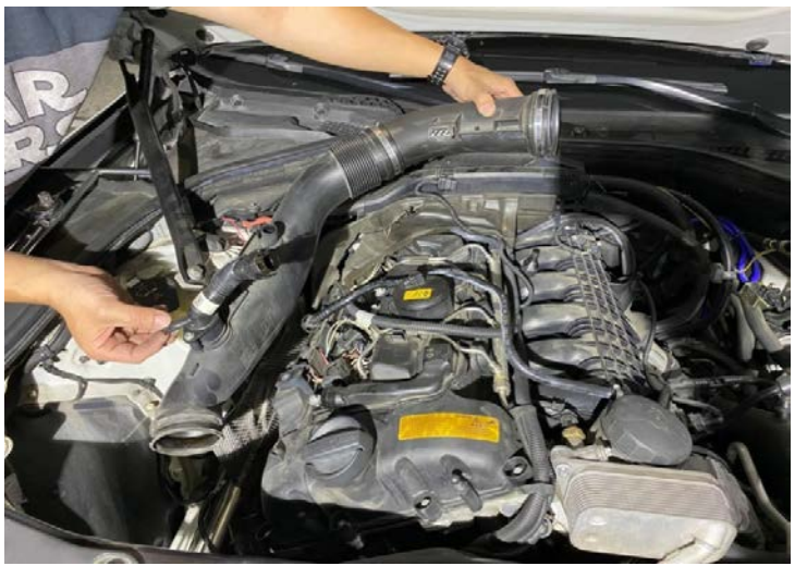
Figure 11: Remove the stock tube. 拆下原廠管
