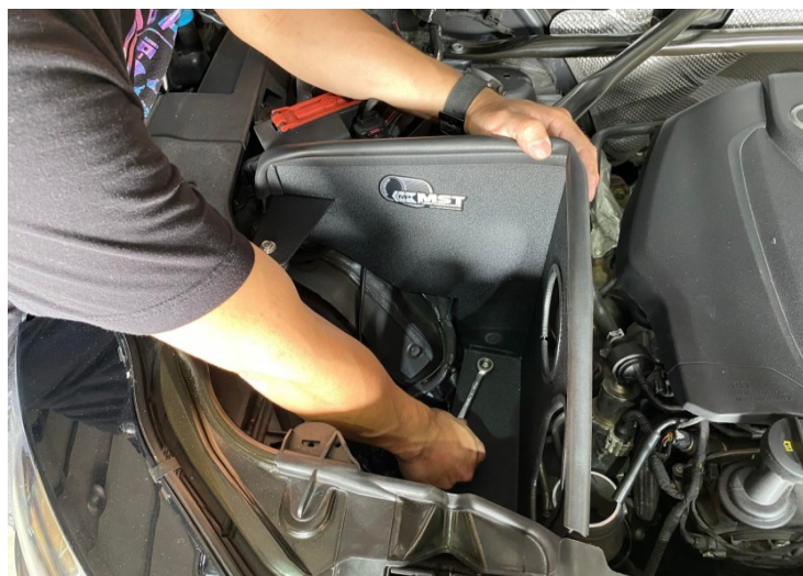
Figure 11: Secure the heat shield with M6 bolt. 用 M6 螺栓固定隔熱罩
