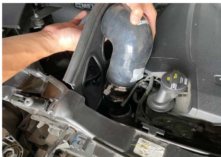
Figure 12: Install the MST silicone hose. 安裝MST矽膠軟管
