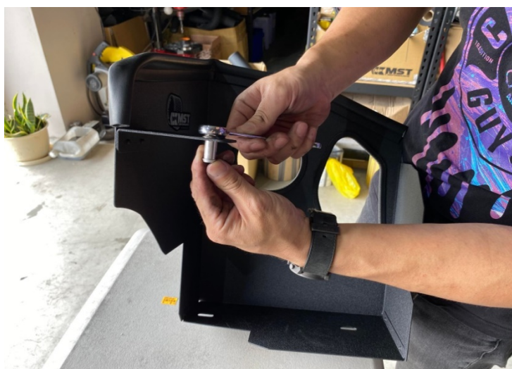
Figure 8: Install the aluminum mount on heatshield. 將鋁製支架安裝到隔熱罩上
