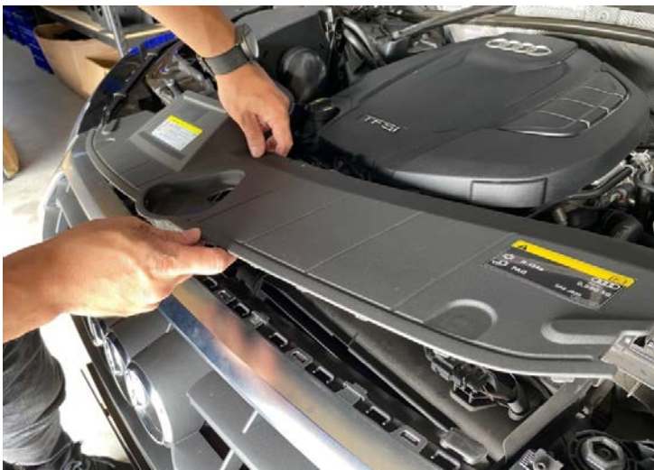
Figure 3: Remove the engine compartment protective cover. 拆下引擎室防護罩
