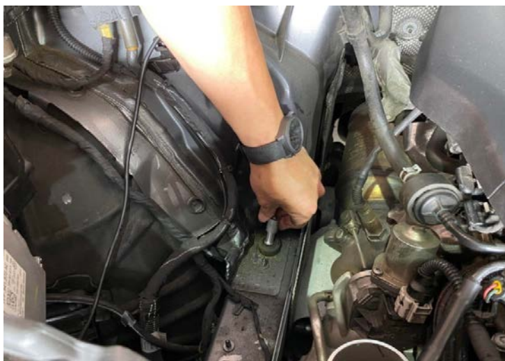
Figure 9: Install the aluminum mount on rubber. 將鋁製安裝座安裝在橡膠上
