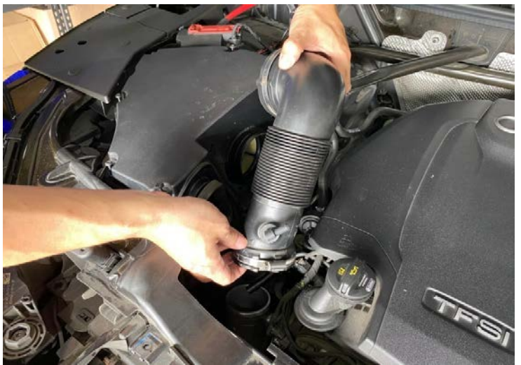
Figure 6: Remove the stock hose. 拆下原廠軟管
