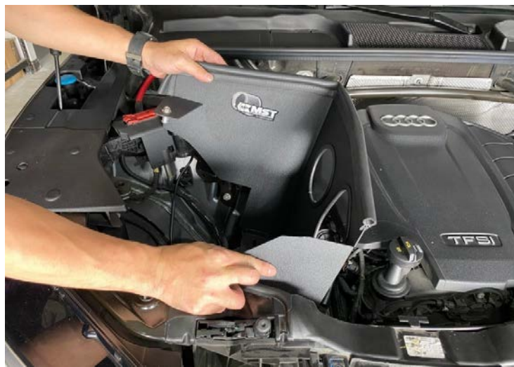
Figure 10: Install the MST heatshield. 安裝 MST 隔熱罩
