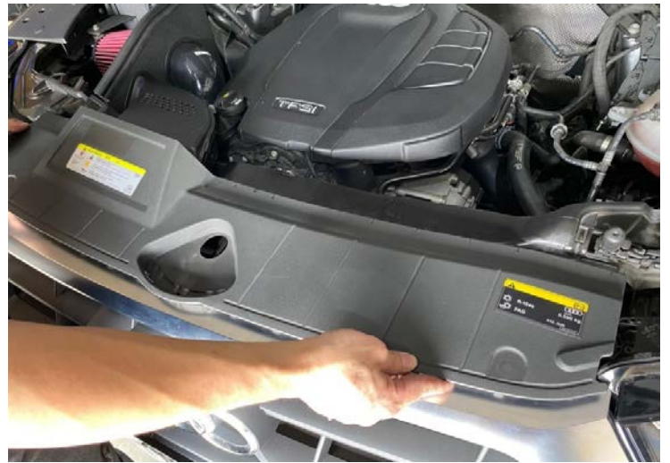
Figure 16: Reinstall the engine compartment protective cover.重新安裝引擎室防護罩
