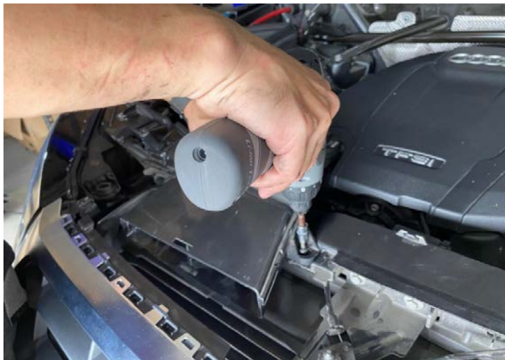
Figure 15: Reinstall the stock air scoop and secure the bolt. 重新安裝原廠進氣口並固定螺栓
