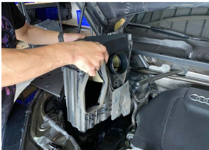
Figure 7: Remove the stock air box. 拆下原廠空氣箱
