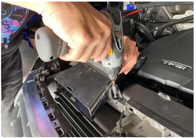
Figure 4: Remove the air scoop bolts. 拆下進氣口螺栓
