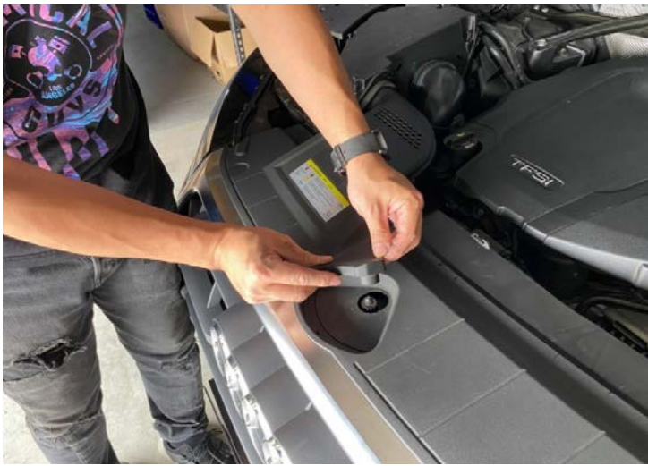
Figure 2: Remove the lever. 拆下控制桿
