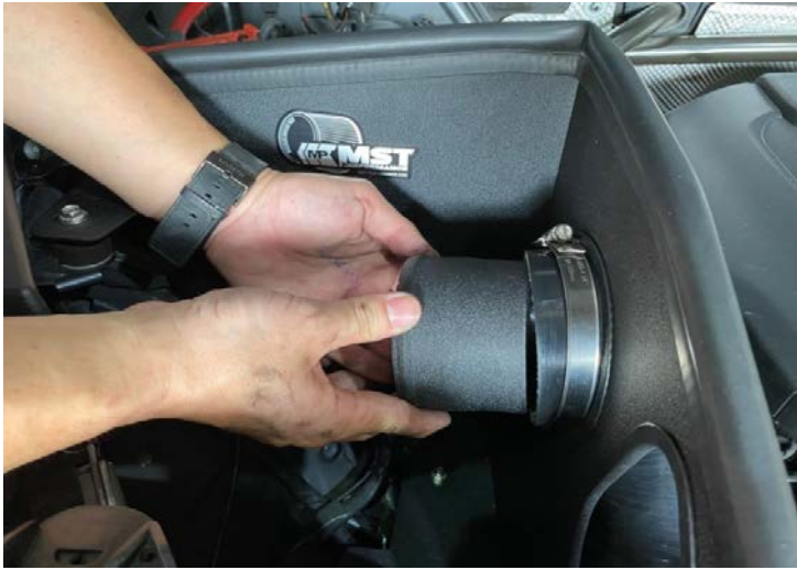
Figure 13: Install the 80-89 tube.安裝80-89鋁管
