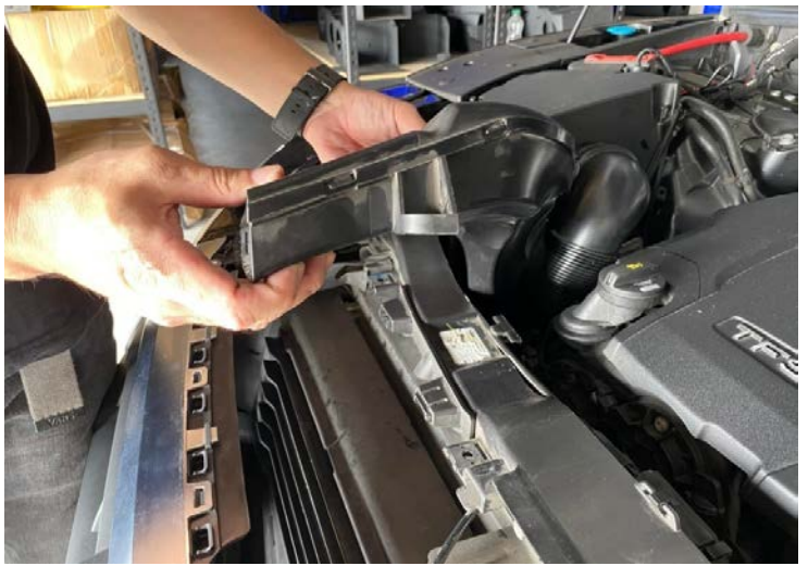
Figure 5: Remove the air scoop. 拆下導風罩
