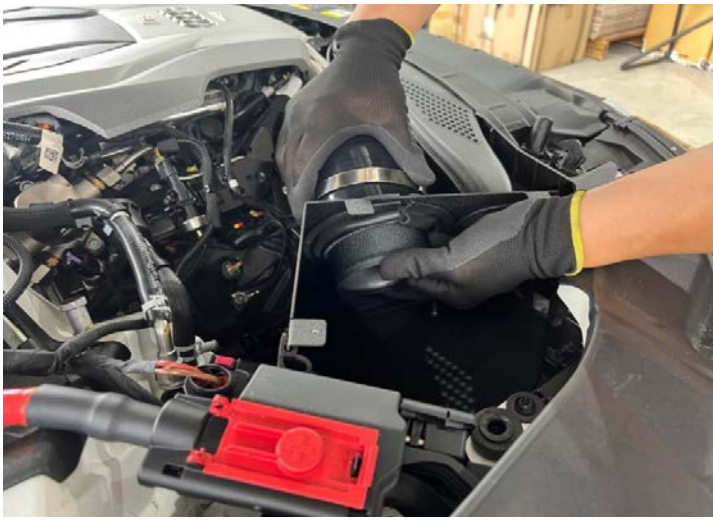
Figure 7: Install the MST tube.安裝MST鋁管
