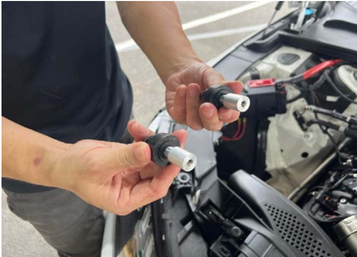
Figure 2: Remove the rubber from the stock air box and install the ALU mount on rubber. 從原廠集氣箱中取出橡膠並將 ALU 安裝座安裝在橡膠上
