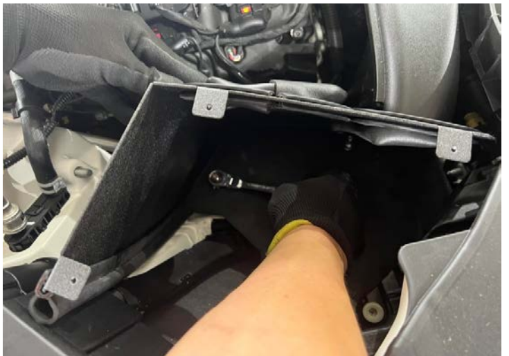
Figure 5: Secure with bolt.用螺栓固定
