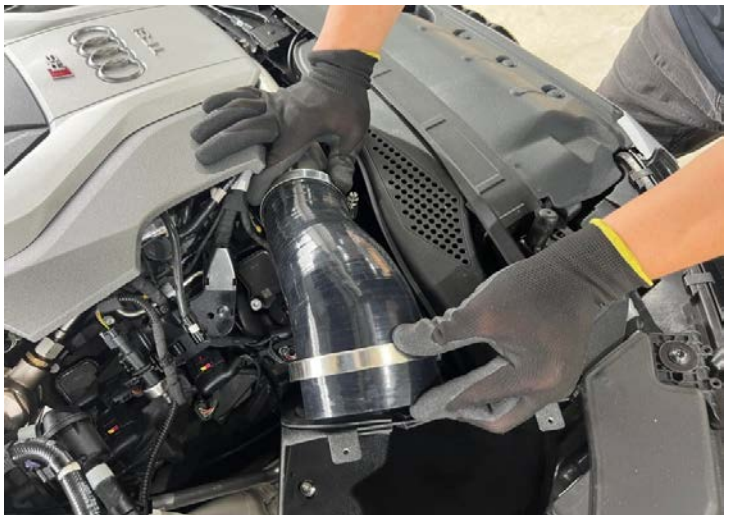
Figure 6: Install the MST silicone hose. 安裝MST矽膠軟管
