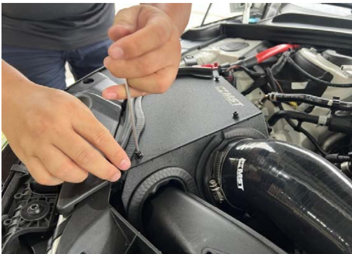
Figure 9: Install the heat shield cover and secure with bolt.安裝隔熱罩並用螺栓固定
