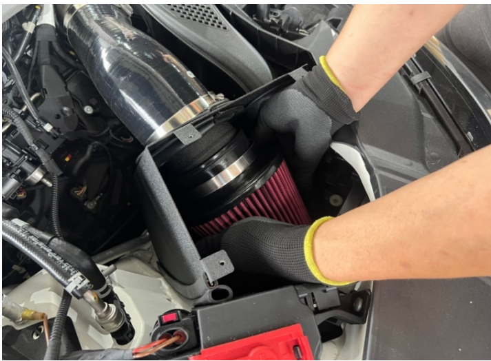
Figure 8: Install the air filter.安裝空氣過濾器
