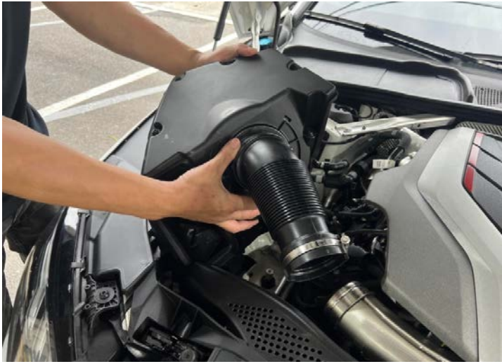
Figure 1: Loosen the hose clamp and remove the air box. 鬆開軟管夾並拆下原廠集氣箱。
