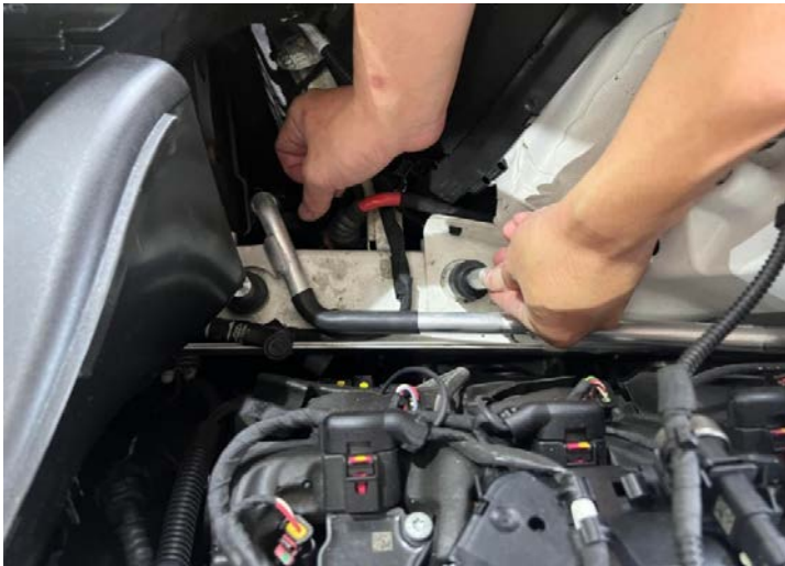
Figure 3: Install the ALU mount and rubber. 安裝 ALU 安裝座和橡膠
