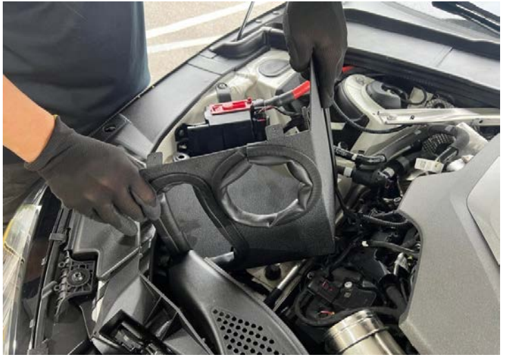
Figure 4: Install the heat shield.安裝隔熱罩
