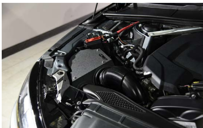
Figure 9: Congratulations! You have just completed the installation of this intake system. Periodically, check the alignment of the intake, normal wear and tear can cause nuts and bolts to come loose.
