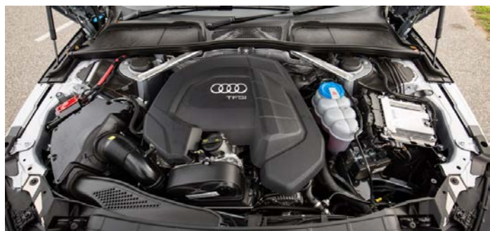
Figure 1: Loosen the hose clamp and remove the air box. 鬆開軟管夾並拆下集氣箱
