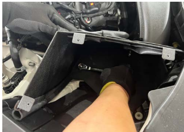
Figure 5: Secure with bolt. 用螺栓固定
