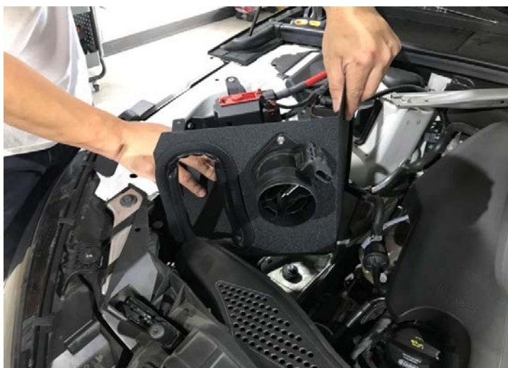
Figure 9: Install the heat shield.安裝隔熱罩
