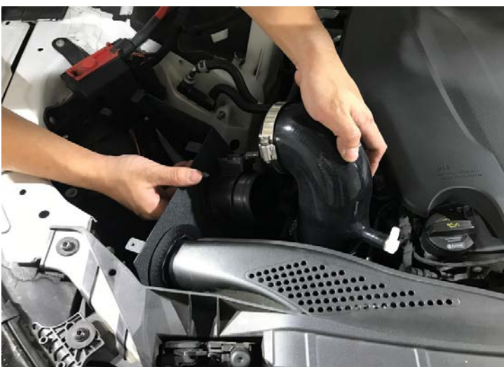
Figure 11: Install the MST silicone tube.安裝MST矽膠管
