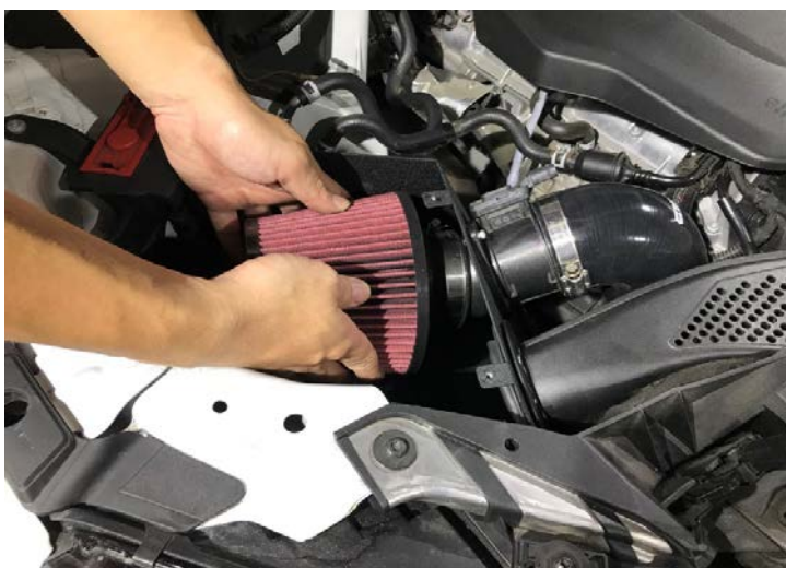
Figure 12: Install the air filter.安裝空氣過濾器
