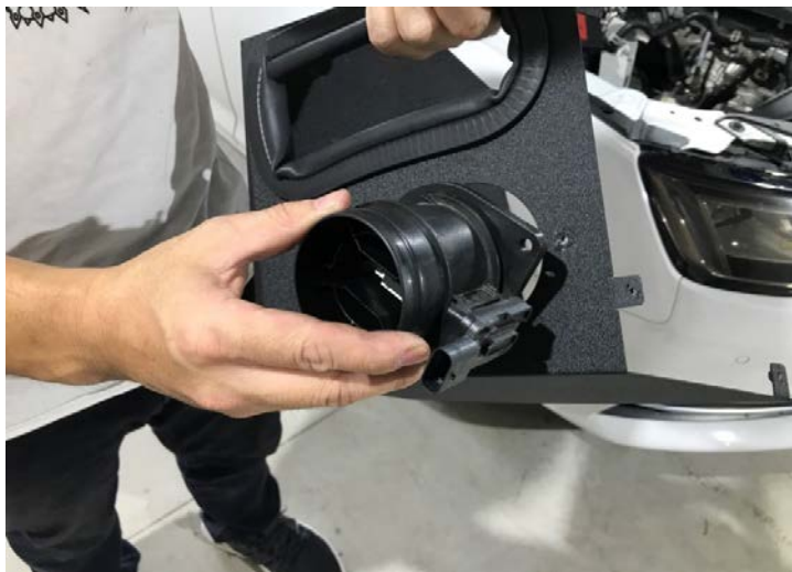
Figure 7: Install MAF sensor on the heat shield. 將 MAF 感知器安裝在隔熱罩上
