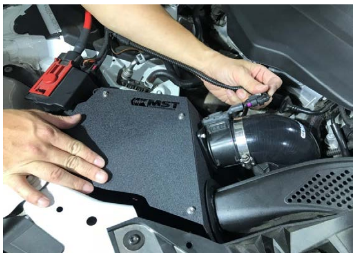
Figure 14: Connect the MAF sensor.連接MAF感測器
