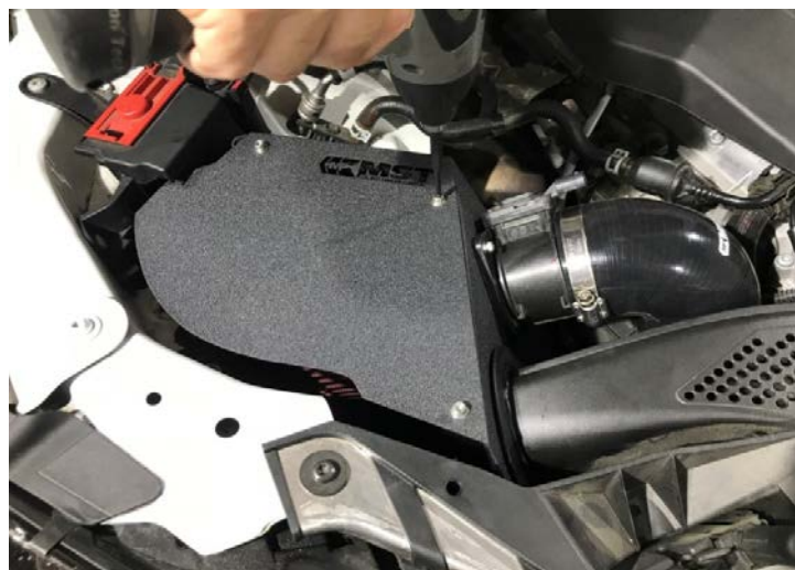
Figure 13: Install the heat shield cover.安裝隔熱罩
