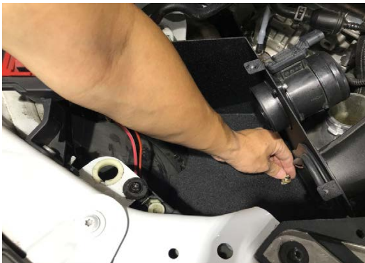
Figure 9: Secure with bolt.用螺栓固定
