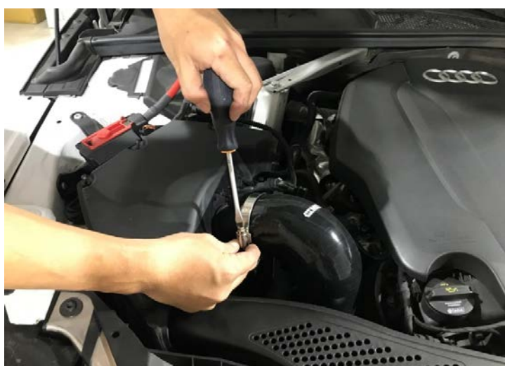
Figure 3: Loosen hose clamp from the factory tube. 從原廠管上鬆開軟管夾
