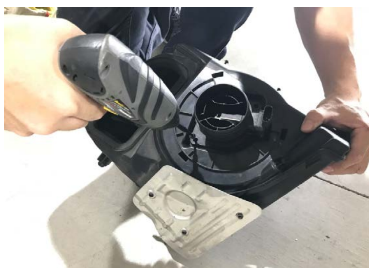
Figure 6: Remove the MAF sensor from the factory airbox. 從原廠集氣箱中取出 MAF 感知器
