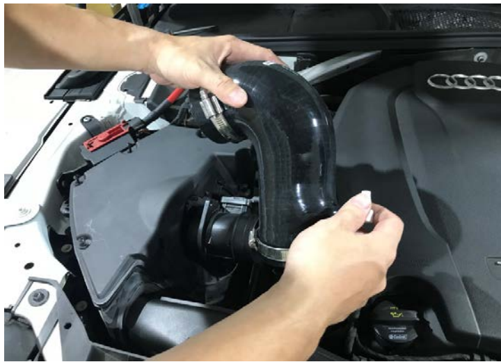
Figure 4: Remove the factory tube. 拆掉原廠管
