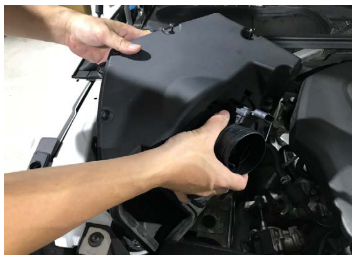
Figure 5: Remove the factory airbox. 拆下原廠集氣箱
