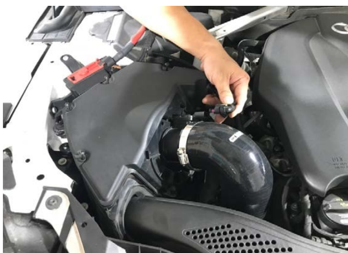
Figure 2: Unclip the sensor. 鬆開感應器
