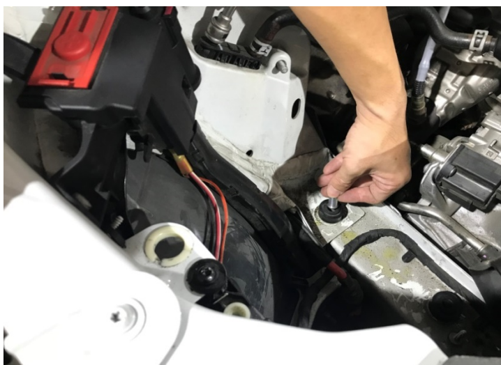
Figure 8: Install the heat shield mount(*2) in the rubber. 將隔熱罩安裝座 (*2) 安裝在橡膠中
