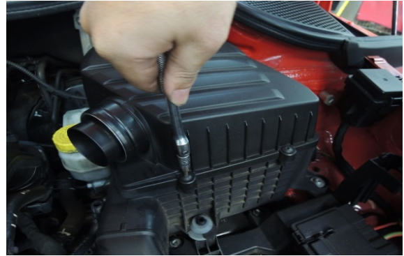
Figure 4 . Remove the bolts from the air box lid and put them aside for install later. 從空氣箱蓋上拆下螺栓，並將其放在一邊以備後用
