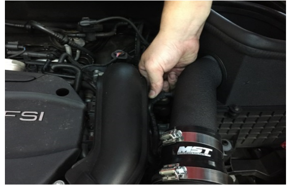
Figure 12. Refit the electrical plug that has been removed from step 3.
