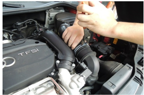
Figure 2. Loosen the clamps to unclip and remove the intake hose from the air box lid 鬆開夾子以鬆開並從空氣箱蓋上取下進氣軟管
