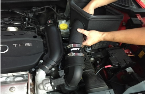
Figure 11. Slide two clamps to each side of the silicone hose, joint the silicone hose and aluminum piece. Tighten the clamps later.
