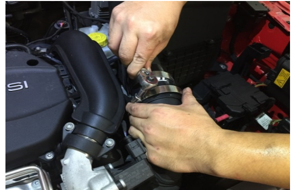
Figure 14. Tighten the clamps (see figure 11) to secure. (Do not overtighten)
