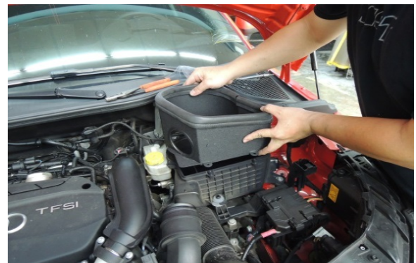
Figure 6 . Install the MST heatshield lining up the grommets with the holes on the base 安裝 MST 隔熱罩，使索環與底座上的孔對齊
