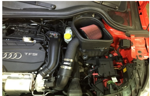
Figure 16: Congratulations! It's all set. Periodically, check the alignment of the intake, normal wear and tear can cause nuts and bolts to come loose.
