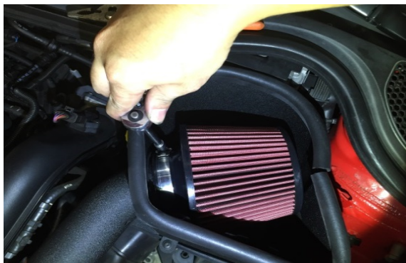
Figure 15. Tighten the clamp to secure the air filter. (Do not overtighten)
