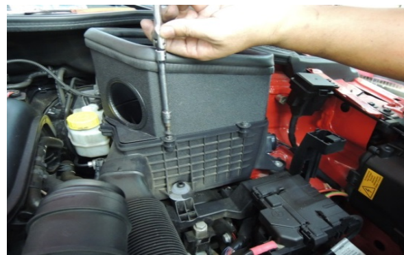
Figure 8. Secure the heat shield with bolts. 用螺栓固定隔熱罩
