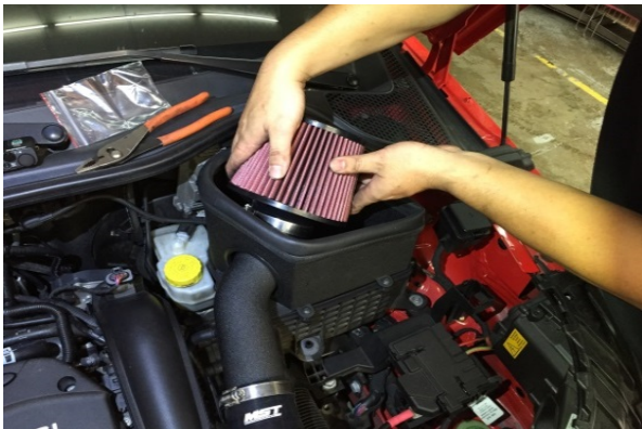
Figure 13. Slide the clamp to MST air filter then insert to the heat shield.
