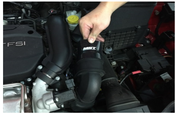
Figure 10. Install the silicone hose.
