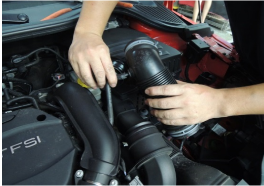
Figure 3. Unclip and remove the electrical plug from the hose 從軟管上鬆開並取下電插頭
