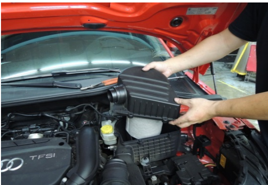
Figure 5. Remove the air box lid from the vehicle.從車輛上拆下空氣箱蓋
