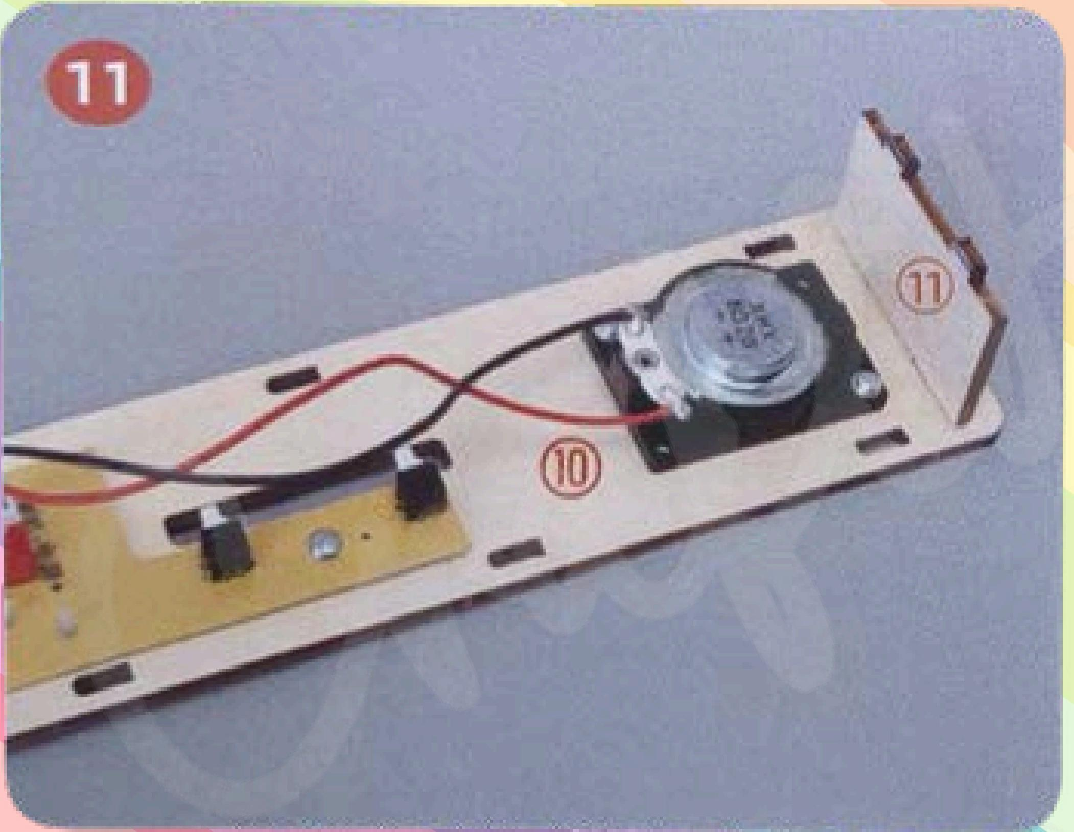
As shown in the picture, insert board No. 11 into board No. 10.
