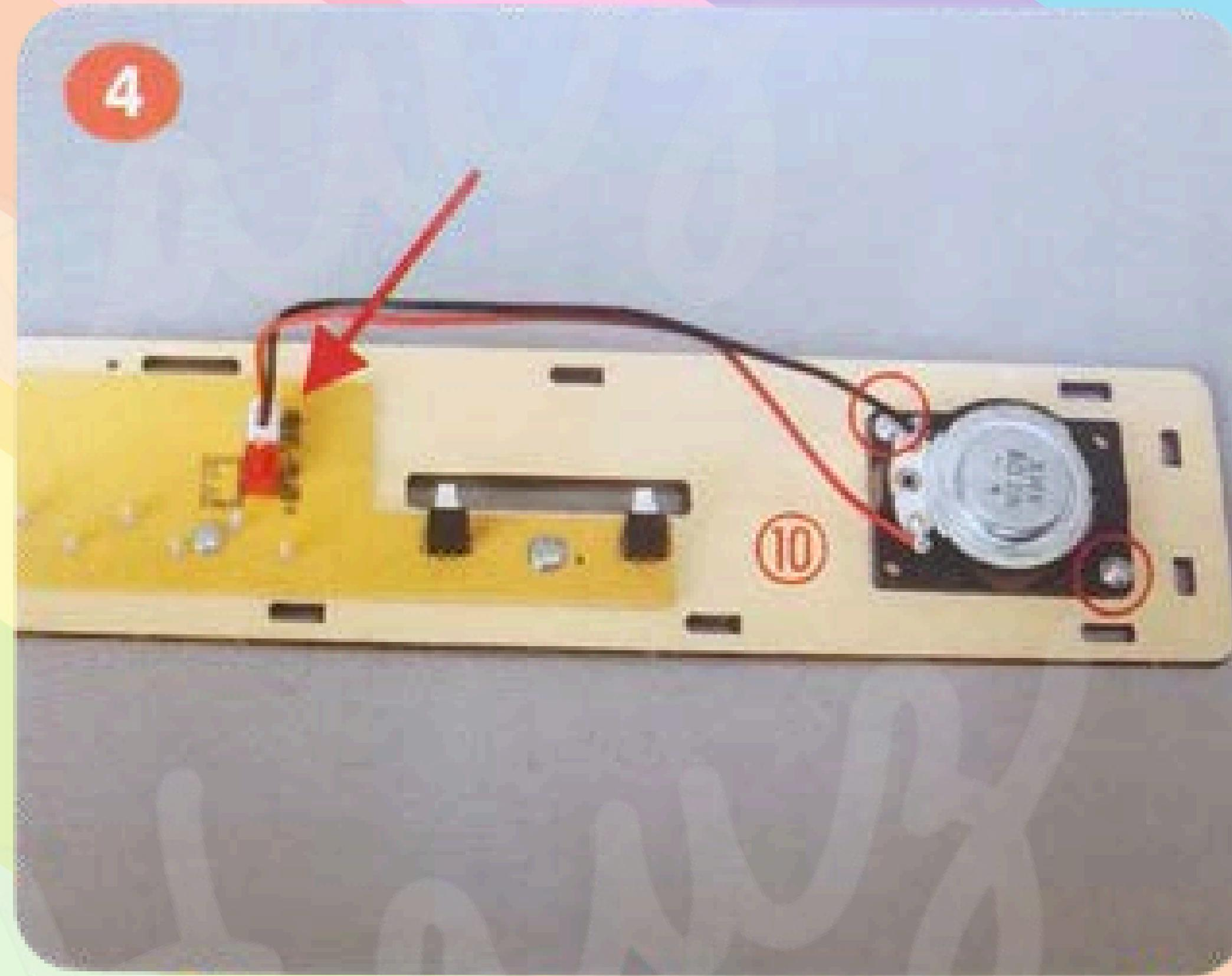
Use two 6 mm screws to fix the speaker onto board No. 10 (as shown in the picture).
