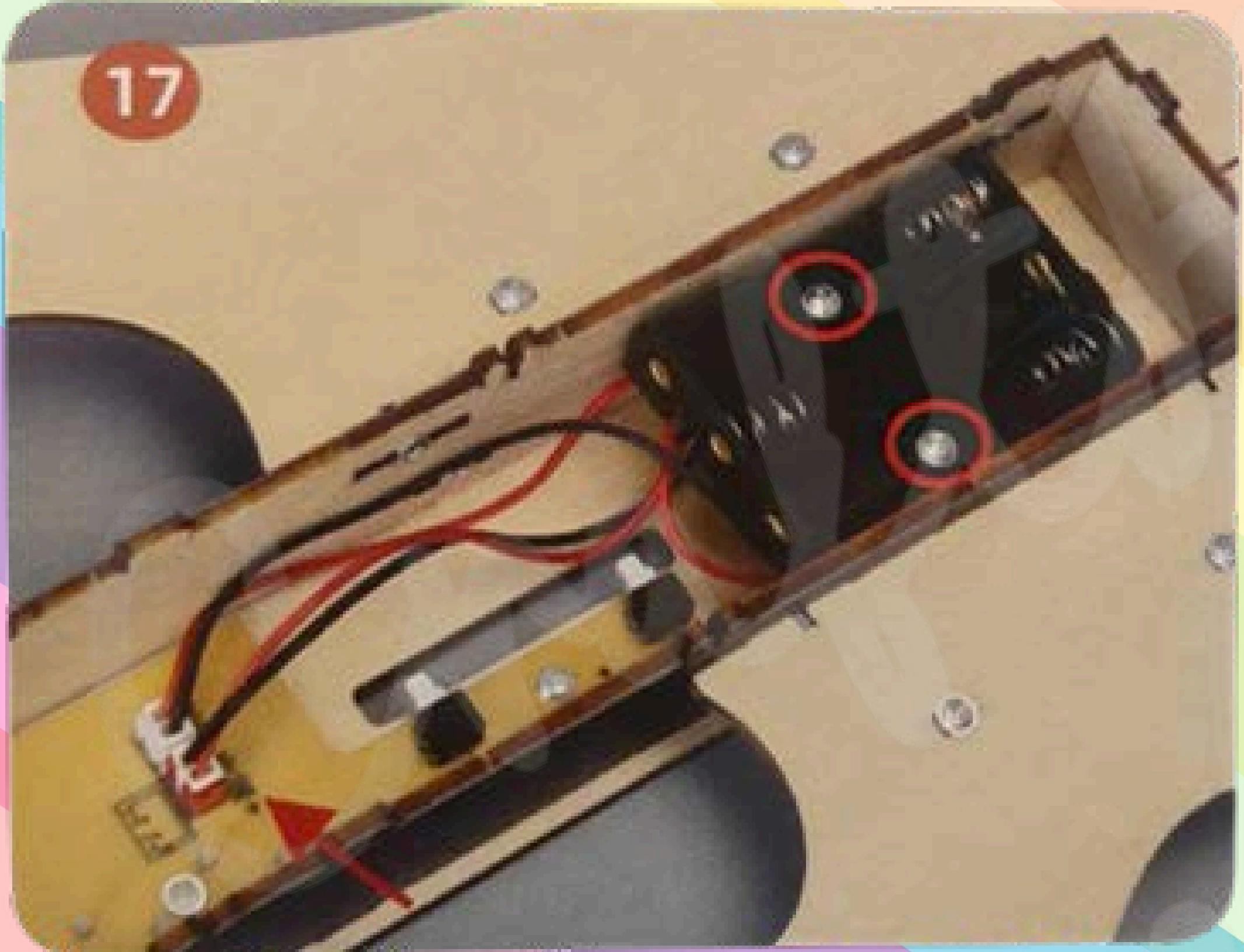
As shown in the picture, use two 4 mm screws to secure the battery box to board No. 12 by aligning the holes. Insert the connector into the power port.
