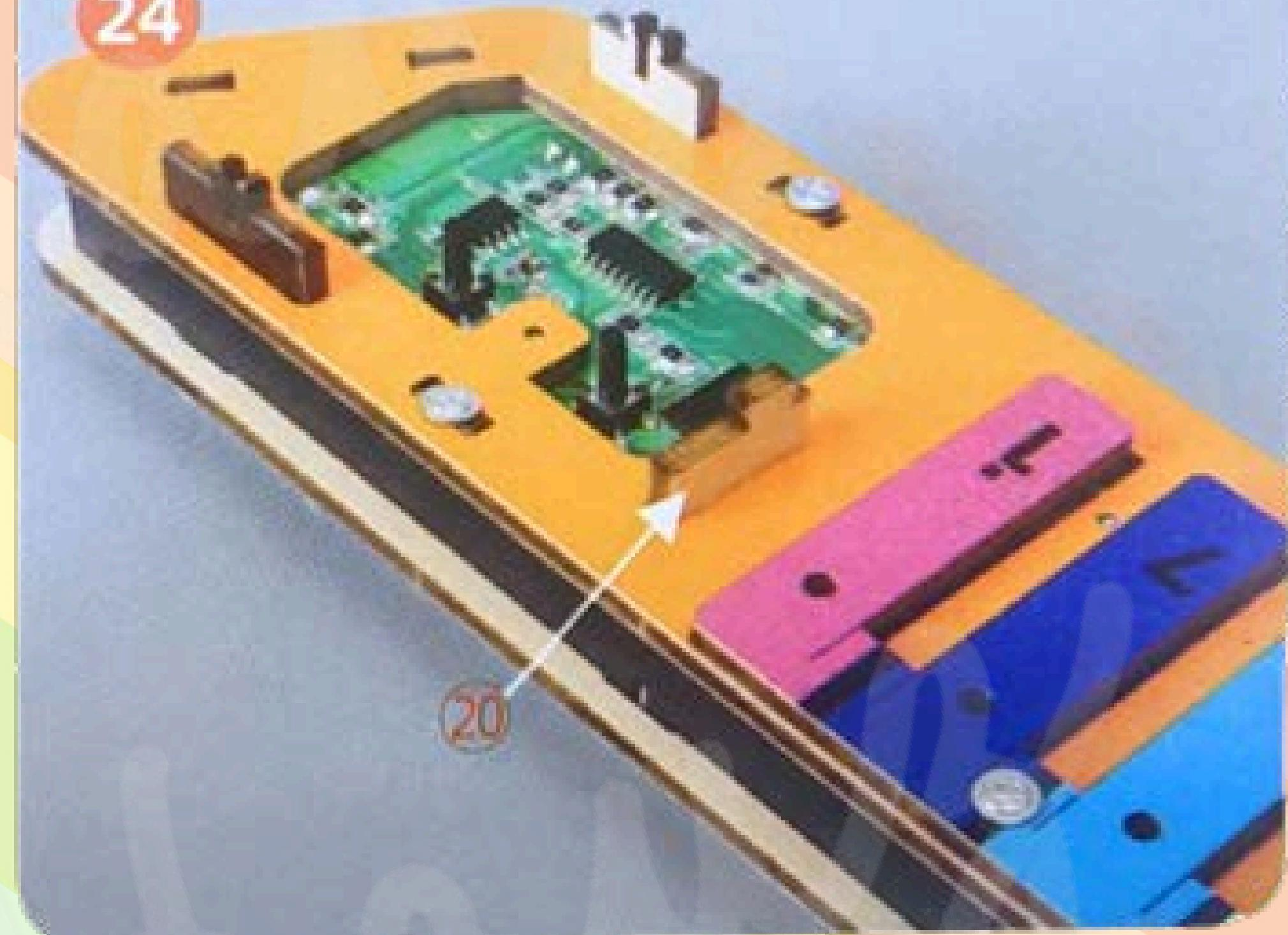
As shown in the picture, insert board No. 20 into place.
