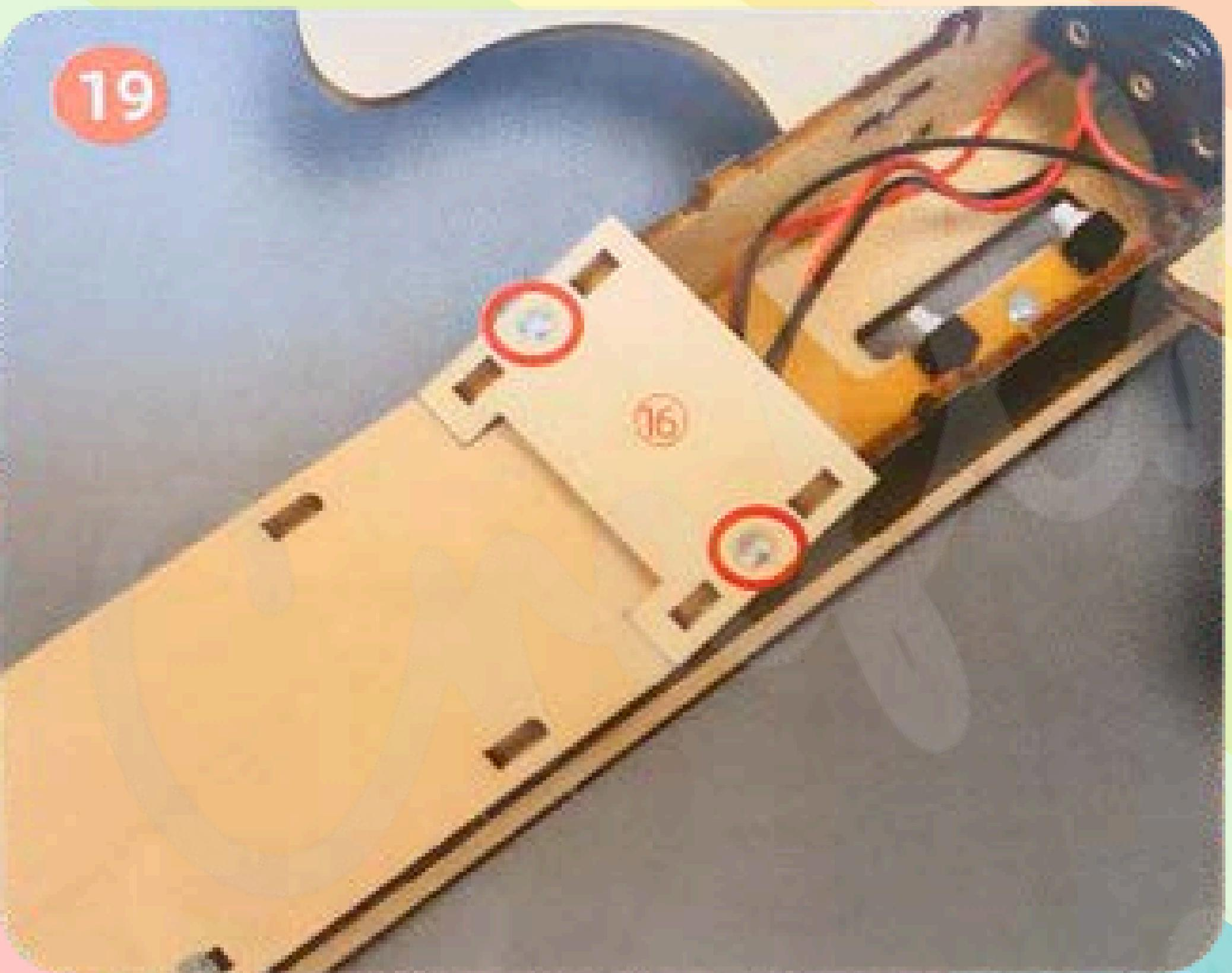
As shown in the picture, install board No. 16 and secure it with two 6 mm screws.
