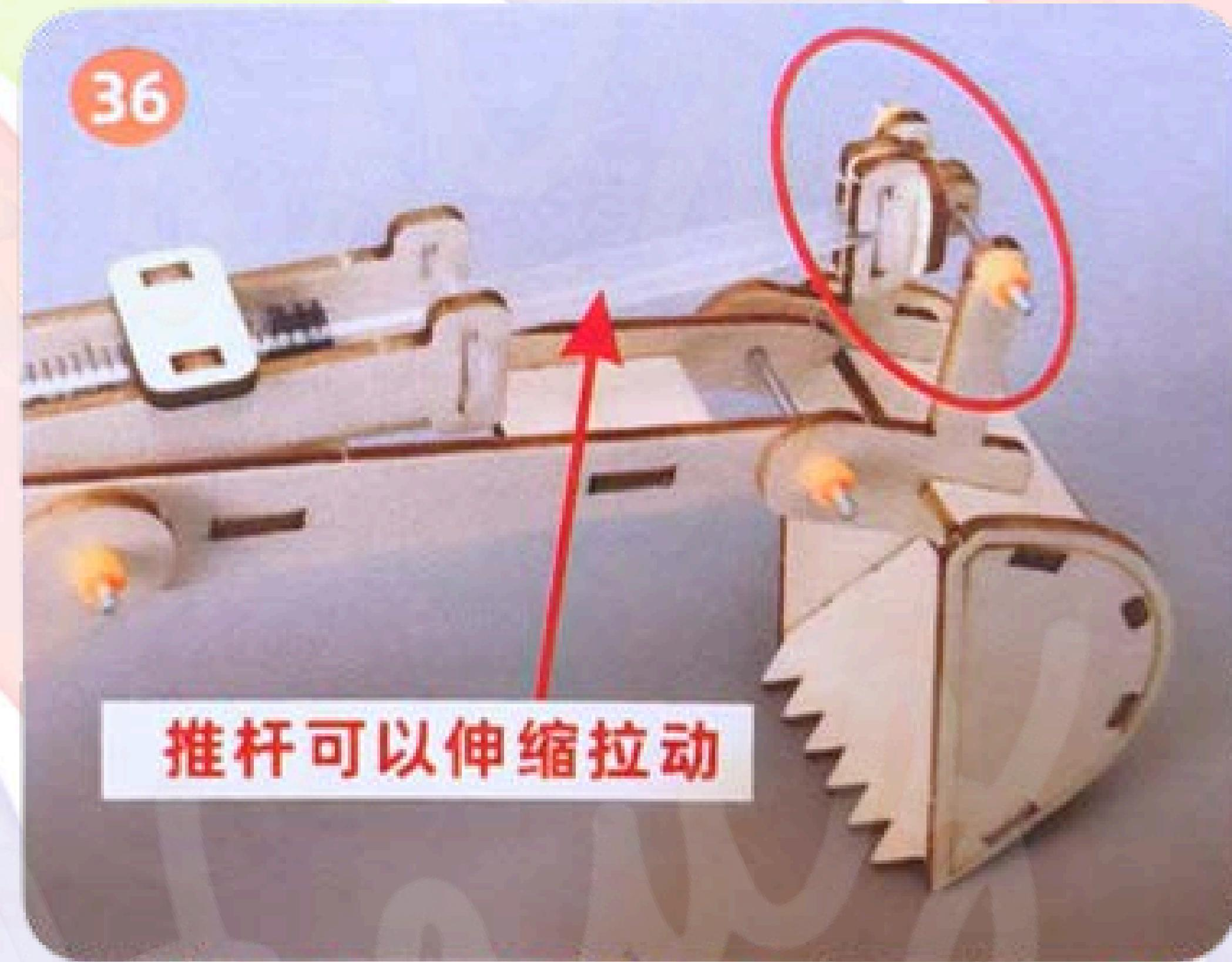
As shown in the picture, insert the 35 mm rod through the small syringe assembly and Support Frame No. 2 (second hole). Secure both sides with rubber sleeves. Prepare one 40 mm rod and two rubber sleeves.
