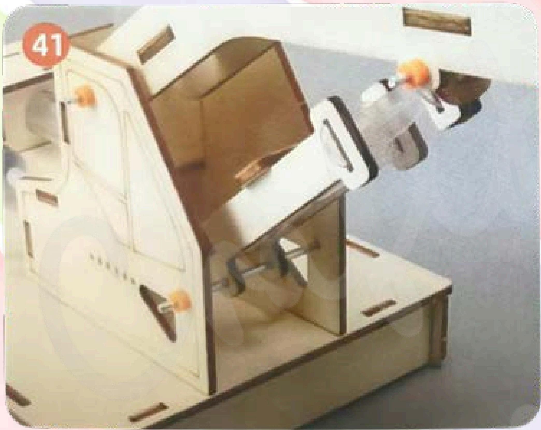
As shown in the picture, use a 55 mm rod to secure the small syringe assembly onto the base. Fix both sides with rubber sleeves.
