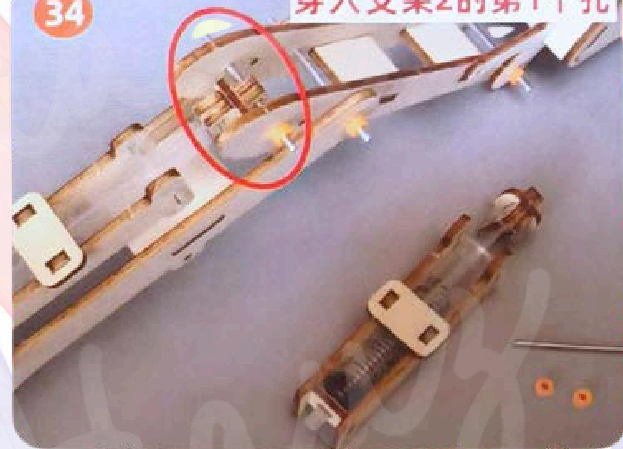
As shown in the picture, insert the 35 mm rod through Support Frame No. 2 and the small syringe assembly.
