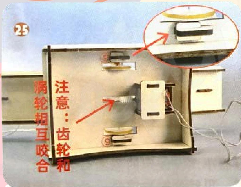
As shown in the picture, insert board No. 9 into the bottom of board No. 2 to prevent movement.
