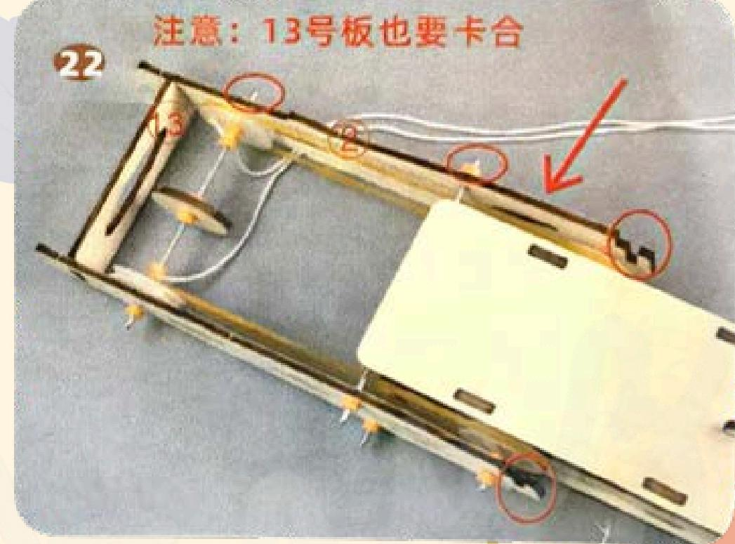
As shown in the picture, insert the other end of the rod into the corresponding hole on the second board No. 2, and secure it with rubber sleeve.
