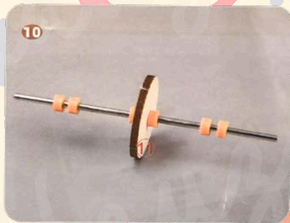
As shown in the picture, install board No. 11 and the rubber sleeves onto the metal rod.
