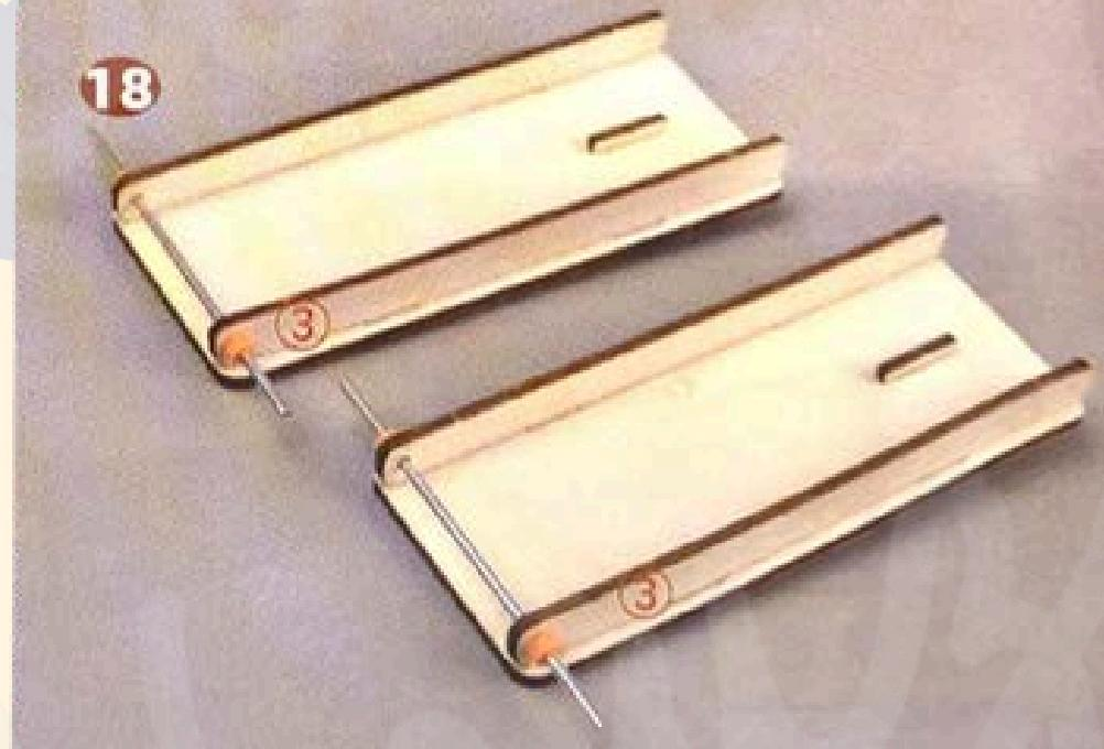
As shown in the picture, insert the rod into the round holes of board No. 3 and secure both sides with rubber sleeves.
