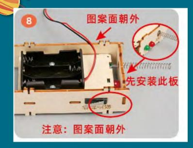
Install the ANT board first, then install the two side panels.
