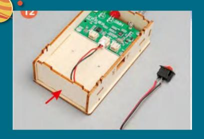
Install the wooden panel and prepare the switch.
