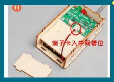
Insert the battery box terminals into the slot and prepare the wooden panels.
