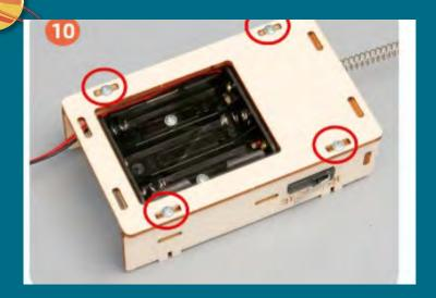
Install and fix with screws.
