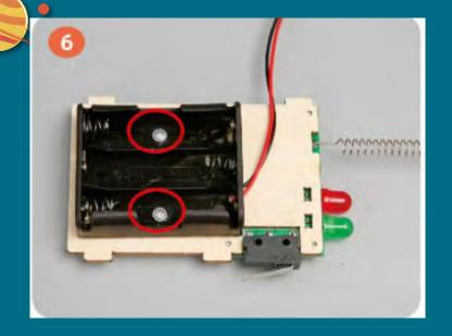
Use 4mm screws to fix the battery box.
