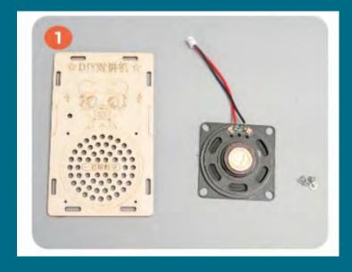
Prepare the components shown in the picture and four 4mm screws.
