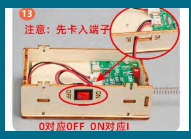
Insert the terminal first, then install the switch.
