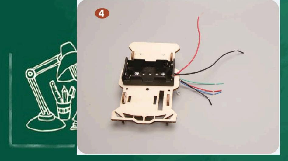
As shown, fix the battery box to the bottom of Step 3 using 4mm screws.
