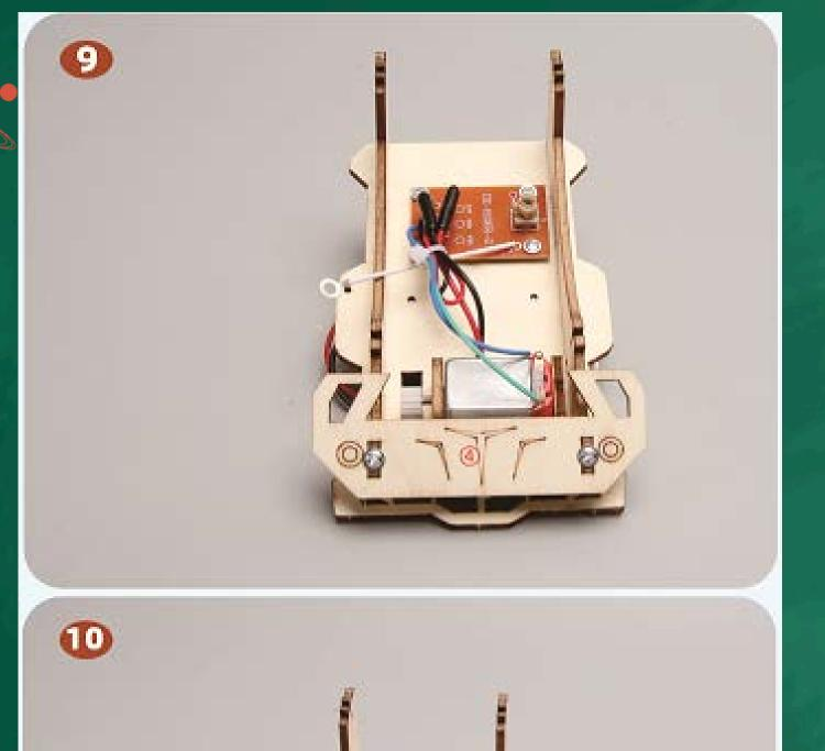
As shown, combine the No.4 board with Step 8 and fix with 7mm screws.
