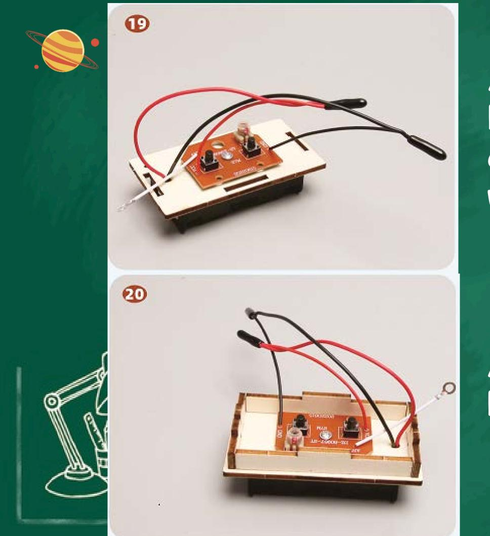
As shown, connect the battery box wires to remote control board B and insulate with heat-shrink tubing.
