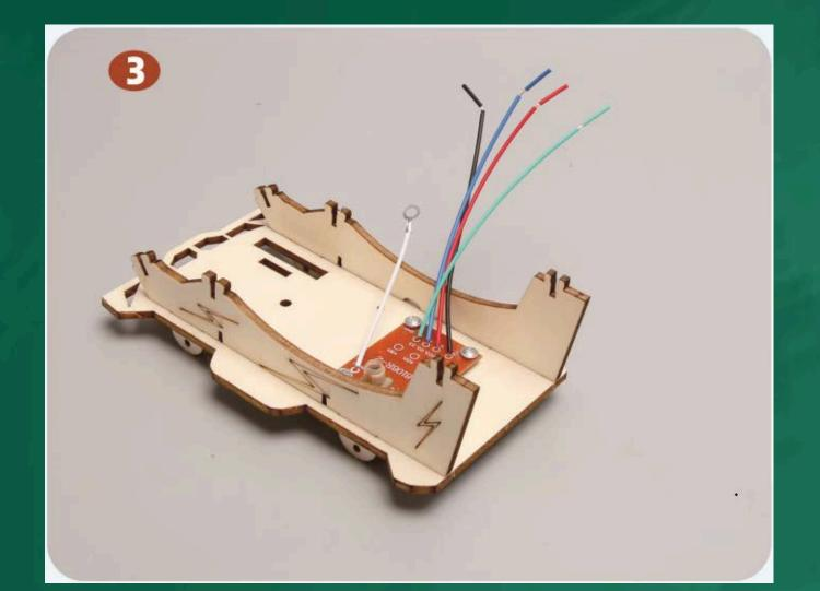
As shown, fix the remote control board A onto the No. 1 board with 7mm screws.
