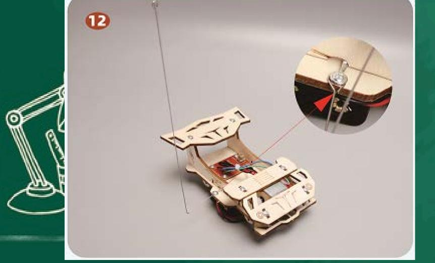
As shown, fix antenna 1 in the designated position on the No. 1 board.
