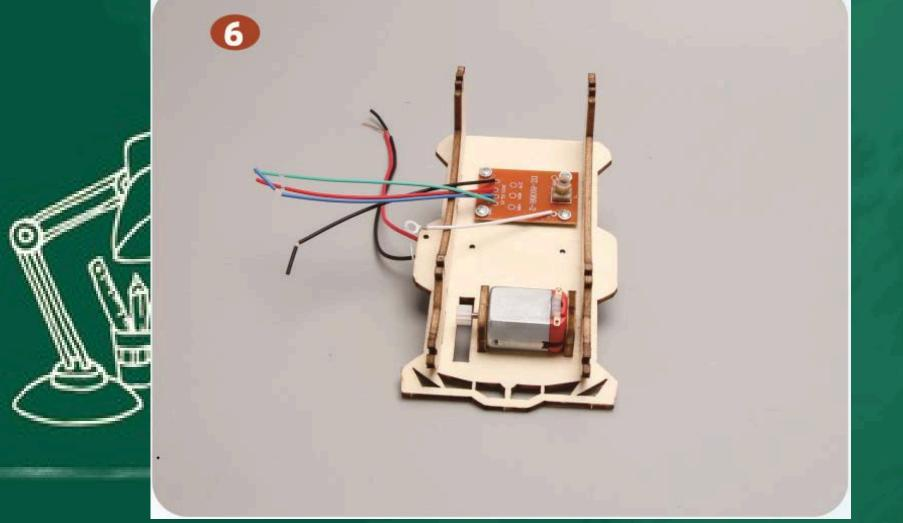
As shown, install the motor and fix it with 4mm screws.
