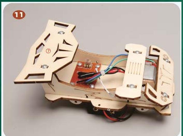
As shown, combine the No. 7 board with Step 10 and fix with 7mm screws.
