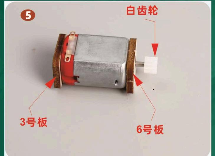
As shown, combine the No. 3 board, No. 6 board, and white gear with the motor (install the No. 6 board first, then the white gear).
