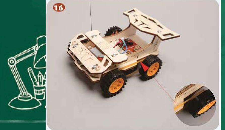
As shown, attach the rubber band to the belt wheel (car body completed).
