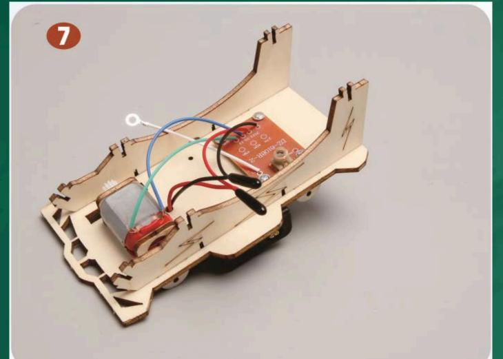
As shown, connect the wires and use heat-shrink tubing for insulation.
