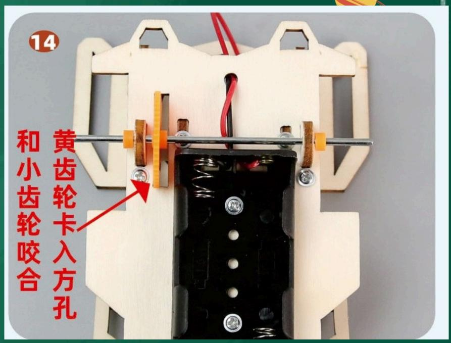
The yellow gear fits into the square hole and meshes with the small gear.
