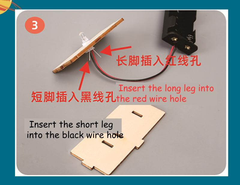
Insert the LED bulb into the terminal according to the markings.
