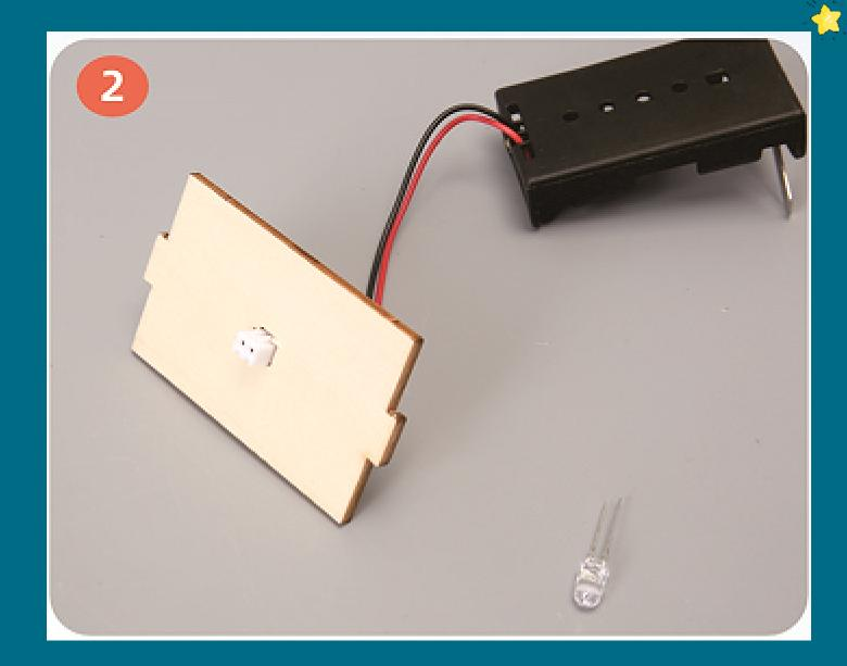
Insert the wire terminal through the hole as shown and prepare the LED bulb.
