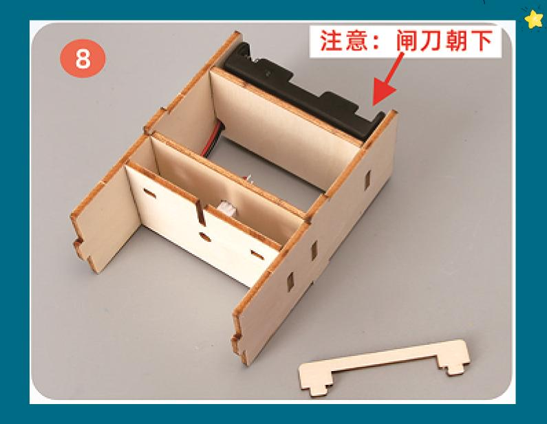
Use the foam adhesive to fix the battery box in place.
