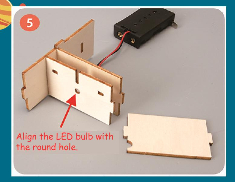
Align the round hole with the LED bulb as shown, then insert the side panel and prepare the parts for the next step.
