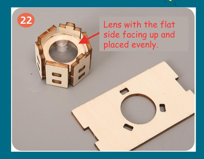
Insert the convex lens as shown.
