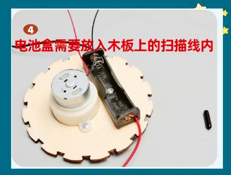
The battery box needs to be placed within the marked area on the wooden board.
