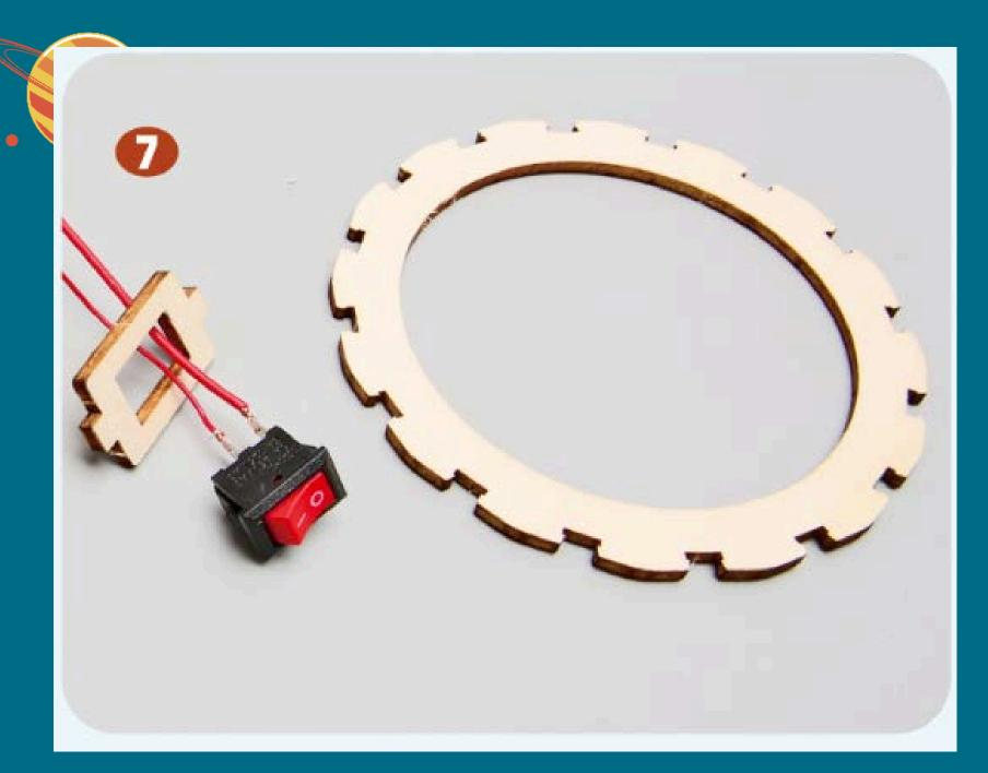
Connect the red wire to the switch and prepare the next set of parts.
