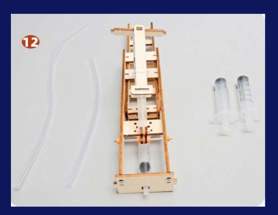
Prepare two soft tubes and two 5 ml syringes as shown.
