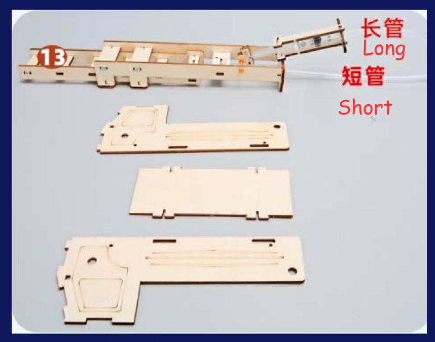
Connect the soft tubes and syringes, then prepare the wooden parts shown.
