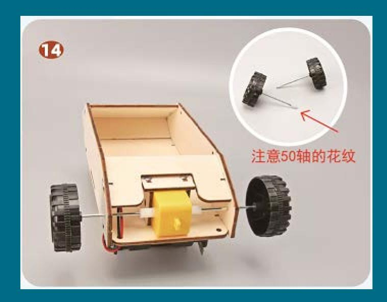
Then install the 50 mm shaft and large wheels on the motor bracket.
