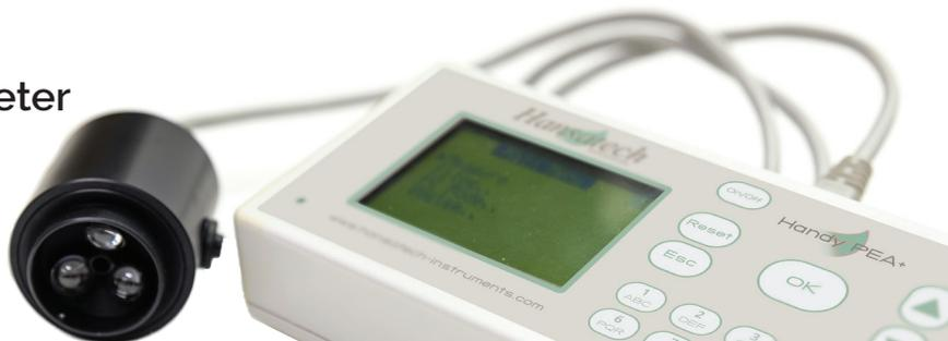
Simple to configure and operate, basic measurement functionality can be defined directly on the Handy PEA+. More complex experimental design may be achieved using the protocols feature which allows up to 5 user-defined protocols to be stored in memory for different field applications. Protocols are written using a custom Windows® software package, PEA+ (supplied). A tactile keypad allows selections and inputs to be made and a liquid crystal display module presents menu options and data.
