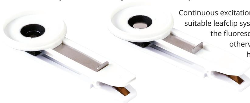
Continuous excitation fluorescence systems rely on the use of a suitable leafclip system with 2 functions. Firstly, the leafclip shields the fluorescence detector from ambient light which would otherwise "blind" the sensor due to the comparatively high levels of red/infra-red light within the same waveband as fluorescence itself. Secondly, the leafclip pre-conditions or dark adapts a section of the sample prior to the measurement.
