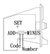
Code "H": Set up "15" Code "P": Output signal quantity: inset a coin usually, P1=01 for Lowest coin value, P+number=P1 multiply value rate Example: 2 dollar, 4 dollar: P1=01,P2=02 Code "F": Set up "08" Number: indicate rank of coin type
